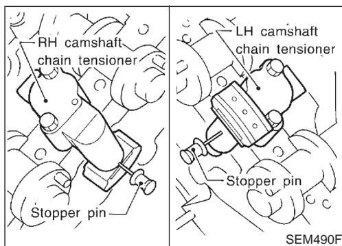
6. Install camshaft chain tensioners on both sides of cylinder head.
