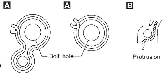
Sealant protrusion away from bolt hole
