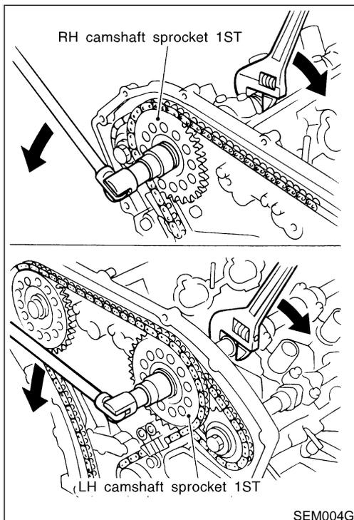
33. Remove RH & LH camshaft sprocket 1ST bolts.
