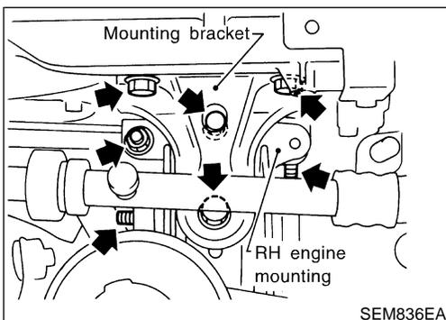
11. Remove RH engine mounting.
