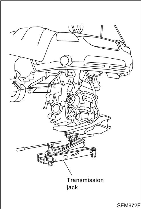
13. Remove engine with transaxle as shown.
