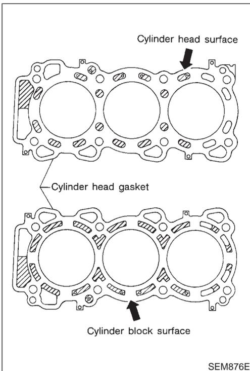
5. Install cylinder heads with new gaskets.
