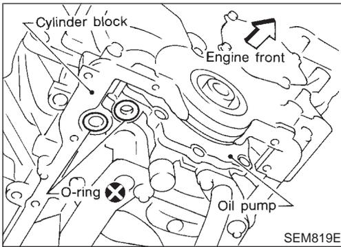
e. Install O-rings, cylinder block and oil pump body.
