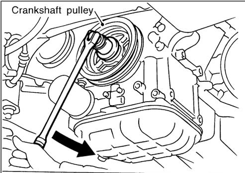
19. Loosen crankshaft pulley bolt. (At this time remove oil pan rear cover plate and set a suitable tool to ring gear so that crankshaft cannot rotate.)
