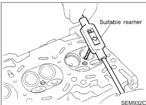
3. Ream cylinder head valve guide hole.
