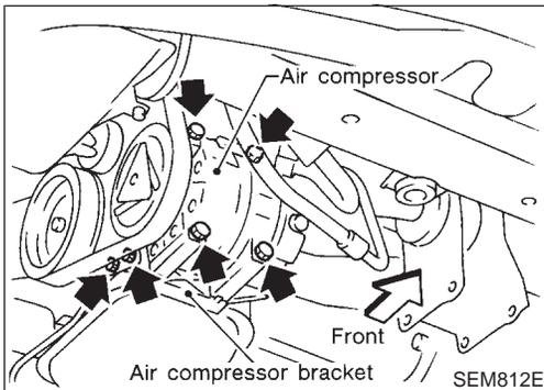
4. Install air compressor and bracket. Refer to HA-112, "Removal and Installation".
