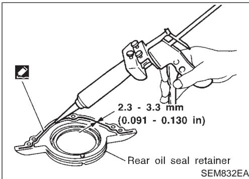
6. Apply liquid gasket to rear oil seal retainer.
