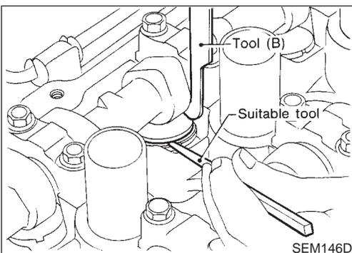
6. Blow air into the hole to separate adjusting shim from valve lifter.
