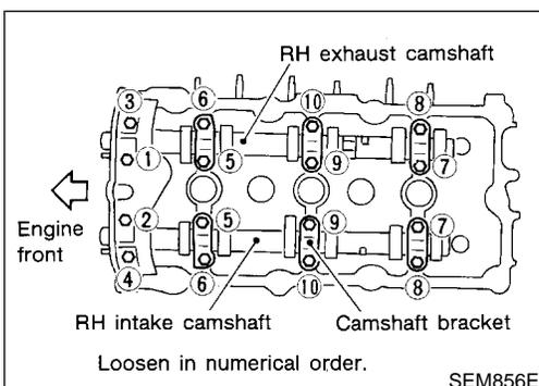
3. Remove intake and exhaust camshafts and camshaft brackets.
