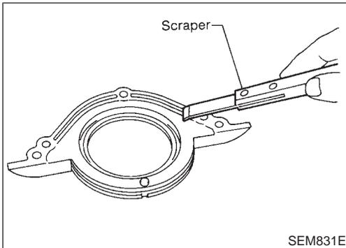
5. Remove old liquid gasket using scraper.
