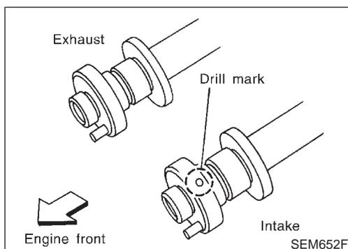
7. Install exhaust and intake camshafts and camshaft brackets.
