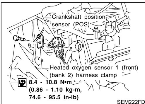
8. Install crankshaft position sensors (POS and REF) and heated oxygen sensor 1 (front) (bank 2) harness clamp.
