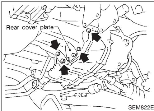
2. Install the four engine-to-transaxle bolts. For tightening torque, refer to AT-284, "Installation".
