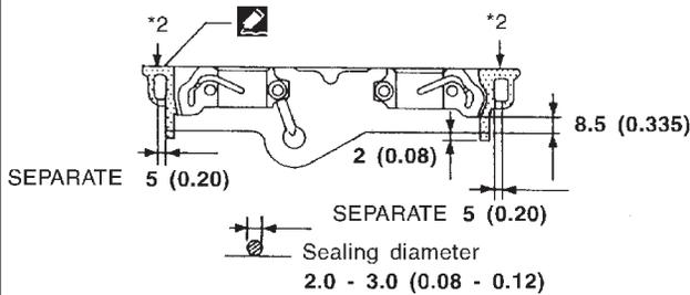
\*2 : Remove the protruding sealant from front face.
