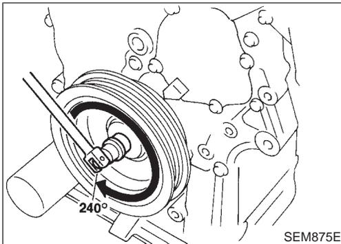
4. Turn crankshaft until No. 1 piston is set at approximately 240° before TDC on compression stroke to prevent interference of valves and pistons.
