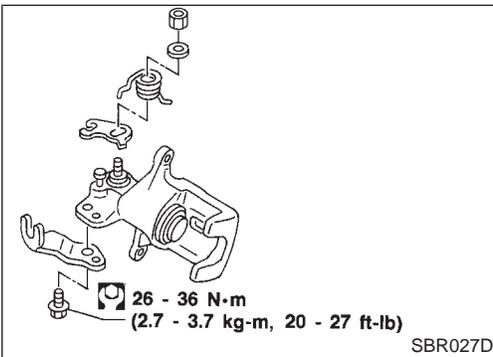
10. Fit toggle lever, return spring and cable guide.
