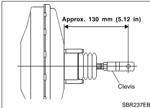
1. Before fitting booster, temporarily adjust clevis to dimension shown.
