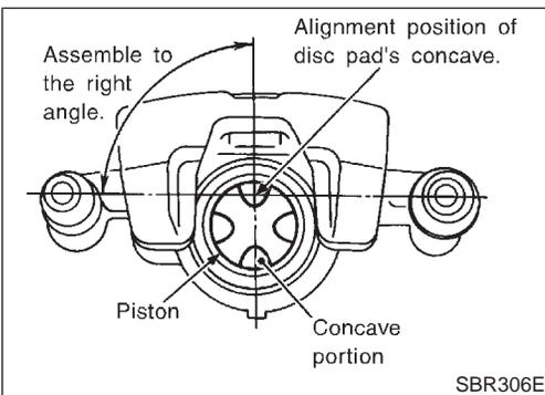
11. Adjust the piston to the right angle as shown in the figure.
