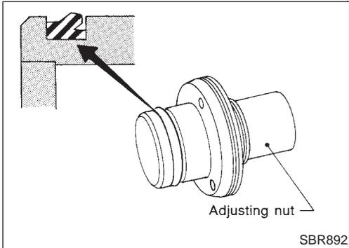
7. Install cup, adjuster, bearing, spacers, washers and ring A with a suitable tool.
