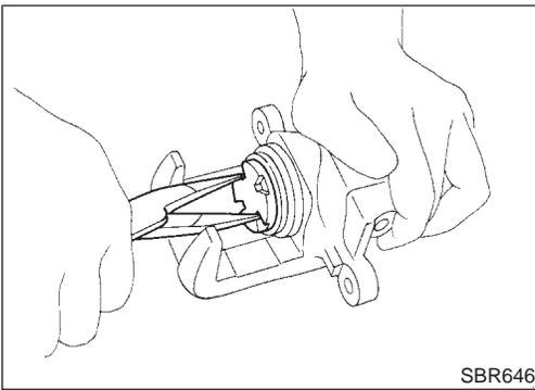
8. Insert piston seal into groove on cylinder body.
