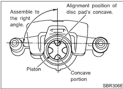
7. Adjust the piston to the right angle as shown in the figure.
