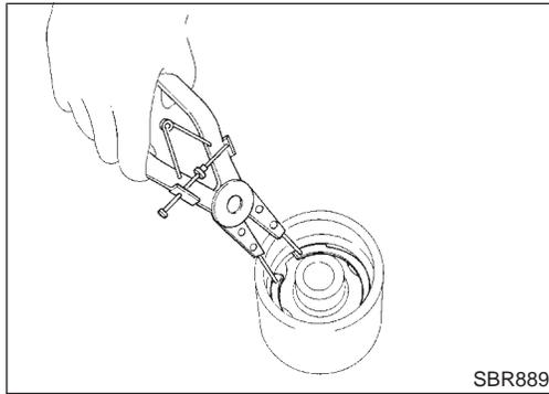
3. Disassemble cylinder body.
