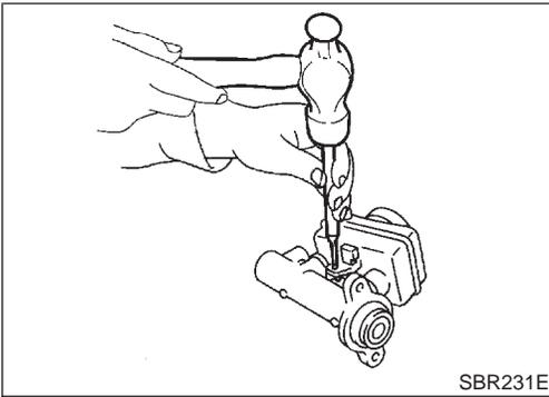
2. Drive out spring pin from cylinder body.
