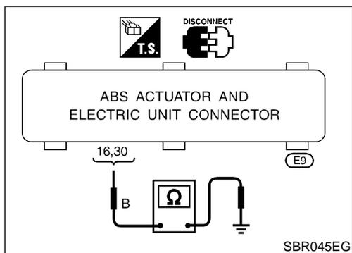
**Ground Circuit Check****ABS ACTUATOR AND ELECTRIC UNIT GROUND**
