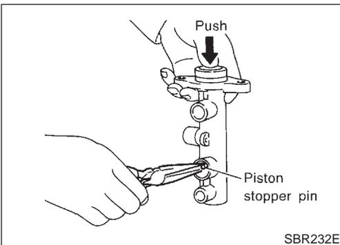
2. Install piston stopper pin while piston is pushed into cylinder.
