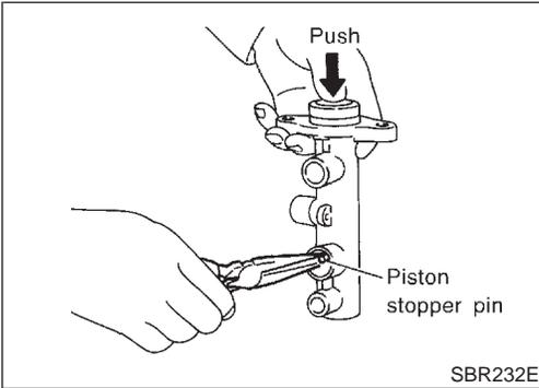
4. Remove piston stopper pin while piston is pushed into cylinder.
