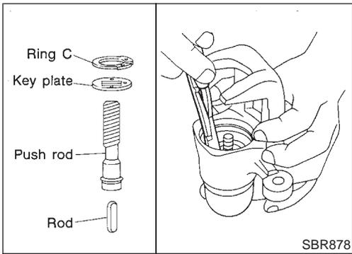
4. Install ring C with a suitable tool.
