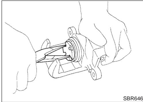
2. Pry off ring A from piston with suitable pliers and remove adjusting nut.
