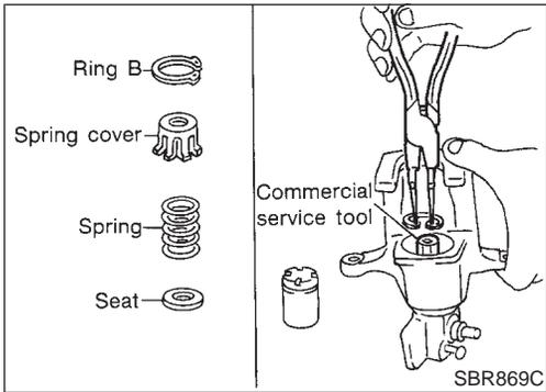
5. Install seat, spring, spring cover and ring B with suitable press and drift.
