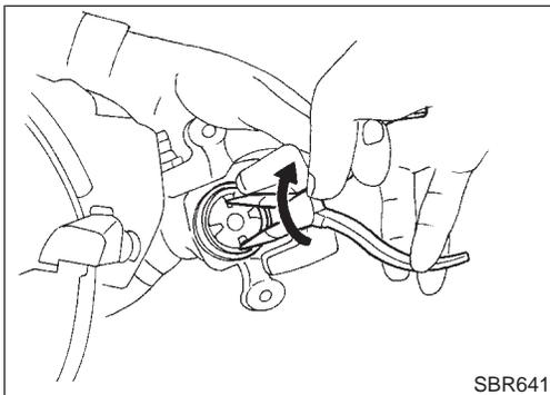
6. When installing new pads, push piston into cylinder body by gently turning piston clockwise, as shown. **Carefully monitor brake fluid level because brake fluid will return to reservoir when pushing back piston.**
