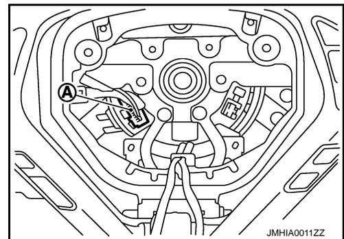
3. Remove the steering wheel. Refer to [ST-17. "Removal and Installation"](#).
