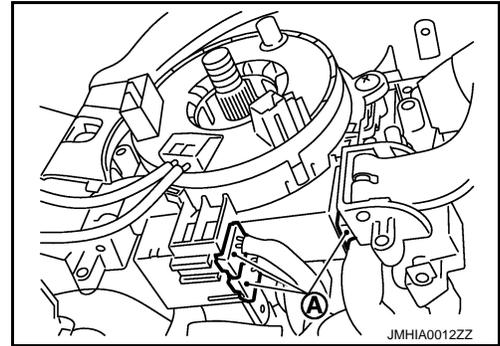
8. Remove the steering angle sensor. Refer to [BRC-117. "Removal and Installation"](#).
