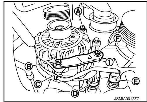
12. Remove alternator assembly downward from the vehicle.
