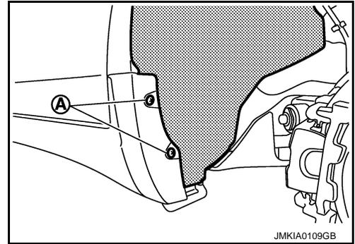
3. Remove rear wheel house protector mounting nuts and then remove rear wheel house protector.
