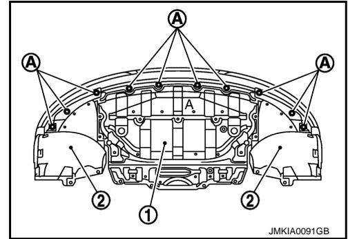
7. Remove fender protector (front) mounting bolts and clips, and then remove screws (A) of fixing bumper fascia left and right side.
