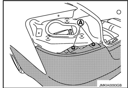
4. Remove screw (A) of bumper fascia underside.
