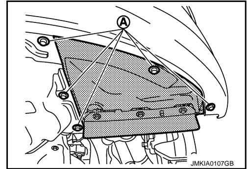
6. Remove fender protector (front) mounting clips.
