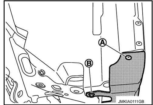
3. Remove screws (A) of center mud guard rear end.
