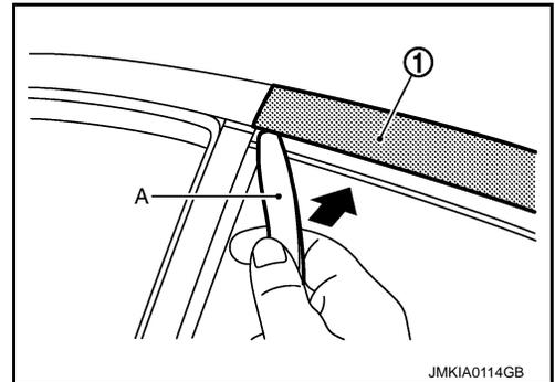
5. Release rear door sash molding connection between rear door panel and molding (1), using a remover tool (A), and take off double-faced adhesive tape.
