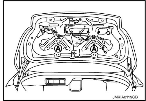
7. Apply protection tape (A) around outer circumference of trunk lid finisher outer (1).
