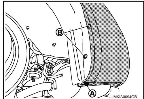
6. Remove screws (A) of bumper fascia front end upper (LH/RH).
