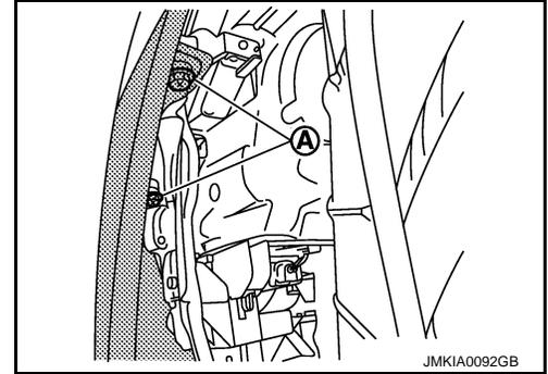
8. Pull bumper fascia assembly side toward the vehicle side, and then disengage bumper fascia assembly from bumper side brackets (LH/RH).
