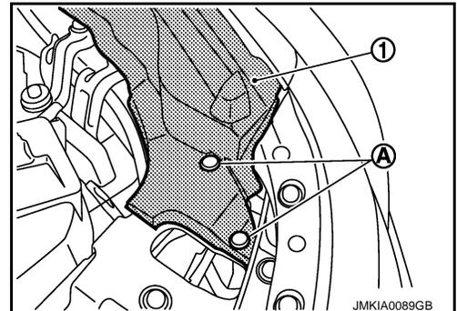
5. Remove bolts (A) of fixing bumper fascia and front fender (LH/RH), using a tool (B).
