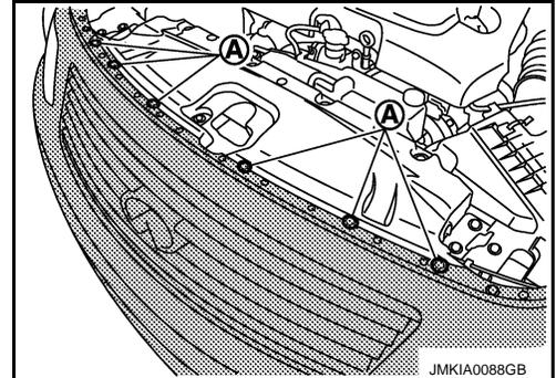
3. Remove radiator core support ornament. Refer to [DLK-203. "Removal and Installation"](#).
