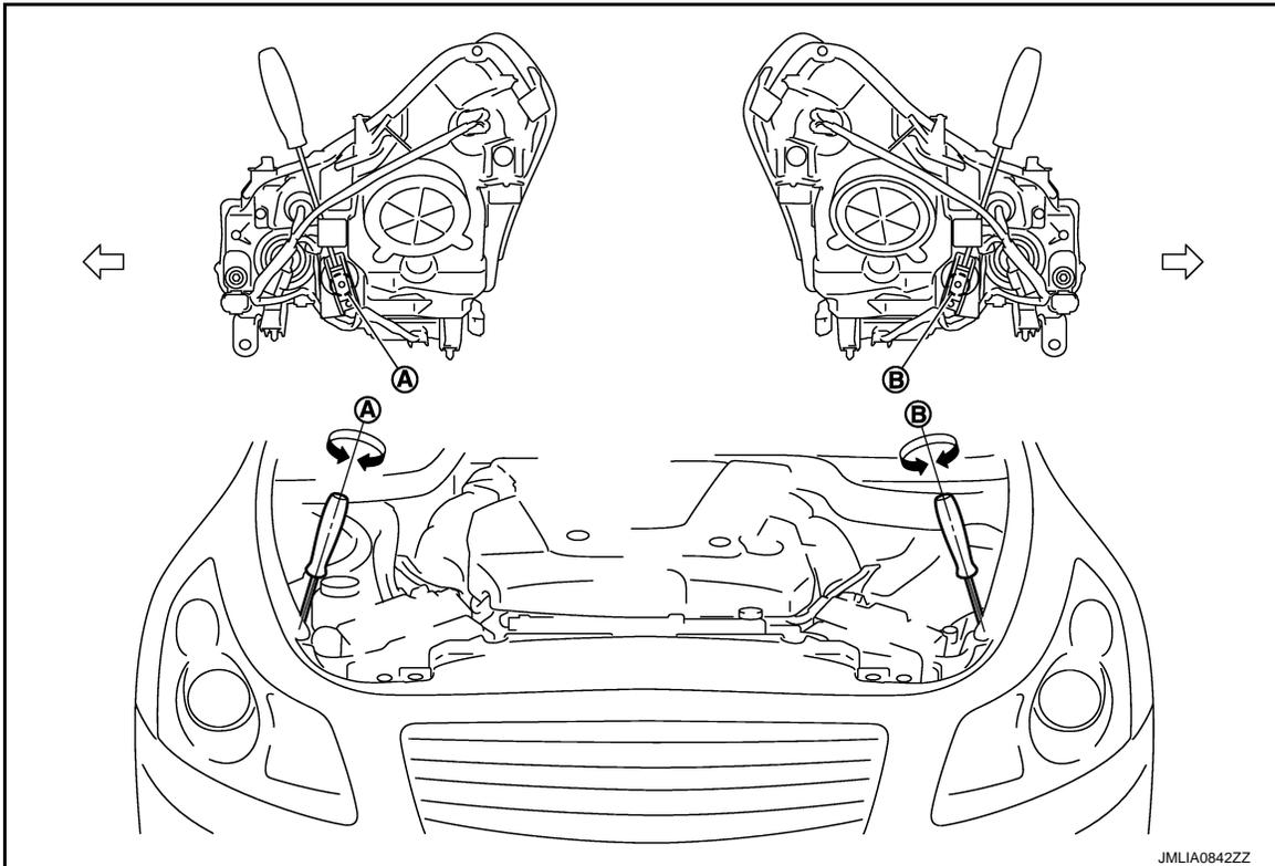
A Headlamp (RH) adjustment screw    B. Headlamp (LH) adjustment screw
