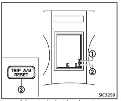
Odometer/twin trip odometer
