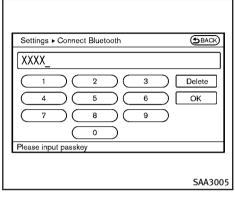
4. Choose a PIN code to use with the compatible Bluetooth® audio device using the number input screen. The PIN code will need to be entered into the Bluetooth® audio device after step 5. Select the "OK" key.
