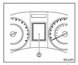
The dot matrix liquid crystal display (1) is located between the tachometer and the speedometer, and it displays the automatic transmission position indicator (if so equipped), the Intelligent Cruise Control (ICC) system (if so equipped) information, the Intelligent Key operation information and other warnings and information.
