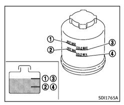
Check the fluid level in the reservoir.
