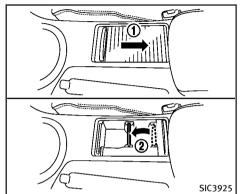
Manual transmission models — Front To open the cup holder, slide the lid ①. Install the partition plate into the slit ②.
