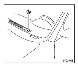
The sunload sensor (A) on the instrument panel helps maintain a constant temperature. Do not put anything on or around this sensor.
