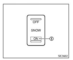
For driving or starting the vehicle on snowy roads or slippery areas, turn on the SNOW mode switch. The indicator light ① on the switch will illuminate. When the SNOW mode is activated, engine output is controlled to avoid wheel spin.
