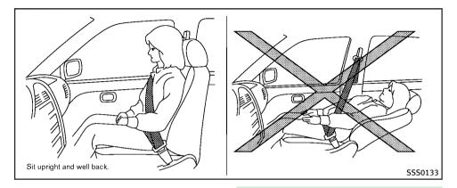
senger sits well back and straight up in the seat. If the seatback is reclined, the risk of sliding under the lap belt and being injured is increased.
