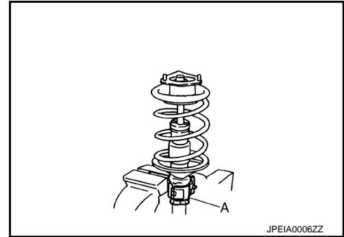
2. Using a spring compressor (A) (commercial service tool), compress coil spring between rubber seat and shock absorber until coil spring with a spring compressor is free.
