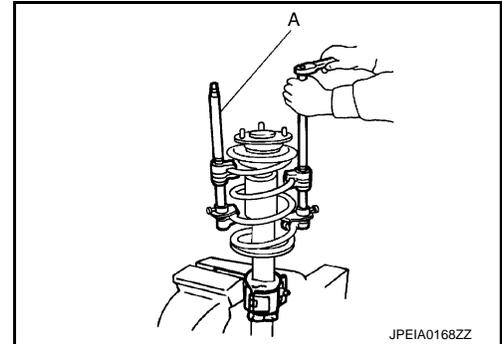
5. After removing coil spring with a spring compressor, then gradually release a spring compressor.
