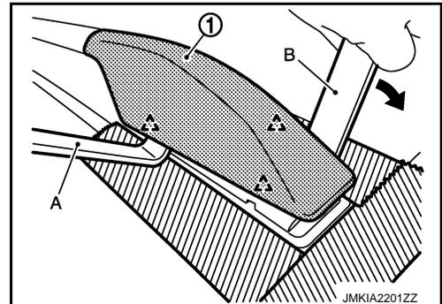
10. Pull rear roof rail cover (1) toward the direction of the arrow.
