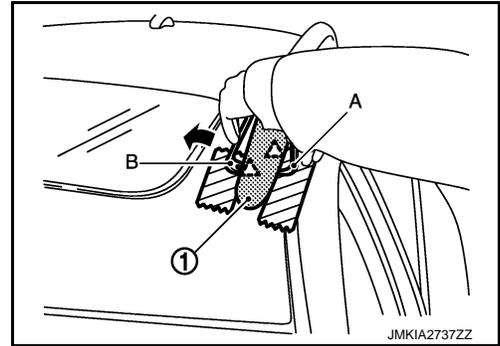
5. Pull front roof rail cover (1) toward the arrow direction.
