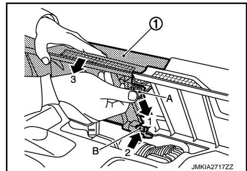
10. Push pawl (A) as shown by the arrow in the figure to remove cowl top cover LH (1).
