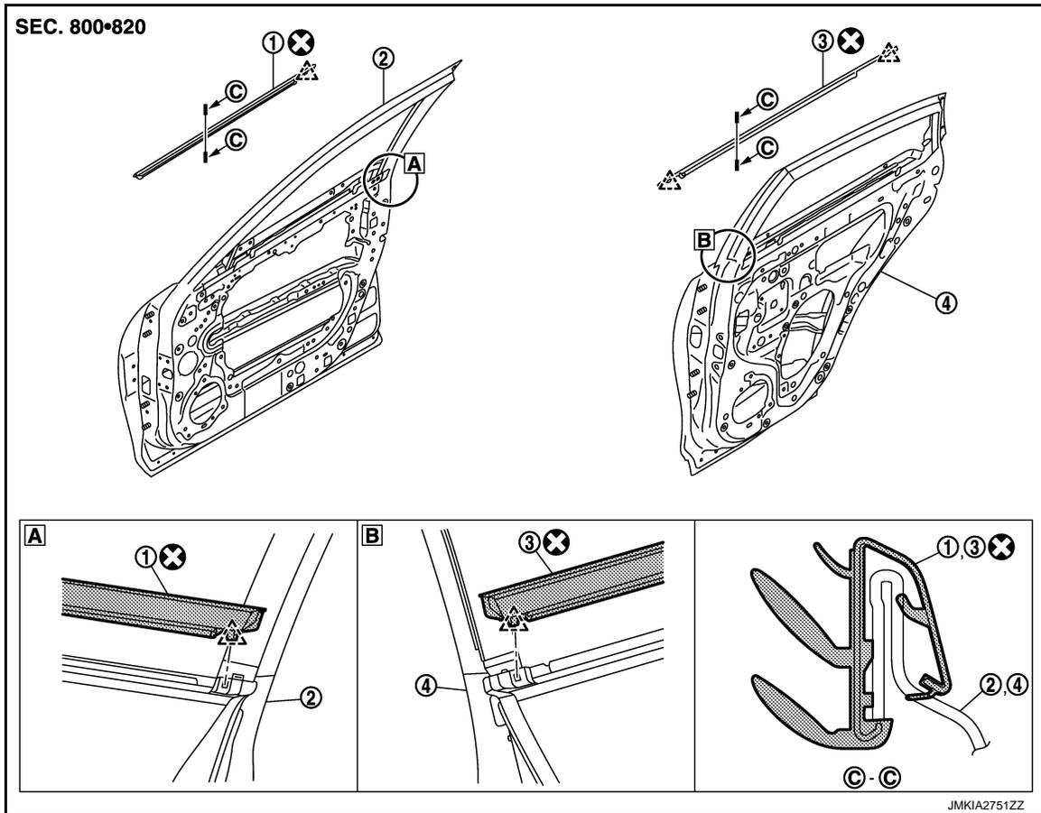
1. Front door outside molding      2. Front door panel      3. Rear door outside molding
