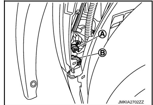
10. Remove bumper fascia assembly fixing screws (A) (LH/RH).
