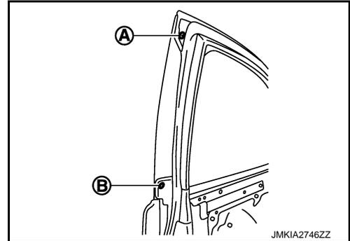
3. Release front door sash outer cover connection between front door panel and cover (1), with a remover tool (A) and cutter knife (B), and take off double-faced adhesive tape.
