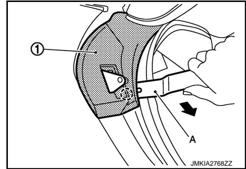
4. Remove back pillar finisher (1) fixing double-faced adhesive tape (A) and clip with a remover tool (B).
