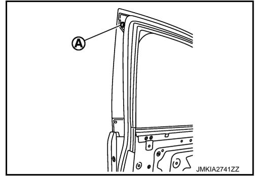
4. Release front door weather-strip and glass run rubber.
