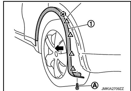
6. Remove bumper fascia assembly fixing screws (A) (LH/RH).
