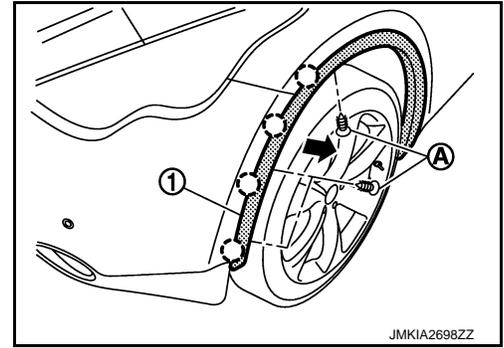
8. Remove front fender grommets (A) with a remover tool (B).
