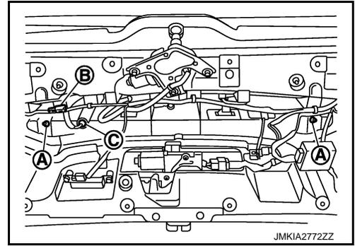
6. Remove back door finisher upper (1) fixing clips with remover tool (A).
