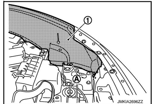
5. Remove bolts (A) of fixing bumper side stiffener (1) and front fender (LH/RH).
