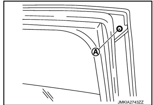
2. Remove rear door sash molding mounting screw (A) from rear end.
