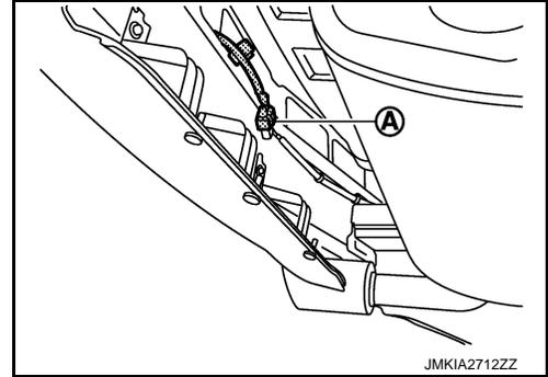
9. Pull both sides bumper fascia assembly toward the vehicle outside to disengage the bumper fascia assembly from bumper side brackets (LH/RH).
