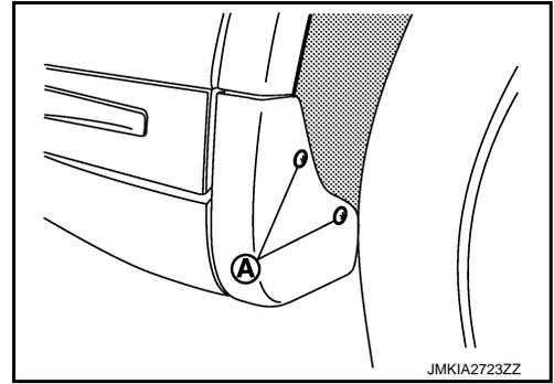
3. Remove rear wheel house protector fixing clips and grommets and then remove rear wheel house protector.
