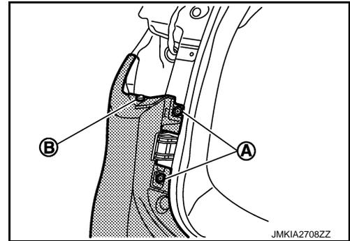
4. Remove rear fillet moldings (1) fixing screws (A) (LH/RH).
