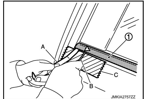
6. Twist and pull up to upper side, and then remove rear door outside molding (1).
