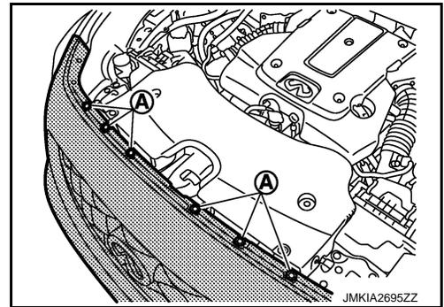
3. Remove engine room covers (LH/RH) (For VK engine models). Refer to [EM-174. "Exploded View"](#).
