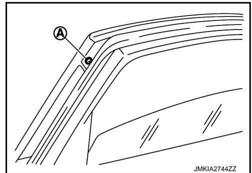
3. Release rear door weather-strip and glass run rubber.
