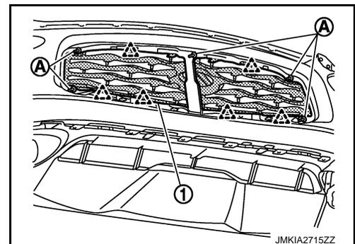
4. Remove the following parts after removing front grille.
