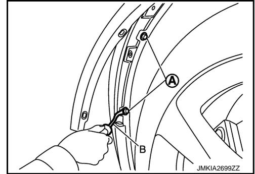
9. Disconnect harness connectors (A) and (B) from back side of bumper fascia assembly (LH).
