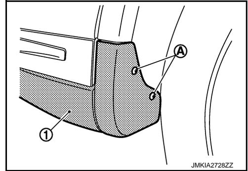
4. Remove bolts of center mud guard underside.
