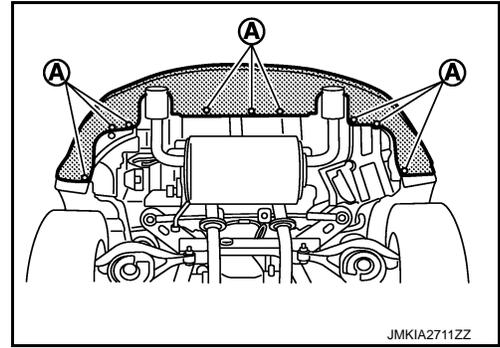
8. Disconnect bumper sub harness connector (A).
