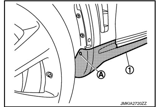
5. Remove fender protector (rear) fixing clips.
