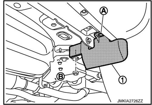
2. Remove screw (A) of center mud guard (1) front end.
