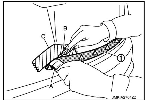
2. Pull and remove back door finisher lower.
