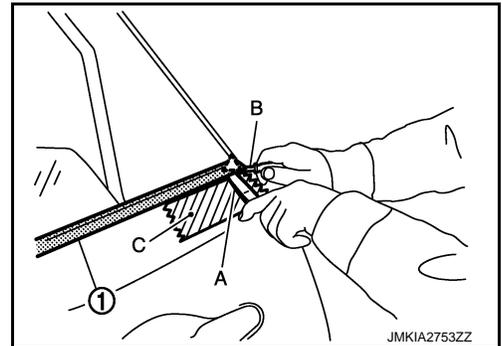
4. Insert a remover tool (A) into lower space.
