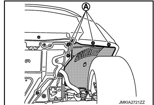
8. Remove fender protector (front) mounting clips.
