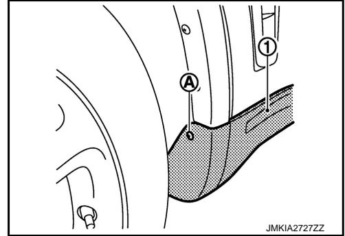
3. Remove screws (A) of center mud guard (1) rear end.
