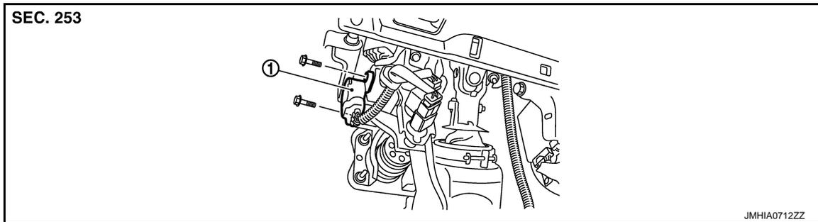
1. Brake pedal stroke sensor
