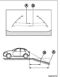
m) distance on the hill is the place (B). Note that any object on the hill is closer than it appears on the monitor.
