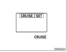
When the ignition switch is pushed to the ON position, the indicators come on as illustrated to check for a burned-out bulb, and it turns off when the engine is started.
