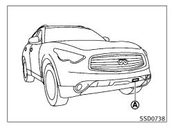
The IBA system uses a distance sensor (A) located below the front bumper to measure the distance to the vehicle ahead. When the system judges that your vehicle is getting close to the vehicle ahead in the traveling lane, the vehicle ahead detection indicator light on the instrument panel blinks and a warning chime sounds.
