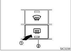
To defog/defrost the rear window glass and outside mirrors, start the engine and push the switch (1) on. The indicator light (2) will come on. Push the switch again to turn the defroster off.
