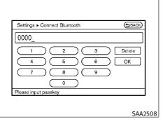
4. Choose a PIN code to use with the compatible Bluetooth audio device using the number input screen. The PIN code will need to be entered into the Bluetooth audio device after step 5. Select the "OK" key.
