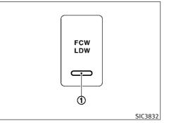
The Lane Departure Warning (LDW) system will sound a warning chime and blink the lane departure warning light (orange) to alert the driver if the vehicle is traveling close to either the left or the right of a traveling lane with detectable lane markers.
