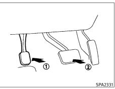
**To apply:** Fully depress the parking brake pedal ①.
