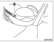
The sunload sensor  $(\mbox{A})$  on the instrument panel helps maintain a constant temperature. Do not put anything on or around this sensor.
