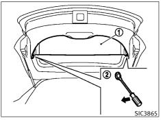
The rear cargo cover (1) can be removed from the lift gate.
