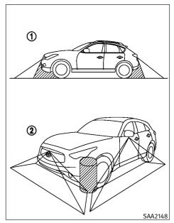
There are some areas where the system will not detect objects. When in the front or the rearview display, an object below the bumper or on the ground may not be detected (1). When in the bird-eye view, a tall object near the seam of the camera detecting areas will not appear in the monitor (2).
