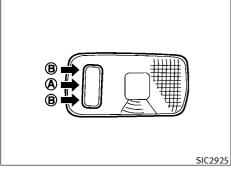
When the switch is in the DOOR position  $(\mathbb{A})$ , the light illuminates while the lift gate is opened. When the lift gate is closed, the light will turn off.
