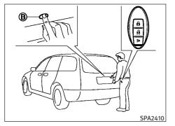
When you carry the Intelligent Key with you, you can lock or unlock all doors by pushing the door handle request switch (driver's or front passenger's) (A) or the lift gate request switch (B) within the range of operation.
