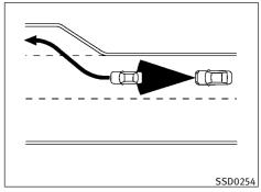
When driving on the freeway at a set speed and approaching a slower traveling vehicle ahead, the ICC will adjust the speed to maintain the distance, selected by the driver, from the vehicle ahead. If the vehicle ahead changes lanes or exits the freeway, the ICC system will accelerate and maintain the speed up to the set speed. Pay attention to the driving operation to maintain control of the vehicle as it accelerates to the set speed.
