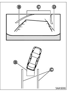
Slowly back up the vehicle adjusting the steering wheel so that the predicted course lines (B) enter the parking space (C).
