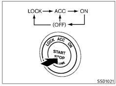
When the ignition switch is pushed without depressing the brake pedal, the ignition switch position will change as follows:
