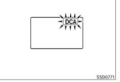
To set the DCA system to on or off, highlight the "Distance Control Assist" key, select ON or OFF and push the ENTER
