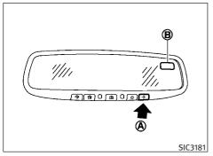
When the ignition switch is pushed to the ON position, the compass display (B) will indicate the direction of the vehicle's heading.
