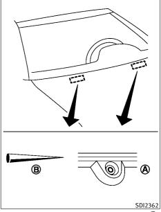
Be careful not to clog the washer nozzle  $(\mathbb{A})$ . This may cause improper windshield washer operation. If the nozzle is clogged, remove any objects with a needle or small pin  $(\mathbb{B})$ . Be careful not to damage the nozzle.
