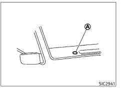
Be sure not to put anything on top of the photo sensor (A) located on the top of the instrument panel. The photo sensor controls the autolight; if it is covered, the photo sensor reacts as if it is dark and the headlights will illuminate.
