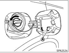
Put the fuel-filler cap on the cap holder A while refueling.
