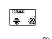
When passing another vehicle, the set speed indicator will flash when the vehicle speed exceeds the set speed. The vehicle detect indicator will turn off when the area ahead of the vehicle is open. When the pedal is released, the vehicle will return to the previously set speed.
