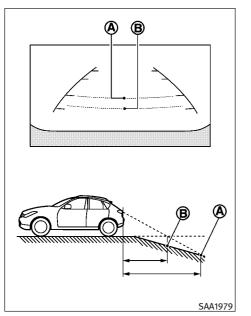
m) distance on the hill is the place (B). Note that any object on the hill is viewed in the monitor closer than it appears.
