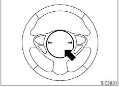
To sound the horn, push the center pad area of the steering wheel.
