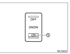
For driving or starting the vehicle on snowy roads or slippery areas, turn on the SNOW mode switch. The indicator light ① on the switch will illuminate. When the SNOW mode is activated, engine output is controlled to avoid wheel spin.
