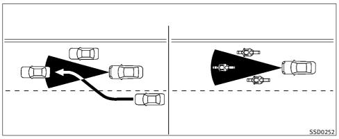
The detection zone of the sensor is limited. A vehicle ahead must be in the detection zone for the system to operate.
