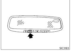
3. Using both hands, simultaneously push and hold both the HomeLink® button you want to program and the hand-held transmitter button.
