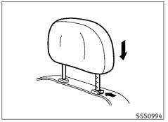
To lower, push and hold the lock knob and push the head restraint down.
