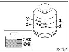
Check the fluid level in the reservoir.
