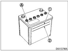
Check the fluid level in each cell (Remove the battery cover if it is necessary). It should be between the UPPER LEVEL (1) and LOWER LEVEL (2) lines.
