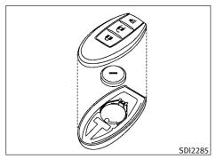
3. Replace the battery with a new one.
