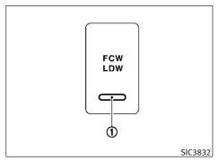
The Forward Collision Warning (FCW) system will sound a warning chime and blink the forward collision warning light (orange) to alert the driver if the vehicle is traveling close to a vehicle ahead.
