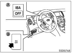
If the IBA OFF indicator light (A) illuminates with a beep sound, pull off the road to a safe location, stop the vehicle and turn the engine off. Check to see if the sensor window is dirty. If the sensor window is dirty, clean it with a soft cloth and restart the engine. If the sensor window is not dirty, restart the engine. If the IBA OFF indicator light continues to illuminate even if the IBA system is turned on with the IBA OFF switch (B), have the system checked by an INFINITI retailer.
