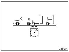
The GCWR equals the combined weight of the towing vehicle (including passengers and cargo) plus the total trailer load. Towing loads greater than these or using improper towing equipment could adversely affect vehicle handling, braking and performance.
