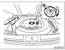
Remove jacking tools and the spare tire located under the luggage room.
