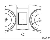
The dot matrix liquid crystal display (1) is located between the tachometer and the speedometer, and it displays the automatic transmission position indicator, the Intelligent Cruise Control (ICC) system (if so equipped), the Distance Control Assist (DCA) system (if so equipped) information, the Intelligent Key operation information and other warnings and information. For detailed information about each system, see the following sections:
