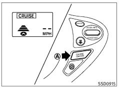
Operating vehicle-to-vehicle distance control mode
