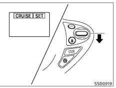
To set cruising speed, accelerate your vehicle to the desired speed, push the SET/COAST switch and release it. (The SET indicator will come on in the display.) Take your foot off the accelerator pedal. Your vehicle will maintain the set speed.
