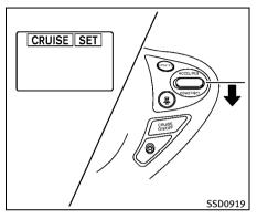
To set cruising speed, accelerate your vehicle to the desired speed, push the SET/COAST switch and release it. (The SET indicator will come on in the display.) Take your foot off the accelerator pedal. Your vehicle will maintain the set speed.
