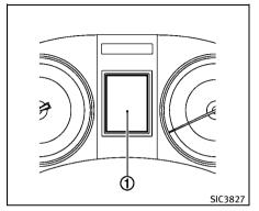
The dot matrix liquid crystal display (1) is located between the tachometer and the speedometer, and it displays the automatic transmission position indicator, the Intelligent Cruise Control (ICC) system (if so equipped), the Distance Control Assist (DCA) system (if so equipped) information the Intelligent Key operation information and other warnings and information.
