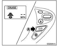
Operating vehicle-to-vehicle distance control mode
