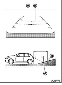
place **B**. Note that any object on the hill is further than it appears on the monitor.
