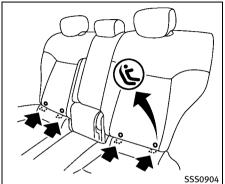
LATCH system lower anchor locations Lower Anchors and Tethers for CHildren (LATCH) System
