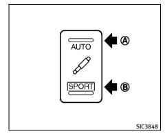
The Continuous Damping Control optimizes damping force and helps minimize the movement of the vehicle body. It helps stable driving when the vehicle moves up and down on large rolling roads or when the vehicle body leans during cornering with a high centrifugal force.
