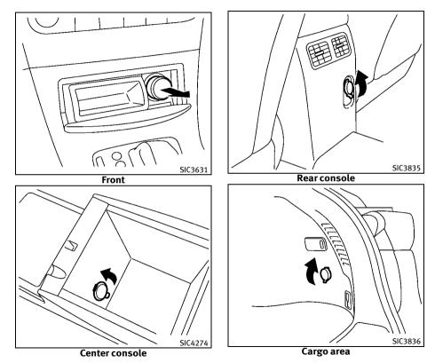
The power outlet is used for powering electrical accessories such as cellular telephones.
