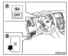
If the IBA OFF indicator light (A) illuminates with a beep sound, pull off the road to a safe location, stop the vehicle and turn the engine off. Check to see if the sensor window is dirty. If the sensor window is dirty, clean it with a soft cloth and restart the engine. If the sensor window is not dirty, restart the engine. If the IBA OFF indicator light continues to illuminate even if the IBA system is turned on with the IBA OFF switch (B), have the system checked by an INFINITI retailer.
