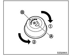
The climate controlled seat warms up or cools down the front seats by blowing warm or cool air from the surface of the seat. The switches located on the center console can be operated independently of each other.
