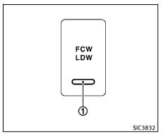
The Forward Collision Warning (FCW) system will sound a warning chime and blink the forward collision warning light (orange) to alert the driver if the vehicle is traveling close to a vehicle ahead.
