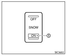
For driving or starting the vehicle on snowy roads or slippery areas, turn on the SNOW mode switch. The indicator light (1) on the switch will illuminate. When the SNOW mode is activated, engine output is controlled to avoid wheel spin.
