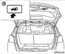
Power lift gate switch — Lift gate
