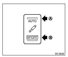
The Continuous Damping Control optimizes the damping force and helps minimize the movement of the vehicle body. It helps stable driving when the vehicle moves up and down on large rolling roads or when the vehicle body leans during cornering with a high centrifugal force.
