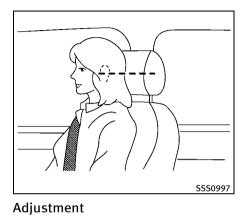
Adjust the headrest so the center is level with the center of your ears.
