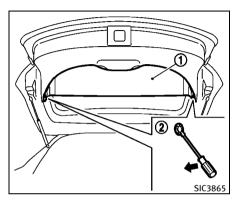
The rear cargo cover 1 can be removed from the lift gate.
