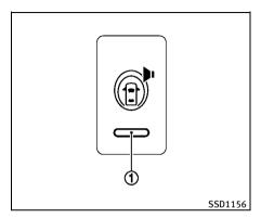
The warning systems switch will turn on and off the Lane Departure Warning (LDW) system and the Forward Collision Warning (FCW) system at the same time.
