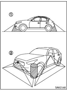
There are some areas where the system will not detect objects. When in the front or the rearview display, an object below the bumper or on the ground may not be detected (1). When in the bird-eye view, a tall object near the seam of the camera detecting areas will not appear in the monitor (2).
