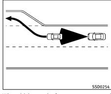
When driving on some roads, such as winding, hilly, curved, narrow roads, or roads which are under construction, the ICC sensor may detect vehicles in a different lane, or may temporarily not detect a vehicle traveling ahead. This may cause the ICC system to decelerate or accelerate the vehicle.
