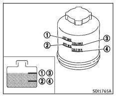
Check the fluid level in the reservoir.
