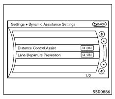
To set the DCA system to on or off, highlight the "Distance Control Assist" key, select ON or OFF and push the ENTER (2) button.
