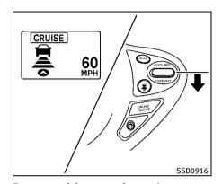
To set cruising speed, accelerate your vehicle to the desired speed, push the SET/COAST switch and release it. (Vehicle ahead detection indicator, set distance indicator and set vehicle speed indicator come on.) Take your foot off the accelerator pedal. Your vehicle will maintain the set speed.
