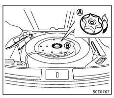
Remove jacking tools and the spare tire located under the luggage room.
