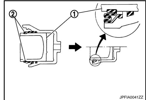
5. Secure piston boot with retaining ring (1).
