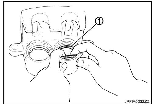
3. Apply rubber grease to piston boots (1). Cover the piston (2) end with piston boot, and then install cylinder side lip on piston boot securely into a groove on cylinder body.
