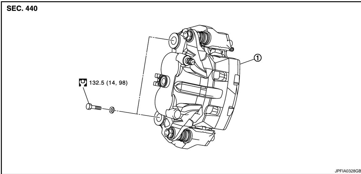
1. Brake caliper assembly
