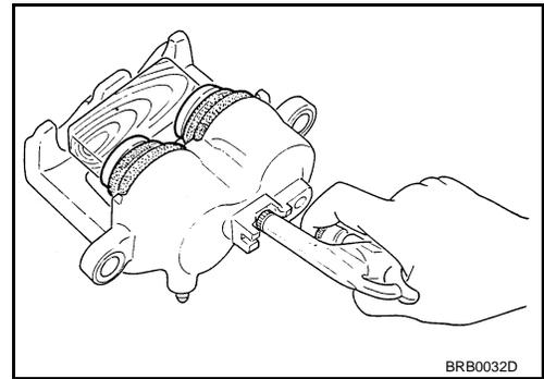
6. Remove piston seal from cylinder body using suitable tool.
