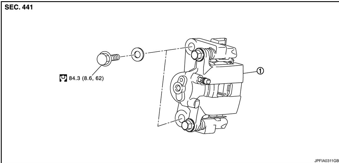
1. Brake caliper assembly
