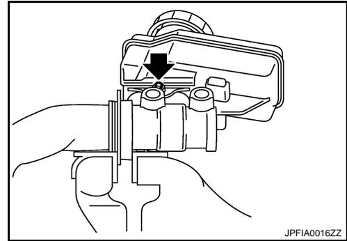
4. Tilt the reservoir tank so that a mounting pin can be inserted. Insert a mounting pin. Return the reservoir tank to the horizontal position. Insert another mounting pin into the pin hole on the opposite side in the same manner after the mounting pin passes through the cylinder body pin hole.
