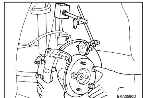
4. Find the installation position that has a minimum runout by shifting the disc rotor-to-wheel hub and bearing assembly installation position by one hole at a time if the runout exceeds the limit value.
