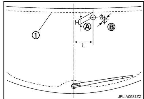
Insert a needle or similar object (A) into the spray opening (1) and move up/down and left/right to adjust the spray position.
