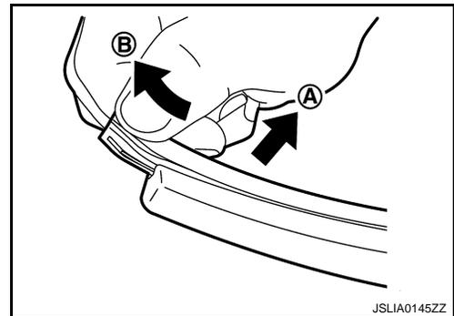
3. Insert a tip of new blade refill ("LOCK" mark is blade refill rear end) from the wiper blade rear end. And then slide until the hole of the blade refill fits in the tab of the wiper blade.
