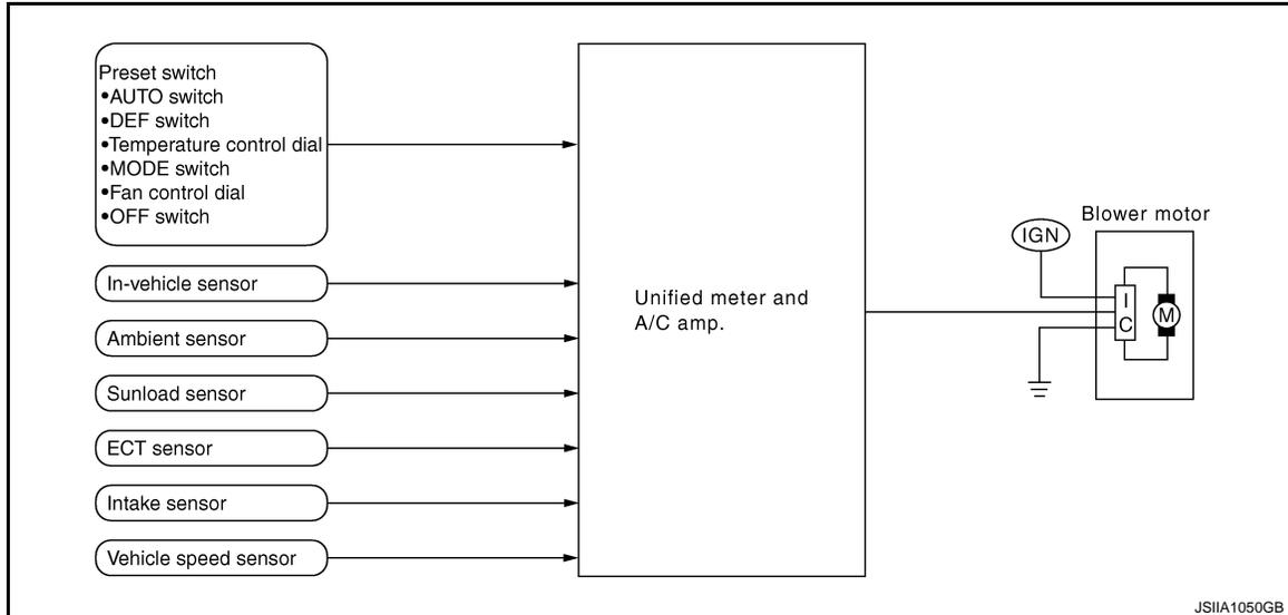
WITHOUT LEFT AND RIGHT VENTILATION TEMPERATURE SEPARATELY CONTROL SYSTEM : System Description
