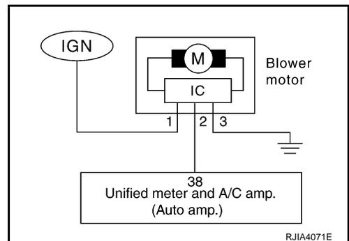
WITHOUT LEFT AND RIGHT VENTILATION TEMPERATURE SEPARATELY CONTROL SYSTEM : Component Function Check
