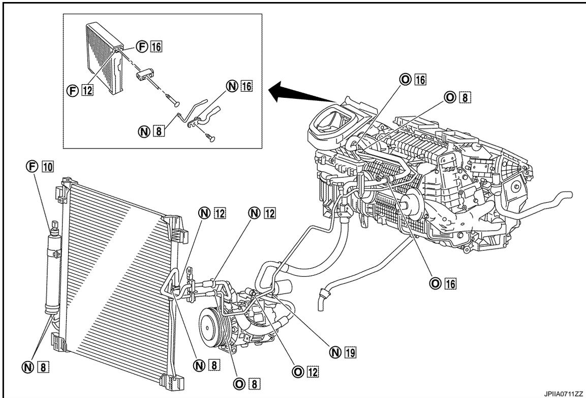
F. Former type refrigerant connection    N. New type refrigerant connection    O. One-touch joint
