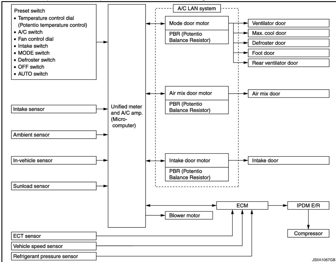
WITHOUT LEFT AND RIGHT VENTILATION TEMPERATURE SEPARATELY CONTROL SYSTEM : System Description
