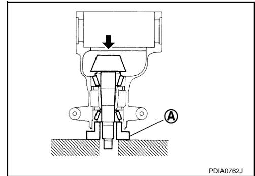
8. Using the drift (A) [SST: ST30720000 (J-25405)], install front oil seal as shown in figure.
