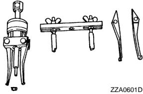
ZZA0601D                                                                                         | <ul style="list-style-type: none"> <li>• Removing side oil seal (right side)</li> <li>• Removing side bearing outer race</li> </ul> |
