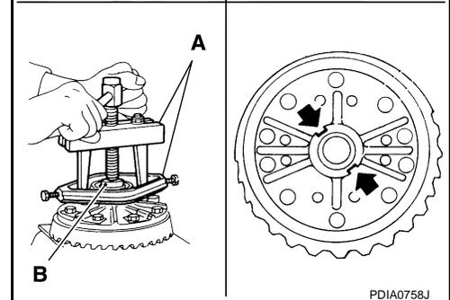
10. For proper reinstallation, paint matching marks on one differential case assembly.
