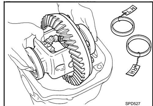
14. Insert selected left and right side bearing adjusting washers in place between side bearings and gear carrier. Refer to [DLN-170, "2WD : Adjustment"](#).
