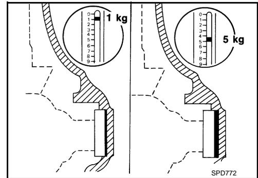
9. Record the total amount of washer thickness required for the correct carrier side bearing preload.
