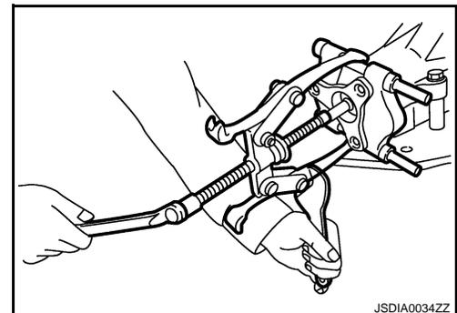
5. Press drive pinion assembly out of gear carrier.
