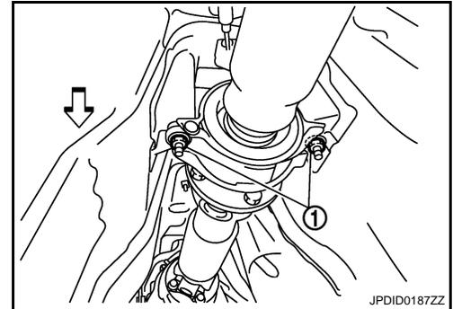
7. Remove propeller shaft assembly fixing bolts and nuts (←).
