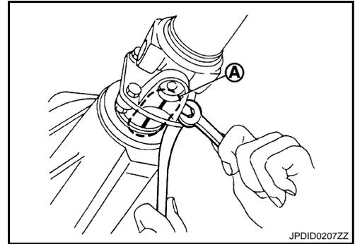
6. Put matching marks (A) on propeller shaft rebro joint and final drive companion flange.
