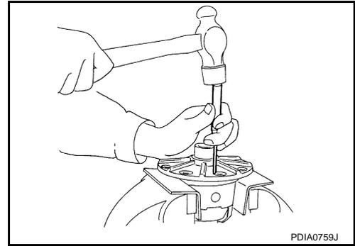
14. Remove pinion mate shaft.
