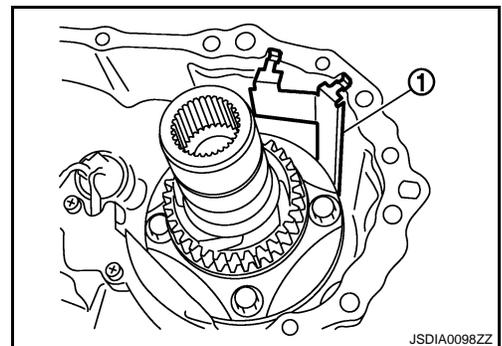
11. Install drive chain to front drive shaft.
