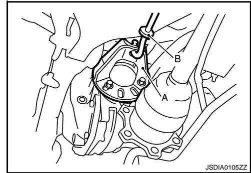
5. Remove side oil seal, using a flat-bladed screwdriver.
