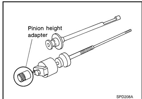
8. Position the side bearing discs, J-25269-4, and arbor firmly into the side bearing bores. Install the bearing caps and tighten bearing cap mounting bolts to the specified torque. Refer to [DLN-197, "AWD : Exploded View"](#).
