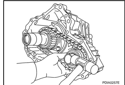
14. Remove oil gutter (1) from rear case.
