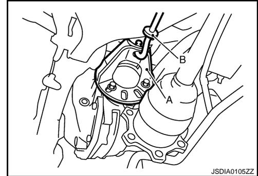
5. Remove side oil seal, using a flat-bladed screwdriver.
