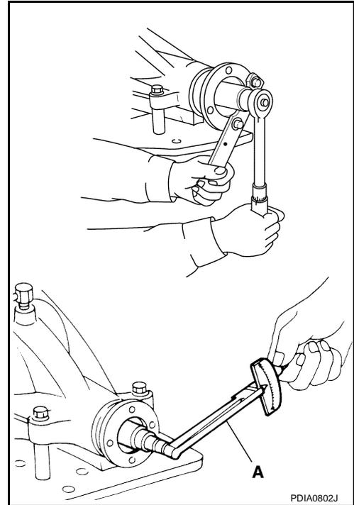
13. Install differential case assembly. Refer to [DLN-115, "Assembly"](#).
