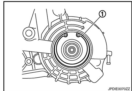
5. Install mainshaft assembly to rear case with the drift (A) [SST: ST35321000 ( — )].
