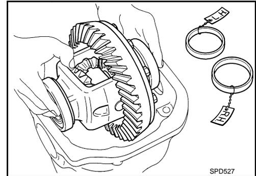
4. Insert left and right original side bearing adjusting washers in place between side bearings and gear carrier.
