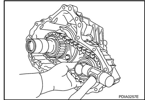
3. Remove front drive shaft front bearing with the drift (A) and puller (B).
