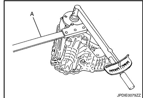
22. Install mainshaft oil seal until it is flush with end face of front case with the drift (A) [SST: ST30720000 (J-25405)].
