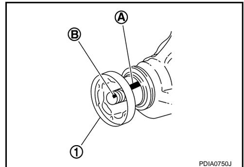
10. Remove drive pinion lock nut using the flange wrench.
