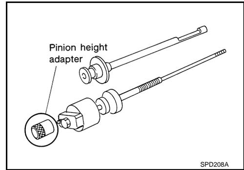
8. Position the side bearing discs, J-25269-4, and arbor firmly into the side bearing bores. Install the bearing caps and tighten bearing cap mounting bolts to the specified torque. Refer to [DLN-189, "2WD : Exploded View"](#).
