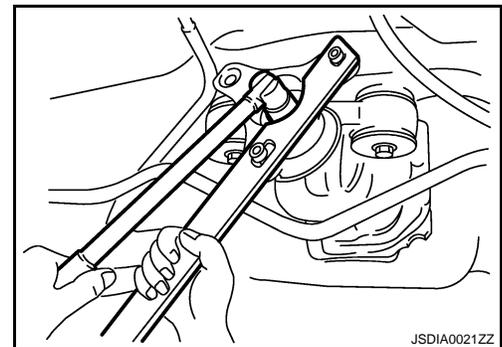
11. Remove companion flange using pullers.
