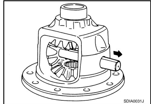
15. Turn pinion mate gear, then remove pinion mate gear, pinion mate thrust washer, side gear and side gear thrust washer from differential case.
