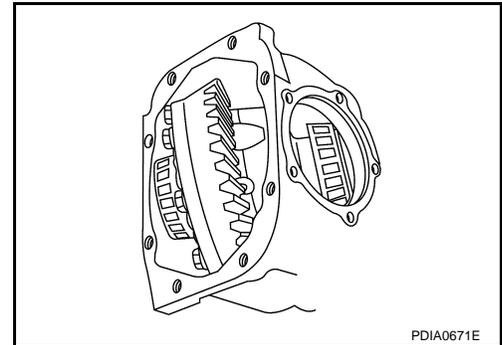
4. Install side bearing adjusting shim before disassembling or shim which thickness is the same as the one before disassembling.
