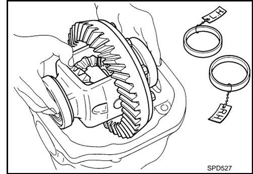
9. Remove side bearing inner race.
