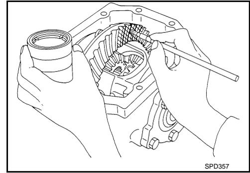
3. Rotate drive gear back and forth several times, check drive pinion gear to drive gear tooth contact.
