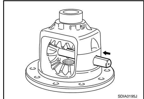
6. Measure side gear end play. If necessary, select the appropriate side gear thrust washers.
