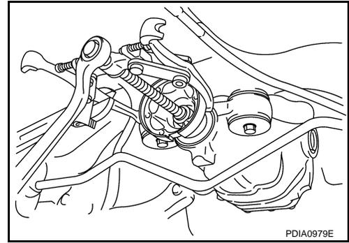
12. Remove front oil seal using the puller (A) [SST: KV381054S0 (J-34286)].
