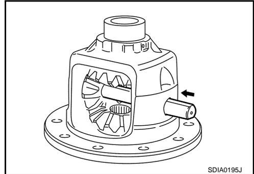
5. Measure side gear end play. If necessary, select the appropriate side gear thrust washers.
