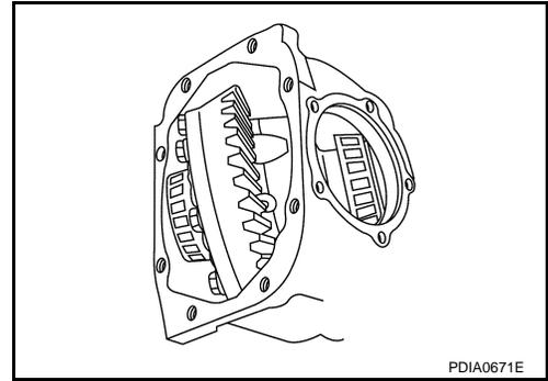
15. Install selected side bearing adjusting shim (1). Refer to [DLN-119, "Adjustment"](#).
