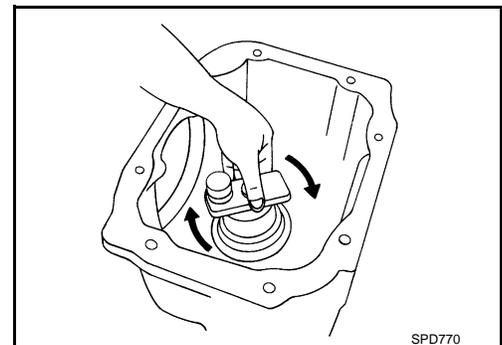
6. Measure the turning torque at the end of the J-34309-2 gauge anvil using preload gauge [SST: ST3127S000 (J-25765-A)].
