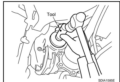
3. Install side flange with the following procedure.
