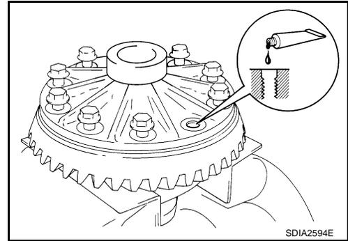
9. Install drive gear on the mounting bolts.
