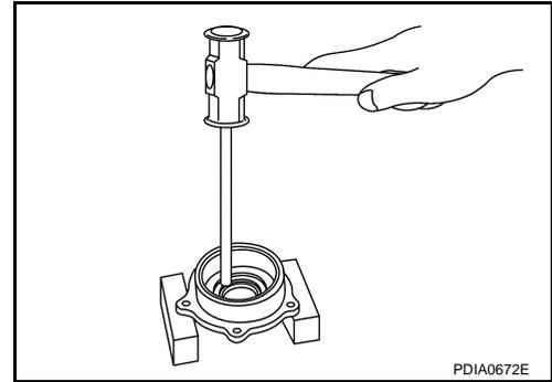
9. Remove side bearing outer race with puller (A) [SST: KV381054S0 (J-34286)].
