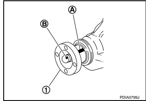
11. Apply anti-corrosion oil to the thread and seat of new drive pinion lock nut, and temporarily tighten drive pinion lock nut to drive pinion.
