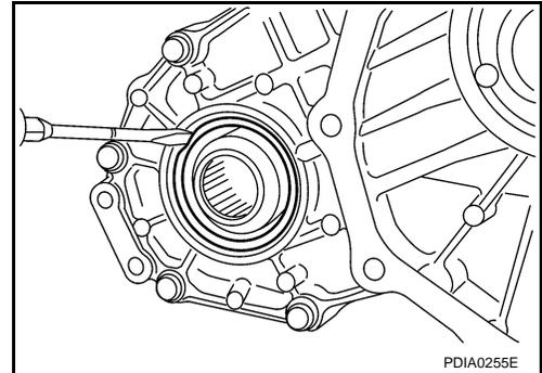
5. Put a matching mark (A) on the end of mainshaft. The mark should be in line with the mark (B) on the companion flange.
