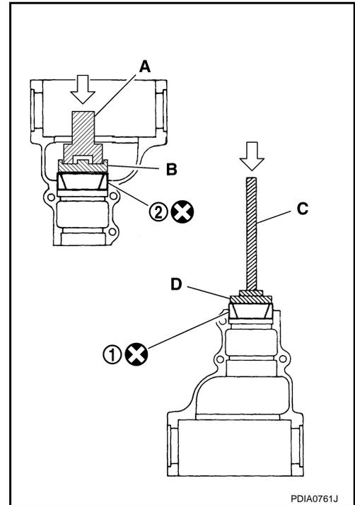
3. Install selected drive pinion height adjusting washer (2) to drive pinion. Press pinion rear bearing inner race (1) to it, using drift (A) [SST: ST30901000 (J-26010-01)].
