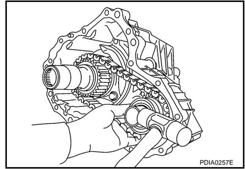
13. Install mainshaft bearing to front case with the drift (A) [SST: ST30621000 (J-25742-5)].
