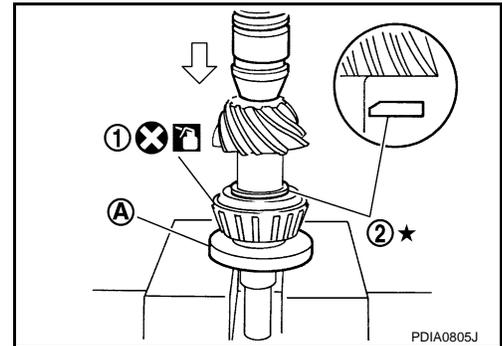
4. Assemble collapsible spacer to drive pinion.
