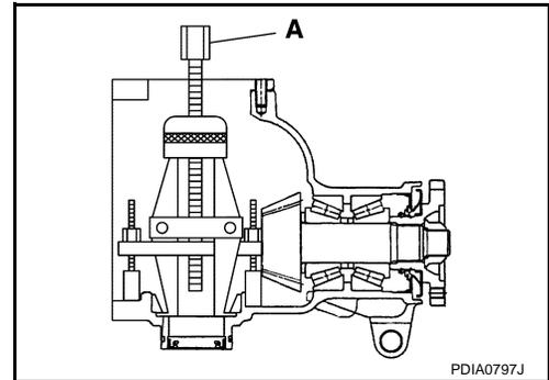
13. Remove side bearing inner race.
