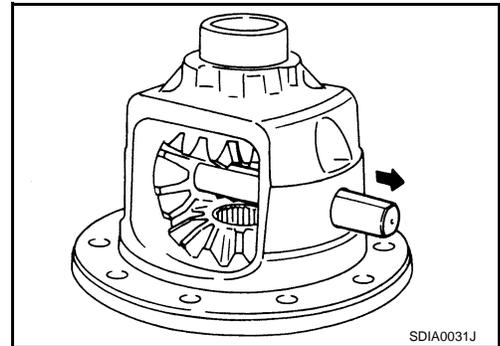
19. Turn pinion mate gear, then remove pinion mate gears, pinion mate thrust washers, side gears and side gear thrust washers from differential case.
