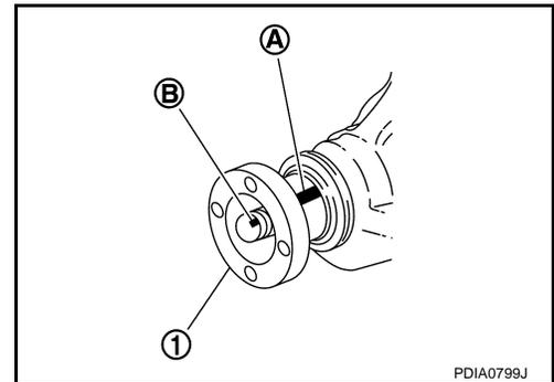
3. Temporarily tighten removed drive pinion lock nut to drive pinion.
