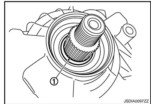
19. Install rear oil seal to rear case with the drifts within the dimension (L) shown as follows.
