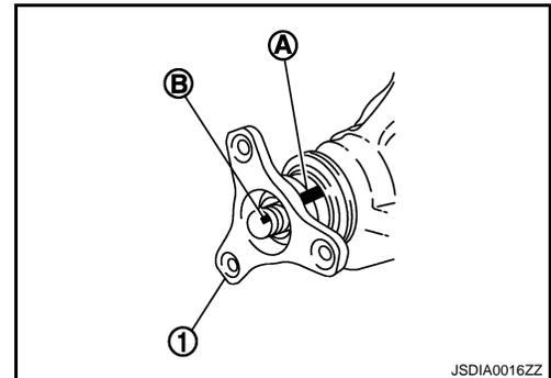
4. Remove companion flange using the suitable pullers.
