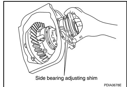
6. Install side retainer mounting bolts to the specified torque.
