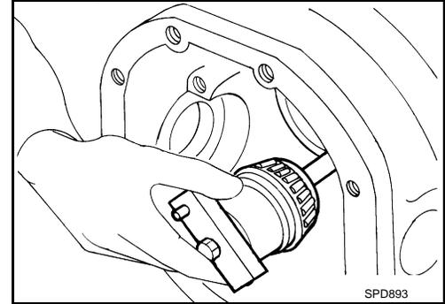
4. Assemble the pinion front bearing inner race and the J-34309-2 gauge anvil. Assemble them together with the J-34309-1 gauge screw in gear carrier. Make sure that the pinion height gauge plate, J-34309-16, turns a full 360 degrees. Tighten the two sections together by hand.
