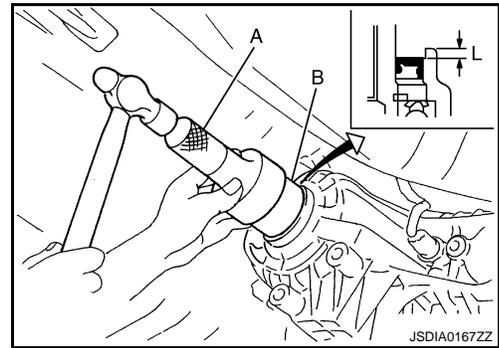
2. Align the matching mark (A) of mainshaft with the mark (B) of companion flange, then install the companion flange.
