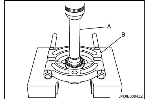
4. Remove front drive shaft rear bearing with the drift (A) and puller (B).
