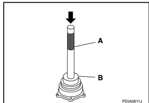
12. Press-fit side bearing outer race into gear carrier with the drift and the drift bar.
