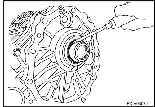
3. Remove front oil seal from front case with a suitable tool.
