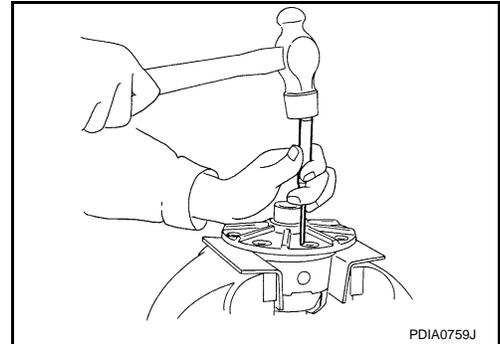
18. Remove pinion mate shaft.
