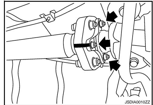
8. Slightly separate the rubber coupling (1) from the final drive companion flange (2).
