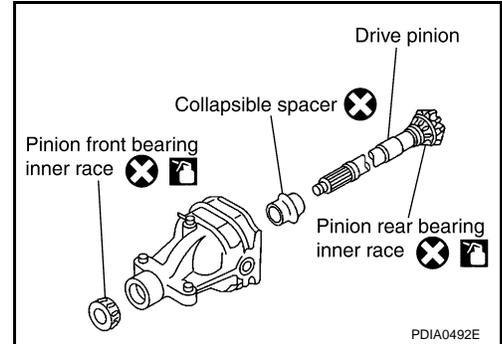
7. Using suitable spacer (A), press the pinion front bearing inner race to drive pinion as far as drive pinion nut can be tightened.
