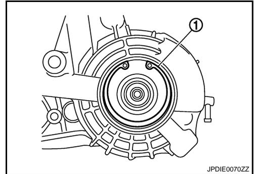
21. Remove rear bearing from rear case with the drifts.
