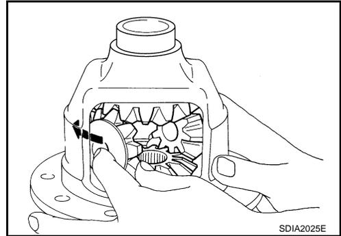
4. Align the lock pin holes on differential case with shaft, and install pinion mate shaft.
