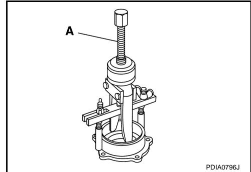
12. Remove side bearing outer race with puller (A) [SST: KV381054S0 (J-34286)].
