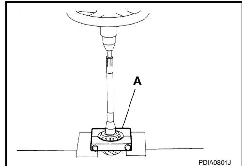
10. Tap pinion front/rear bearing outer races uniformly a brass rod or equivalent to removed.
