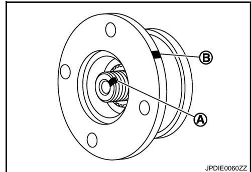
6. Remove companion flange with a puller (A) (commercial service tool).
