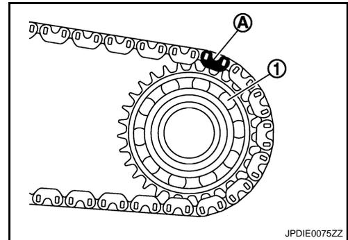
4. Install drive chain to mainshaft, and then install by tapping front drive shaft with plastic hammer. Press-fit rear bearing of front drive shaft to rear case.
