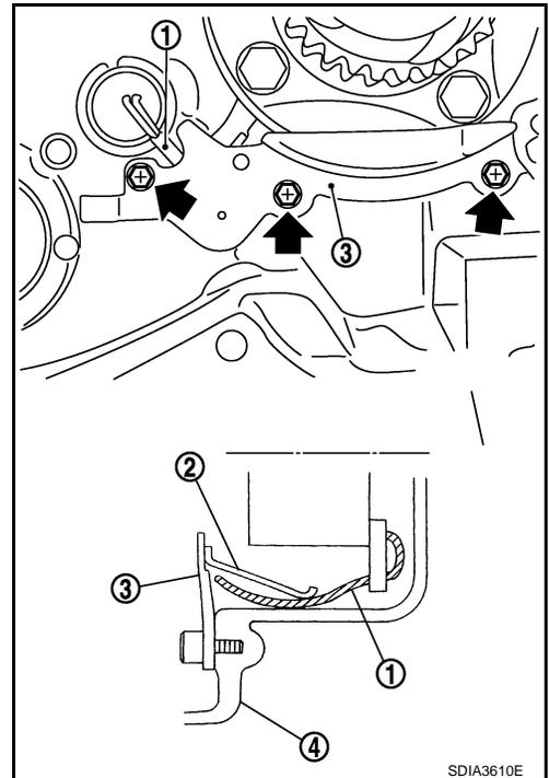
10. Install oil gutter (1) to rear case.
