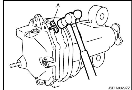
5. Using two 45 mm (1.77 in) spacers, mount carrier on the attachment (A) [SST: KV38100800 (J-25604-01)].
