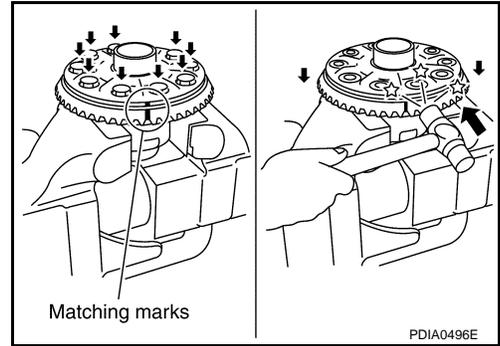
17. Remove lock pin of pinion mate shaft with a punch from drive gear side.
