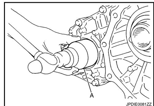
24. Apply sealant to threads of drain plug. Then, install it to rear case.
