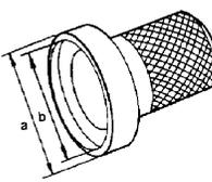
ZZA0702D                                    | <ul style="list-style-type: none"> <li>• Installing side oil seal (right side)</li> <li>• Installing front oil seal</li> </ul>      |
