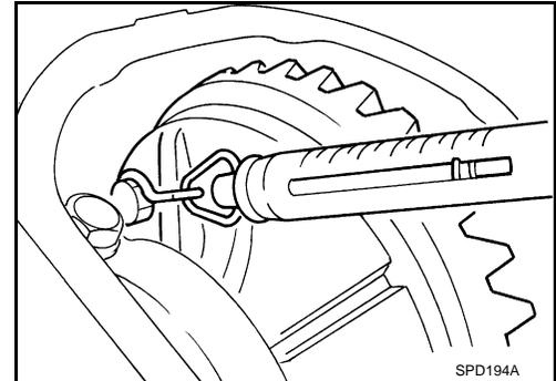
8. If the turning torque is outside the specification, use a thicker/thinner side bearing adjusting washer to adjust.
