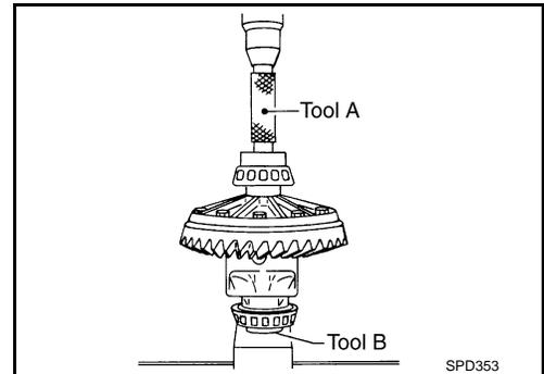
12. Install differential case assembly with side bearing outer races into gear carrier.
