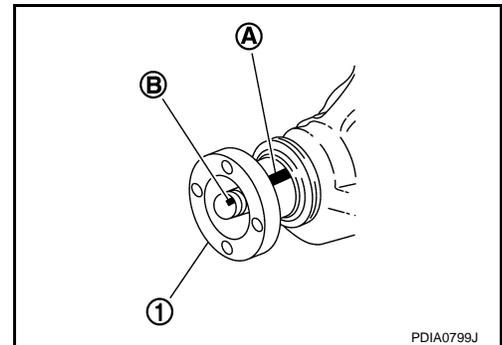
4. Remove companion flange using the suitable puller.
