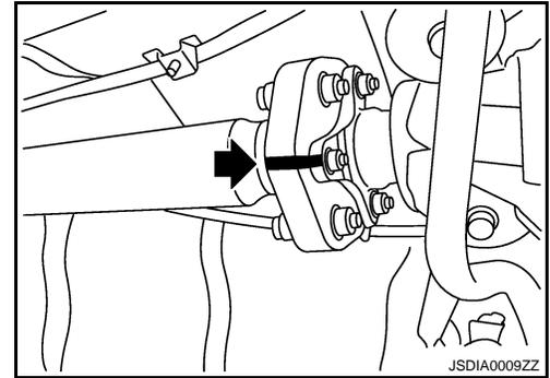
6. Loosen mounting nuts (1) of center bearing mounting brackets (upper/lower).
