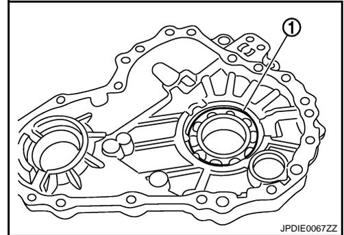
15. Apply liquid gasket to mating surface of rear case. Use Genuine Anaerobic Liquid Gasket or equivalent. Refer to [GI-15, "Recommended Chemical Products and Sealants"](#).
