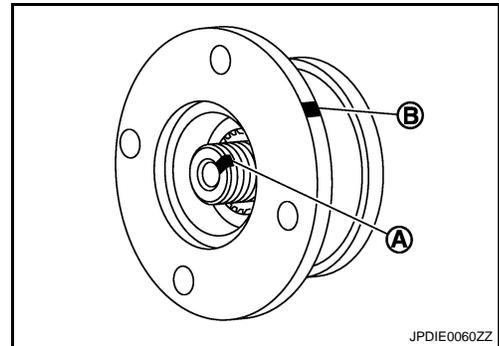
3. Using a flange wrench (A) (commercial service tool), install the self-lock nut of companion flange and tighten to the specified torque.
