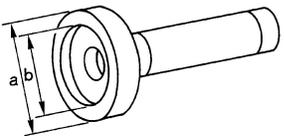
ZZA1143D                                        | Installing side shaft oil seal                                                                                                      |
