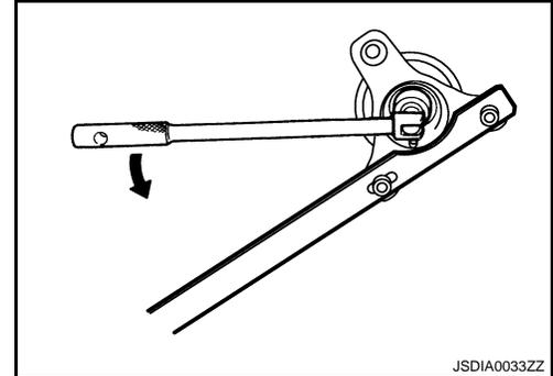
3. Put matching mark (B) on the end of drive pinion. The matching mark should be in line with the matching mark (A) on companion flange (1).
