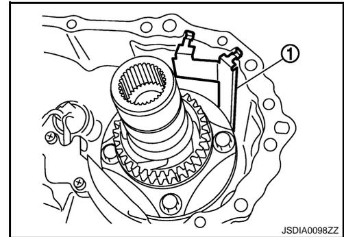
15. Remove oil cover bolts from rear case. And then, remove oil cover (1).
