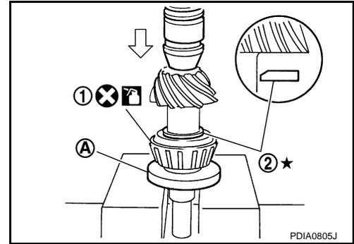
4. Assemble collapsible spacer to drive pinion.
