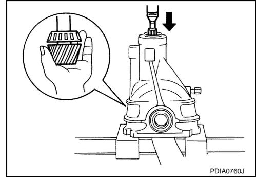
10. Remove pinion rear bearing inner race and pinion height adjusting washer with the replacer (A) (commercial service tool).
