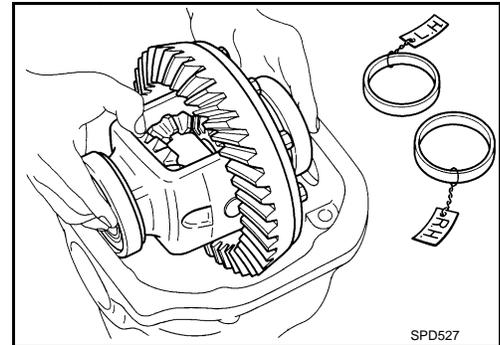
9. Remove side bearing inner race.
