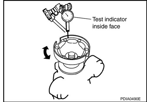
3. If the runout value is outside the runout limit, follow the procedure below to adjust.
