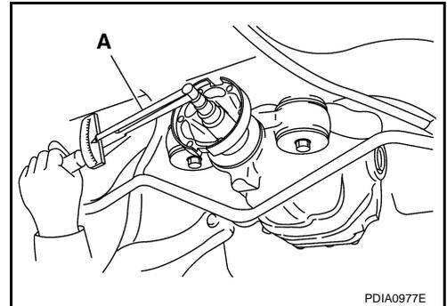
9. Put matching mark (B) on the end of the drive pinion. The matching mark should be in line with the matching mark (A) on companion flange (1).
