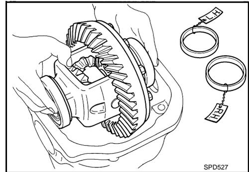
14. Insert selected left and right side bearing adjusting washers in place between side bearings and gear carrier. Refer to [DLN-183, "AWD : Adjustment"](#).
