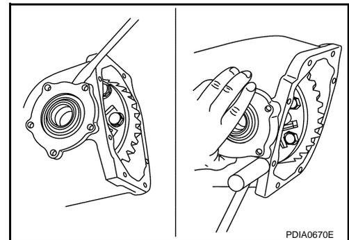
7. Remove differential case assembly from gear carrier.
