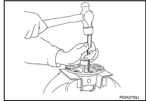
14. Remove pinion mate shaft.
