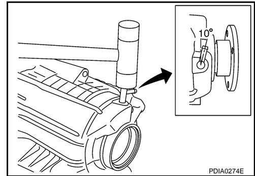
3. Install rear bearing to rear case with the drift (A) [SST: KV38104010 ( — )].
