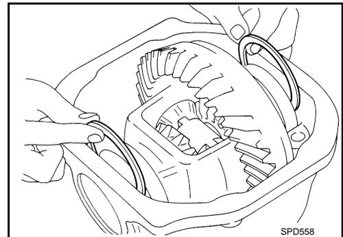
15. Align matching marks on bearing cap with that on gear carrier.
