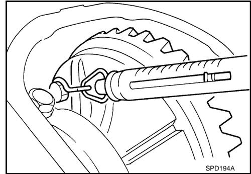
8. If the turning torque is outside the specification, use a thicker/thinner side bearing adjusting shim to adjust.
