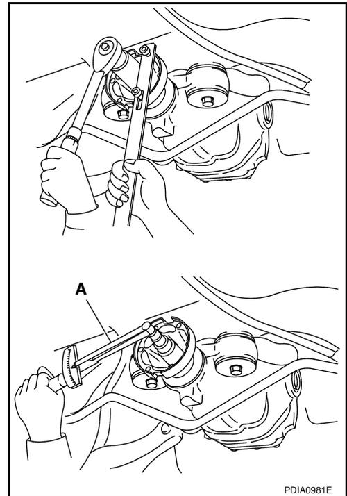
6. Fit a test indicator to the inner side of companion flange (socket diameter).
