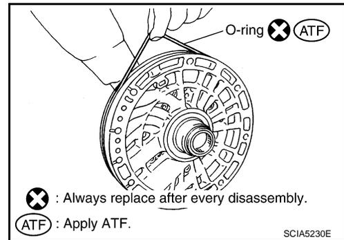
2. Install O-ring to oil pump housing.
