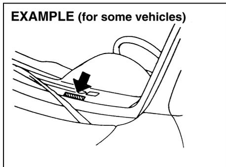
The Vehicle Identification Number (VIN) may be found in the location shown in the above illustrations. This number is used to register the vehicle. It is also used to assist your dealer when ordering parts or referring to special service information.
