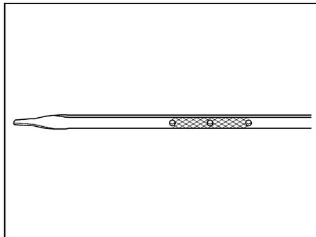
If the oil is below the cross-hatched area at the tip of the dipstick, you need to add at least one quart/liter of oil. But you must use the right kind. This section explains what kind of oil to use. For engine oil crankcase capacity, refer to “Capacities and Specifications” in this section.
