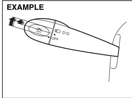
To turn the lights on or off, twist the knob on the end of the lever. There are three positions: in the "OFF" position all lights are off; in the middle position the front parking lights, taillights, license plate light, and instrument lights are on, but the headlights are off; in the third position the headlights come on in addition to the other lights.
