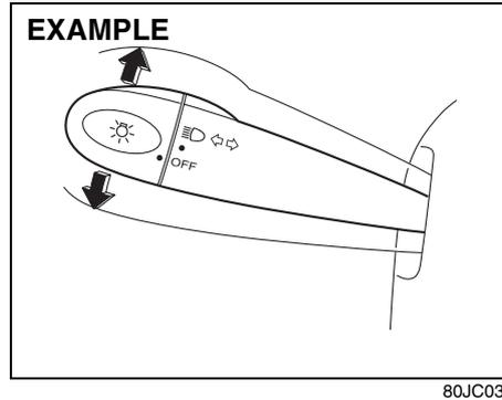
Some times, such as when changing lanes, the steering wheel is not turned far enough to cancel the turn signal. For convenience, you can flash the turn signal by moving the lever part way and holding it there. The lever will return to its normal position when you release it.
