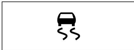
When one of the ESP® systems other than ABS is activated, the SLIP indicator light in the instrument cluster blinks 5 times per second.
