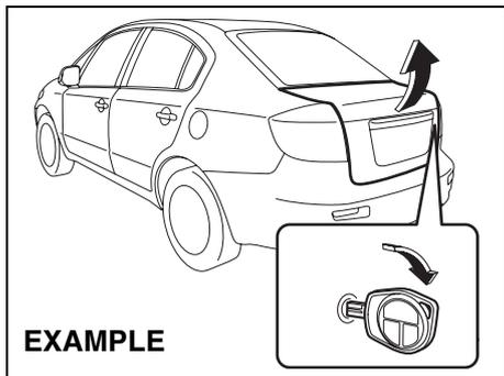
If your vehicle is equipped with a trunk lid key lock, you can open the trunk lid by using the key in the trunk lid lock. To open the trunk lid, insert the key and turn it clockwise to unlatch and lift the trunk lid.
