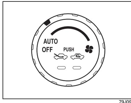
This is used to turn on the blower and to select blower speed.
