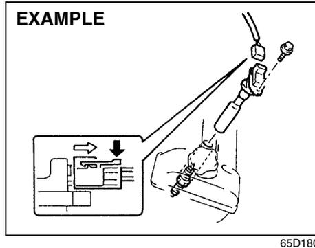
You should inspect spark plugs periodically for carbon deposits. When carbon accumulates on a spark plug, a strong spark may not be produced. Remove carbon deposits with a wire or pin and adjust the spark plug gap.
