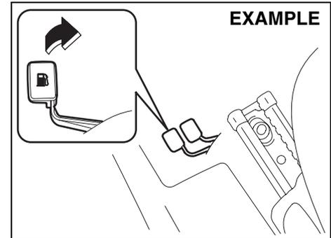
The fuel filler cap is located on the left rear side of the vehicle. The fuel filler door can be unlocked by pulling up the opener lever located on the outboard side of the driver's seat and can be locked by simply closing the door.
