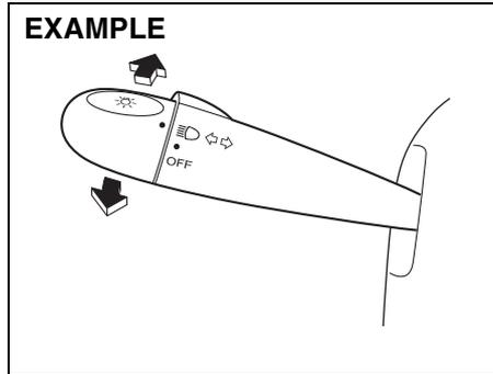
With the headlights on, push the lever forward to switch to the high beams (main beams) or pull the lever toward you to switch to the low beams. When the high beams (main beams) are on, a light on the instrument panel will come on. To momentarily activate the high beams (main beams) as a passing signal, pull the lever slightly toward you and release it when you have completed the signal.
