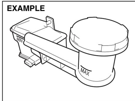
Check the brake fluid level by looking at the reservoir in the engine compartment. Check that the fluid level is between the "MAX" and "MIN" lines. If the brake fluid level is near the "MIN" line, fill it up to the "MAX" line with DOT3 brake fluid.
