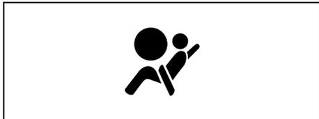
This light monitors inflators, crash sensors, seat belt pretensioners, the front passenger sensing system, and corresponding electrical circuits.
