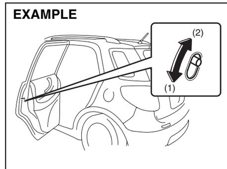
Each of the rear doors is equipped with a child lock which can be used to help prevent unwanted opening of the door from inside the vehicle. When the lock lever is in the "LOCK" position (1), the rear door can only be opened from outside. When the lock lever is in the "UNLOCK" position (2), the rear door can be opened from inside or outside.
