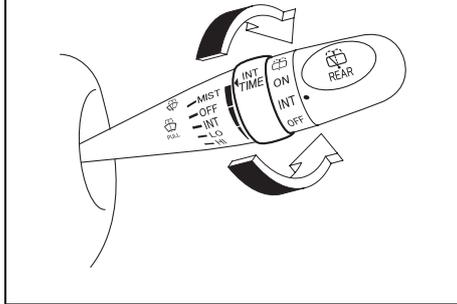
If the lever is equipped with the “INT TIME” control, turn the control forward or rearward to adjust the intermittent wiper operation to the desired interval.
