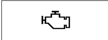
Your vehicle has a computer-controlled emission control system. A malfunction indicator light is provided on the instrument panel to indicate when it is necessary to have the emission control system serviced. The malfunction indicator light comes on when the ignition switch is turned to the "ON" position to let you know the light is working and goes out when the engine is started.
