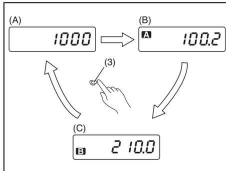
When the ignition switch is turned to "ON" with the lighting switch is in the "OFF" position, the display shows three types of indication; odometer (A), trip meter A (B) and trip meter B (C). Push the selector knob (3) quickly to switch the indication among the three.
