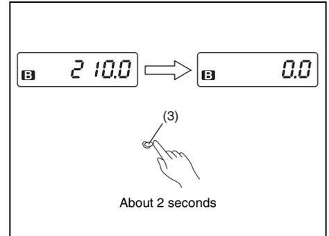
Hold in the selector knob for about 2 seconds to reset the trip meter to zero.
