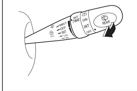
To spray windshield washer fluid, pull the lever toward you. The windshield wipers will automatically turn on at low speed if they are not already on and the “INT” position is equipped.
