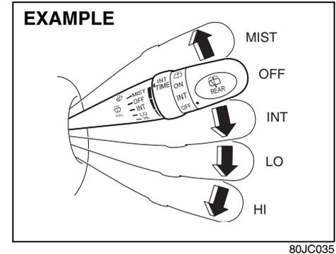
To turn the windshield wipers on, move the lever down to one of the three operating positions. In the “INT” position (if equipped), the wipers operate intermittently. The “INT” position is very convenient for driving in mist or light rain. In the “LO” position, the wipers operate at a steady low speed. In the “HI” position, the wipers operate at a steady high speed. To turn off the wipers, move the lever back to the “OFF” position.
