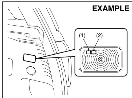
When you open the tailgate with the luggage compartment light switch in the “ON” position (1), the light comes on and remains on as long as you keep the tailgate open.
