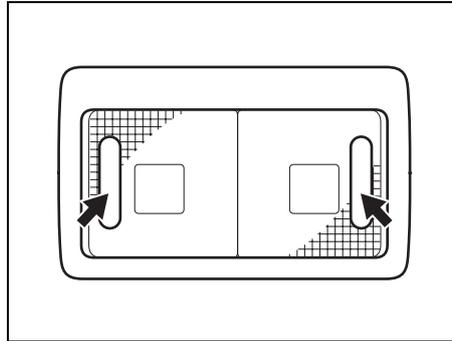
Push the switch to turn on the light and push it again to turn off the light.
