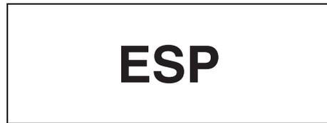
When the ESP® systems (other than ABS) have a system malfunction, the “ESP” warning light in the instrument cluster comes on.
