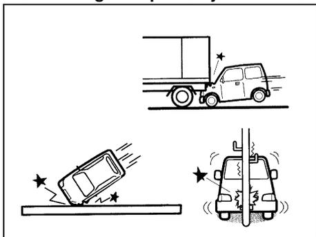
They are not designed to inflate in rear impacts, side impacts, rollovers or minor frontal collisions, since they would offer no protection in those types of accidents. Remember, since air bags deploy only one time during an accident, seat belts are needed to restrain occupants from further movements during the accident.
