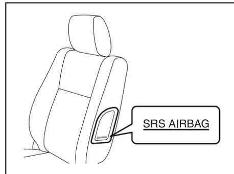
Side air bags are located in the part of the front seatbacks closest to the doors. The words “SRS AIRBAG” are molded into the side air bag cover to identify the location of the side air bags.
