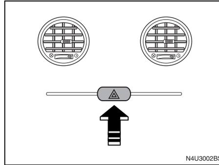
The hazard warning flasher button is located on the center of the instrument panel.
