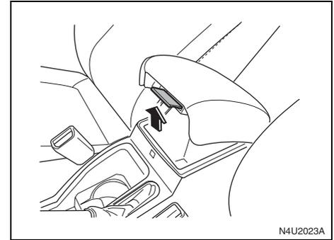
Your vehicle has a front armrest storage area. To open the storage area, pull up on the lift lever and raise the lid. To close the storage area, lower the lid and push it down until it latches securely.
