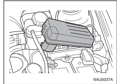
The engine compartment fuse block is located on the driver's side of the vehicle, near the battery. See "Engine Compartment Overview" in this section for more information on location.
