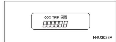
There are two independent trip odometers, which measure the distances your vehicle has traveled since you last reset this function.
