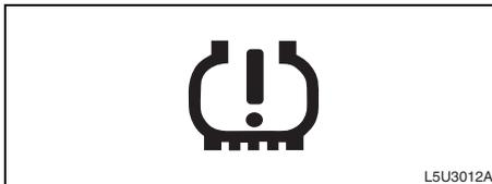
The light comes on when the tire pressure monitoring system detects that one or more of your tires is significantly under-inflated. This light will also come on for a few seconds and then go off when you turn the ignition to ON. This indicates that the tire pressure monitoring system is functioning properly.
