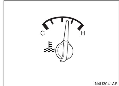
Your vehicle is equipped with an engine coolant temperature gauge. With the ignition in the ON position, this gauge shows the engine coolant temperature.
