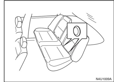
The disks are located near the base of the two rear outside seating positions.
