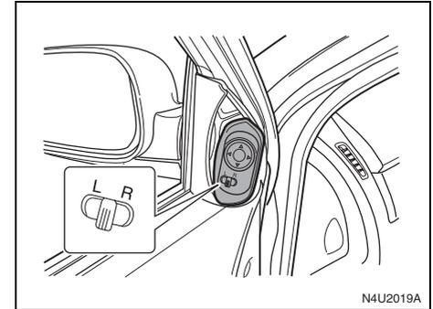
If your vehicle has this feature, the control for the power mirrors is located on the driver's side door trim.
