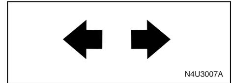
An arrow on the instrument panel cluster will flash in the direction of the turn or lane change.
