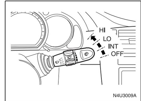
Use the windshield wiper/washer lever to operate the windshield wipers.
