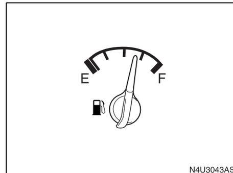
Your fuel gauge tells you approximately how much fuel you have left, when the ignition is on. When the indicator nears empty, the low fuel warning light will come on. You
