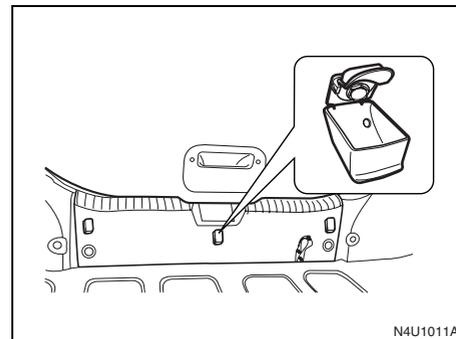
Top strap anchors are located at both sides and at the center of the lower rear tail member in the rear cargo area.
