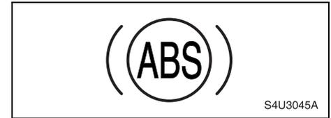
If there's a problem with the anti-lock brake system, this warning light will stay on. See "Anti-Lock Brake System Warning Light" in section 3.
