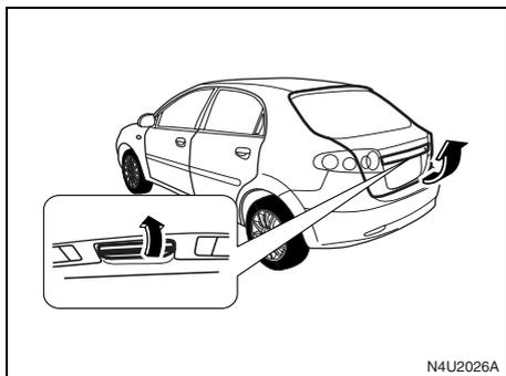
To open the liftgate from outside of the vehicle, insert the key into the lock cylinder and turn it clockwise. Then pull up the handle above the license plate to open the liftgate.
