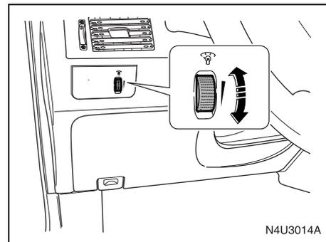
The thumbwheel for this feature is located on the instrument panel to the left of the steering wheel.
