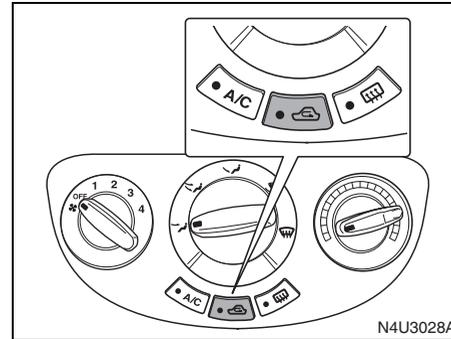
Press this button when driving in dusty conditions or to avoid traffic or outside fumes, and when quick cooling or heating of the passenger area is required. The indicator light will illuminate and interior air will be recirculated.
