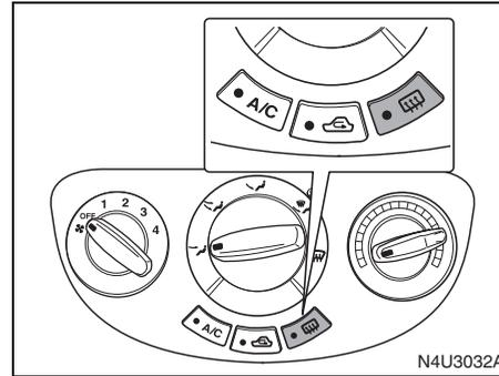
The rear window defogger uses a warming grid to remove fog or frost from the rear window. This feature will only work when the ignition is in ON.
