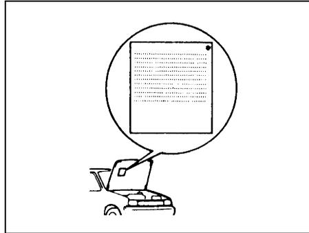
The EPA emission compliance label is located under the hood. It provides much of the information needed to perform an engine tune-up on your vehicle.
