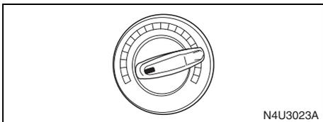
Turn this knob clockwise or counterclockwise to manually increase or decrease the temperature inside your vehicle. Turn the knob to the blue area to get cool air and to the red area to get warm air.
