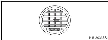
Use the lever located in the center of each outlet to change the direction of the airflow. Use the thumbwheel located next to the outlets to turn them on and off.
