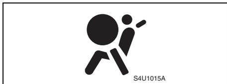
There is an air bag readiness light on the instrument panel, which shows the air bag symbol.
