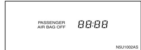
When the ignition key is turned to ON or START, the passenger air bag off indicator will light for several seconds as a system check. Then, after several more seconds, if the words “PASSENGER AIR BAG OFF” remain lit, it means that the passenger sensing system has turned off the right
