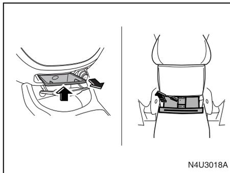
The front ashtray is located at the lower part of the center of the instrument panel. To remove the front ashtray for cleaning, open the ashtray fully, lift the inner case up and then pull it out.
