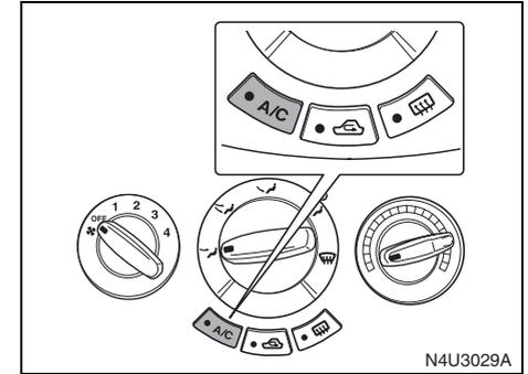
If your vehicle has air conditioning, follow these steps to use the system. Start the engine and set the fan control knob to the desired speed. The air conditioning compressor does not operate when the fan control knob is in the off position. Press the air conditioning button to turn the air conditioning system on. When this button is pressed, the indicator light on the button will come on to let you know the air conditioning is activated.
