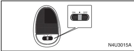
The switch on this lamp has three positions.
