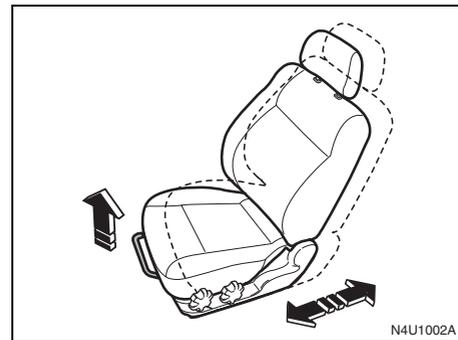
Pull up and hold the bar located under the front of the seat to unlock it. Slide the seat to where you want it and release the bar. Then try to move the seat with your body, to make sure the seat is locked into place.
