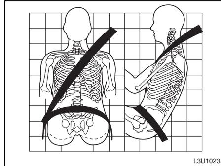
The lap part of the belt should be worn low and snug on the hips, just touching the thighs. In a crash, this applies force to the strong pelvic bones so you'd be less likely to slide under the lap belt. If you slid under it, the belt would apply force at your abdomen. This could cause serious or even fatal injuries. The shoulder belt should go over the shoulder and across the chest. These parts of the body are best able to take belt restraining forces.
