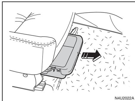
Your vehicle may have a sliding storage tray located under the front passenger seat. To use the tray, pull up on the end of the tray and pull it toward the instrument panel. Push the tray toward the seat to return it to its original position.
