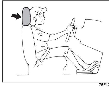
Head restraints are designed to help reduce the risk of neck injuries in case of an accident. Adjust the head restraint to the position which places the center of the head restraint closest to the top of your ears. If this is not possible for very tall passengers, adjust the head restraint as high as possible.
