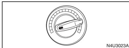
Turn this knob clockwise or counterclockwise to manually increase or decrease the temperature inside your vehicle. Turn the knob to the blue area to get cool air and to the red area to get warm air.
