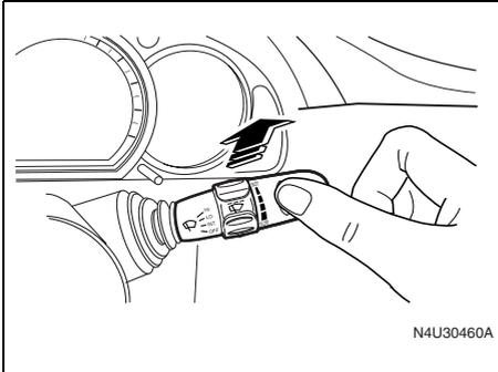
If your vehicle has this feature, operate the rear window washer/wiper system by pushing the windshield wiper/washer lever away from you. The wiper operates continuously when the lever is in the first position.
