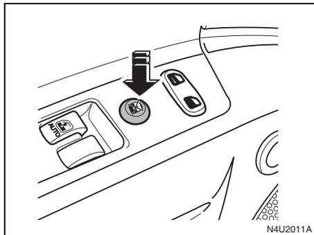
The driver's power window controls also include a lockout button.
