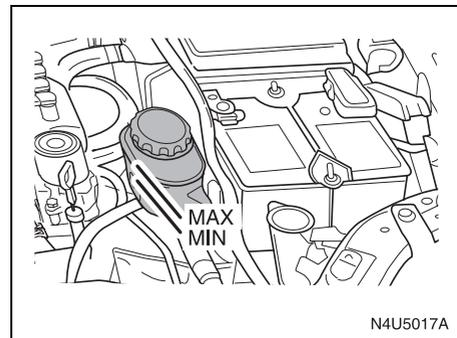
Turn the key off and then check the fluid level. The level should be between the MIN and MAX marks on the reservoir. If the level is below the MIN mark, add power steering fluid.
