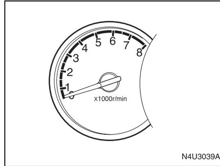
The tachometer shows your engine speed in revolutions per minute (rpm).
