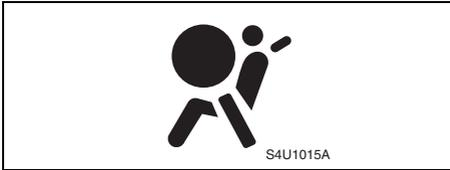
There is an air bag readiness light on the instrument panel, which shows the air bag symbol.
