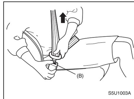
To unfasten the belt, push the red button on the buckle (B) and allow the belt to retract.
