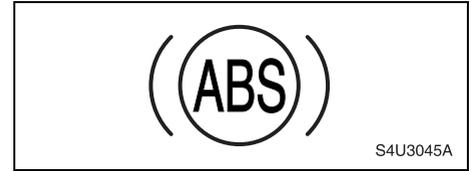
If there's a problem with the anti-lock brake system, this warning light will stay on. See "Anti-Lock Brake System Warning Light" in section 3.
