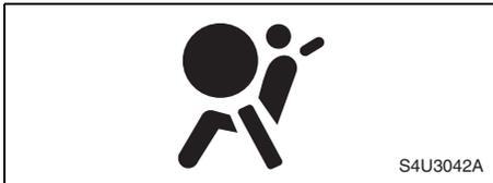
This light will come on when you start your vehicle, and it will flash for a few seconds. Then the light should go out. This means the system is ready.
