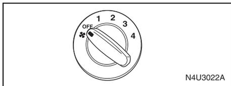
Turn this knob clockwise or counterclockwise to increase or decrease the fan speed. In any setting other than off, the fan will run continuously with the ignition on.
