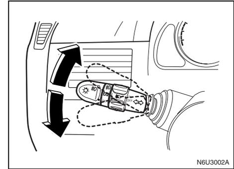
To signal a turn, move the lever all the way up or down. When the turn is finished, the lever will return automatically.
