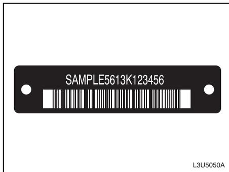
This is the legal identifier for your vehicle. It appears on a plate in the front corner of the instrument panel, on the driver's side. You can see it if you look through the windshield from outside your vehicle. The VIN also appears on the Vehicle Certification and Service Parts labels and the certificates of title and registration.
