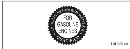
If you choose to perform the engine oil change service yourself, be sure the oil you use has the starburst symbol on the front of the oil container. If you have your oil changed for you, be sure the oil put into your engine is American Petroleum Institute certified for gasoline engines.
