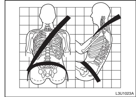
The lap part of the belt should be worn low and snug on the hips, just touching the thighs. In a crash this applies force to the strong pelvic bones so you'd be less likely to slide under the lap belt. If you slid under it, the belt would apply force at your abdomen. This could cause serious or even fatal injuries. The shoulder belt should go over the shoulder and across the chest. These parts of the body are best able to take belt-restraining forces.
