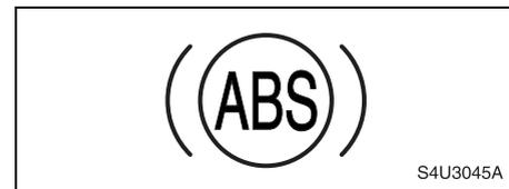
If your vehicle has an anti-lock brake system, the ABS warning light comes on briefly when you turn the ignition ON. This indicates that the system is performing a self-check and the indicator bulb is operating properly. The light should go out after several seconds.
