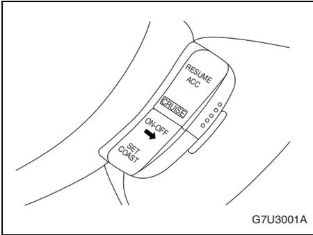
The cruise control pad is located on the right side of the steering wheel.
