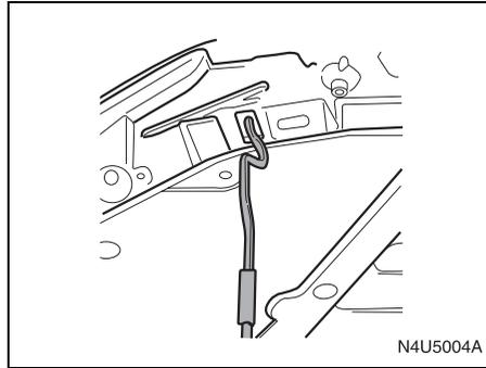
3) Lift the hood, release the hood prop from its retainer and place the hood prop into the slot in the hood.
