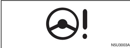
If your vehicle has Speed Sensitive Power Steering (SSPS), this warning light will come on briefly when you turn the ignition to ON as a check to show you the bulb is working.
