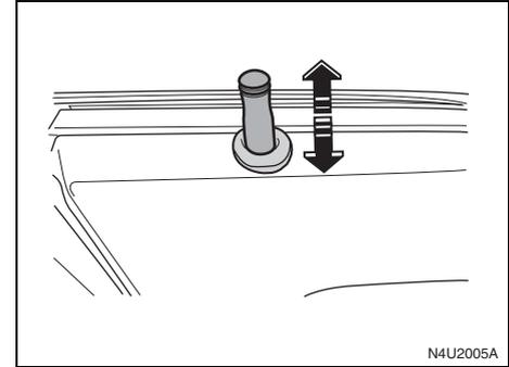
All doors, except the driver's door, can be locked from the outside by pushing down the manual door lock and then closing the door. The driver's door lock cannot be pushed in while the door is open. Upon leaving the vehicle, the driver's door can only be locked from the outside by using the key or the optional remote keyless entry transmitter.
