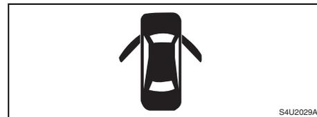
If one of the doors on your vehicle is not closed completely while the ignition is on, the door ajar light on the instrument panel will come on and stay on until the doors are closed and completely latched.
