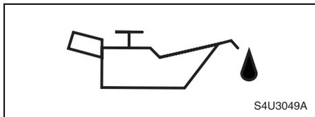
If the oil pressure light appears on the instrument cluster, it means you need to check your engine oil level right away.
