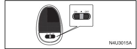
The switch on this lamp has three positions.
