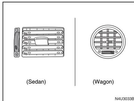
Use the lever located in the center of each outlet to change the direction of the airflow. Use the thumbwheel located next to the outlets to turn them on and off.
