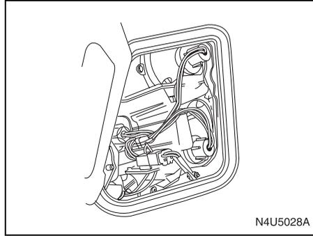
To replace a tail/stop lamp bulb, a rear turn signal lamp bulb, or a rear backup lamp bulb:
