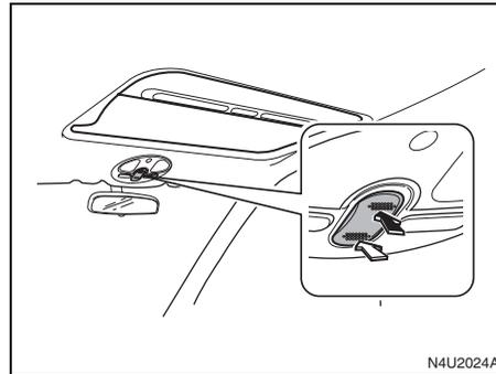
To open the sunroof to the vent position, push the front part of the switch. To return the sunroof to its original position, push the rear part of the switch and hold it until the sunroof reaches the desired position.
