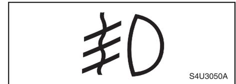
If your vehicle has this feature, the fog lamps indicator light will come on when the fog lamps are in use.
