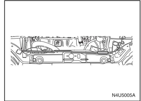
4) Before closing the hood, be sure all the filler caps are on properly. Then lift the hood to relieve pressure on the hood prop. Remove the hood prop from the slot in the hood and return the prop to its retainer. Lower the hood 12 in (30 cm) above the vehicle and release it to latch fully. Check to make sure the hood is closed and repeat the process if necessary.
