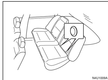
The disks are located near the base of the two rear outside seating positions.
