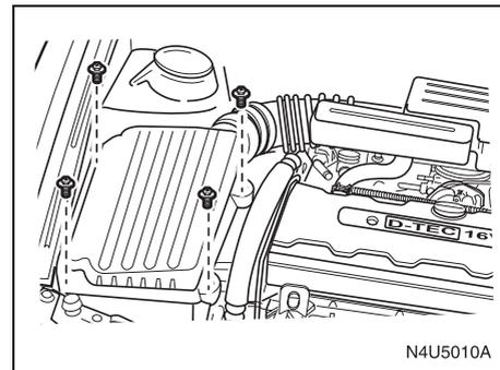
The engine air cleaner/filter is located on the passenger's side of the engine compartment. See "Engine Compartment Overview" in this section for more information on location.
