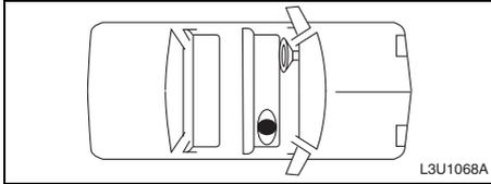
Your vehicle has a right front passenger air bag. A rear seat is a safer place to secure a child restraint. See “Where to Put the Restraint” in this section.
