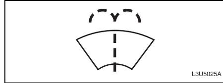
Open the cap with the washer symbol on it. Add washer fluid until the tank is full.
