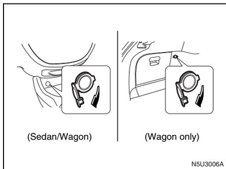
To use the outlet, remove the cover. When not in use, always cover the outlet with the protective cap. The accessory power outlet is operational when the ignition is in the ACC or ON positions.
