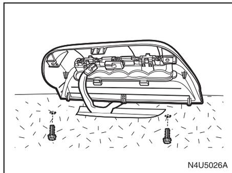
To replace a center high-mounted stop lamp bulb:
