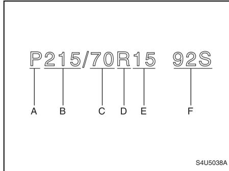
The following illustration shows an example of a typical passenger car tire size.
