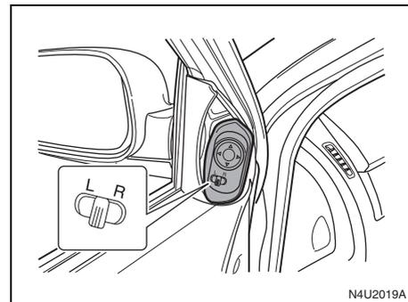
If your vehicle has this feature, the control for the power mirrors is located on the driver's side door trim.
