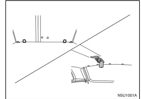
Top strap anchors are located at both sides of the floor mat in the rear cargo area behind the rear seat and at the center of the upper rear roof.
