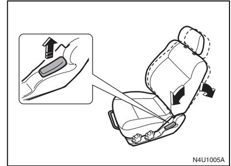
To adjust the seatback angle, lift the lever located on the outboard side of the seat and move the seatback to the desired position.
