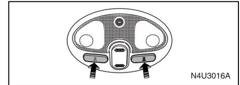
Your vehicle has map lamps. To turn a lamp on, press the button next to it. Press the button again to turn it off.
