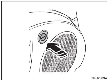
Press the remote trunk release button, located on the side of the driver's door trim, to release the trunk lid.
