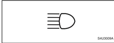
When the high beams are on, a light on the instrument panel cluster also will be on if the ignition is ON.
