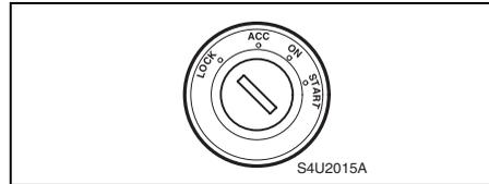
With the key in the ignition switch, you can turn the key to four different positions.
