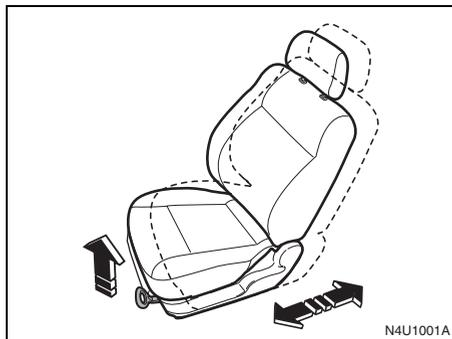
Pull up and hold the lever located under the front of the seat to unlock it. Slide the seat to where you want it and release the lever. Then try to move the seat forward or rearward to make sure the seat is locked into place.
