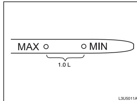
If the oil is at or below the MIN mark, then you'll need to add at least one quart of oil. But you must use the right kind. This section explains what kind of oil to use. For engine oil crankcase capacity, see “Capacities and Specifications” in this section.
