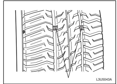
One way to tell when it's time for new tires is to check the tread wear indicators, which will appear when your tires have only 1/16 inch (1.6 mm) or less of tread remaining.
