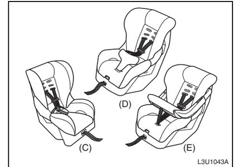
A forward-facing child seat (C–E) provides restraint for the child's body with the harness and also sometimes with surfaces such as T-shaped or shelf-like shields.
