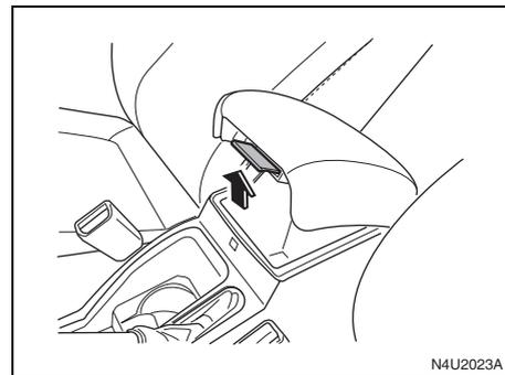
Your vehicle has a front armrest storage area. To open the storage area, pull up on the lift lever and raise the lid. To close the storage area, lower the lid and push it down until it latches securely.
