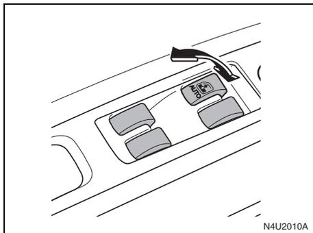
If your vehicle has this feature, the power window switches are located on the armrest on the driver's door. In addition, each passenger door has a switch for its own window. The ignition must be ON to use the power windows.
