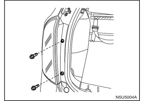
To replace a tail/stop lamp bulb, a rear turn signal lamp bulb, or a rear backup lamp bulb:
