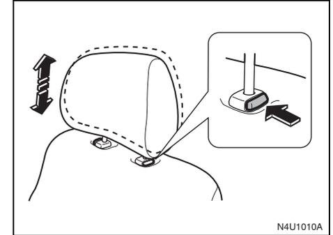
Push in the release button and press downward on the head restraint in order to adjust the position downward.
