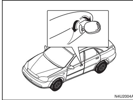
From the outside, use your key or the optional keyless entry transmitter. See “Remote Keyless Entry System” in this section.
