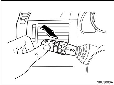
To change the headlamps from low beam to high beam, push the turn signal multifunction lever away from you.
