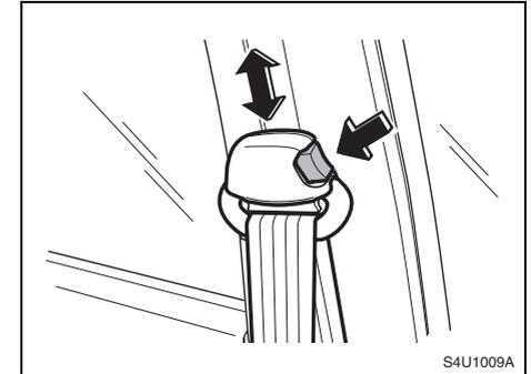
To move it down, squeeze the release button and move the height adjuster to the desired position. You can move the adjuster up just by pushing up on the shoulder belt guide. After you move the adjuster to where you want it, try to move it down without squeezing the release button to make sure it has locked into position.
