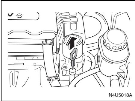
The windshield washer fluid reservoir is located in the front of the engine compartment on the driver's side. See "Engine Compartment Overview" in this section for more information on location.
