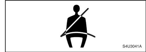
The safety belt light will also come on and stay on until the driver's safety belt is buckled.
