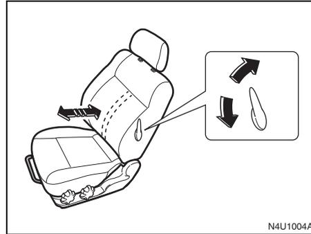
To adjust the front seat lumbar support, use the lever located on the outboard side of the seatback.
