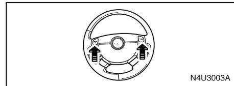
You can sound the horn by pressing the horn symbol on your steering wheel.
