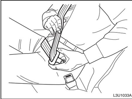
Pull up on the latch plate to make sure it is secure. Make sure the release button on the buckle is positioned so you would be able to unbuckle the safety belt quickly if you ever had to.
