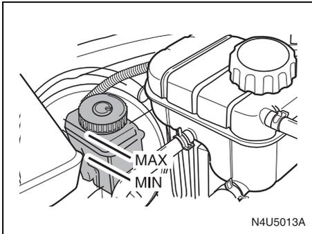
To check the fluid level, look on the side of the reservoir. If the fluid level is between
