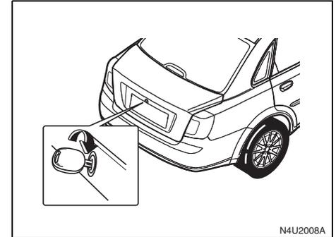
To open the trunk from the outside, insert the key and turn it clockwise in the trunk lock cylinder or use the remote keyless entry transmitter if your vehicle has one.
