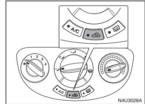
Press this button when driving in dusty conditions or to avoid traffic or outside fumes, and when quick cooling or heating of the passenger area is required. The indicator light will illuminate and interior air will be recirculated.
