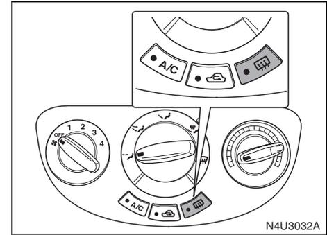
The rear window defogger uses a warming grid to remove fog or frost from the rear window. This feature will only work when the ignition is in ON.
