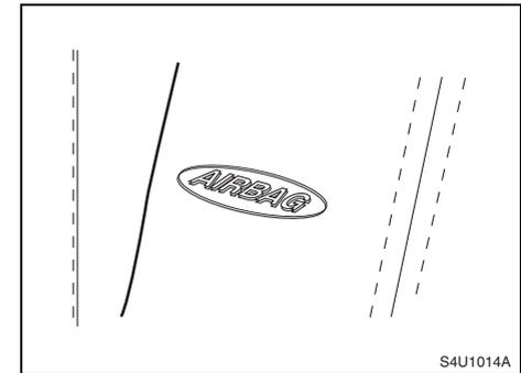
The words AIR BAG will appear on the side of the front seatback closest to the door, to indicate the presence of a side impact air bag.
