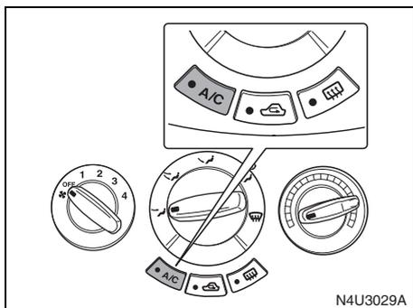
If your vehicle has air conditioning, follow these steps to use the system. Start the engine and set the fan control knob to the desired speed. The air conditioning compressor does not operate when the fan control knob is in the off position. Press the air conditioning button to turn the air conditioning system on. When this button is pressed, the indicator light on the button will come on to let you know the air conditioning is activated.
