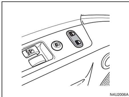
If your vehicle has this feature you can unlock or lock the doors on your vehicle using the driver's door lock switch. Push down the front part of the switch to unlock the doors. Push down the back part of the switch to lock the doors.
