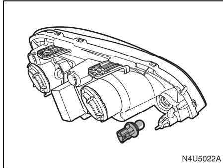
To replace a front turn signal lamp bulb:
