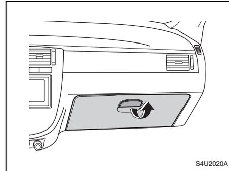
Open the glove box by pulling the bottom of the handle upward. Close the glove box with a firm push.
