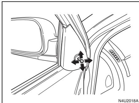
Adjust the outside mirrors with the control levers on the driver's and passenger's doors.
