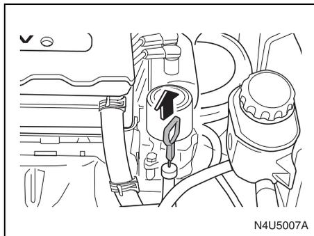
Use the engine oil dipstick to check the oil level. The dipstick's handle will be a yellow ring. See “Engine Compartment Overview” in this section for the location of the engine oil dipstick.
