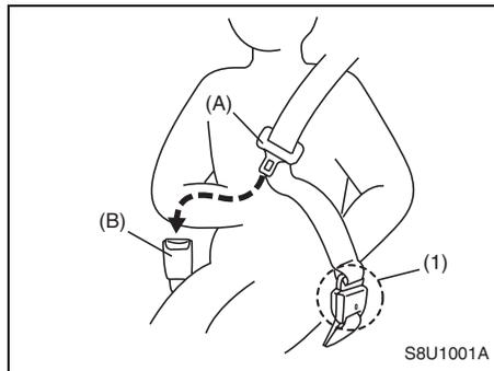
Before fastening the rear center belt, push the connector latch plate (1) at the end of the safety belt strap into the connector and make sure the webbing is not twisted. To fasten the belt, sit up straight and well back in the seat, pull the latch plate (A) across your body and press it into the buckle (B) until you hear a “click”.
