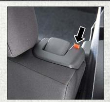
Seatback Latch Indicator Unlocked **Position**
