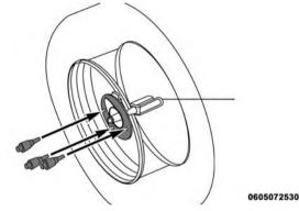
Wheel/Bolts Attaching To Mounting Bracket 5. Follow the steps above for proper spare tire stowage.
