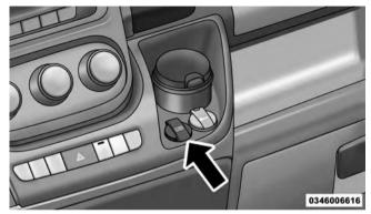
**Passenger Compartment USB Charging Port NOTE:** If the device battery to be charged is completely depleted, it may take awhile to charge.
