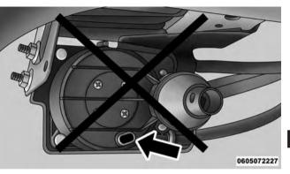
Winch Mechanism NOT Properly Engaged (Black Window Will Appear)
