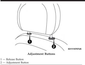
**NOTE:** Do not reposition the head restraint 180 degrees to the incorrect position in an attempt to gain additional clearance to the back of the head.
