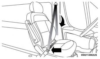
Inserting Latch Plate Into Buckle
