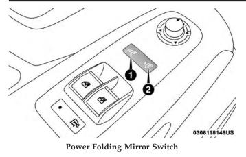
1 — Power Folding Mirror (Normal Driving Position) 2 — Power Folding Mirror (Fold In Position) The power folding mirrors are designed to be folded and unfolded using the power folding switch. If the mirrors are manually folded, the mirror head may appear loose.
