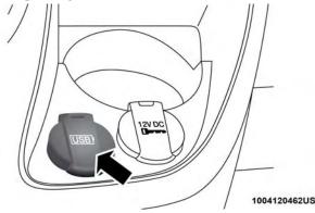
**Passenger Compartment USB Charging Port NOTE:** If the device battery to be charged is completely depleted, it may take awhile to charge.
