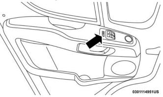
Load Compartment Power Door Lock Switch
