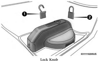
To open the jack kit container you must push the containers release to separate the top and bottom.
