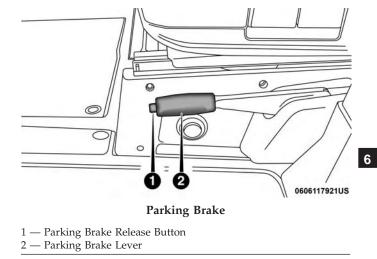
When the parking brake is applied with the ignition switch in the MAR (ACC/ON/RUN) position, the Brake Warning Light in the instrument cluster will illuminate.
