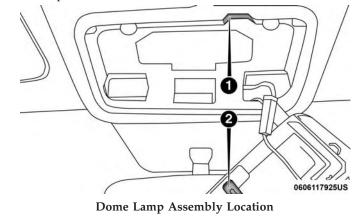
1. Spring Tension Relief Access 2. Dome Lamp Assembly
