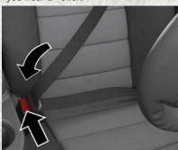
**Inserting Latch Plate Into Buckle**
