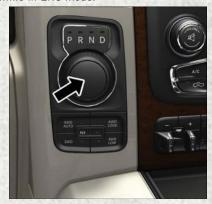
**Electronic Transmission Gear Selector**
