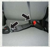
Mini-Latch And Mini-Buckle Connected
