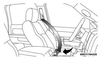
**Inserting Latch Plate Into Buckle**
