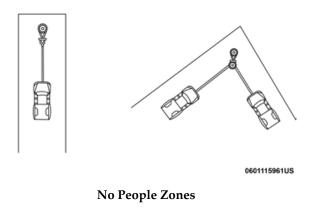
14. Begin winching. With the winching vehicles engine on and light tension already on the synthetic rope, begin winching slowly and steadily. Be sure that the rope is winding evenly and tightly around the spooling drum. For additional assistance, the winched vehicle can be slowly driven while being pulled by the winch. Continue pulling until the vehicle is on stable ground. If you are able to drive the vehicle, the winching operation is complete.
