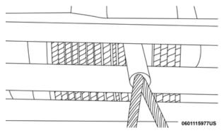
Synthetic Rope Neatly Wound Around The Spooling Drum
