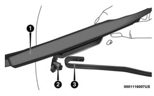
Removing Wiper From Wiper Arm
