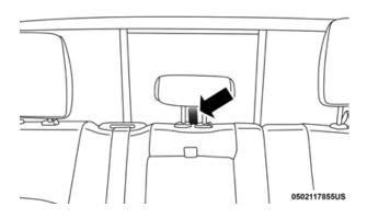
Crew Cab Center Tether Anchorage With Head Restraint In Raised Position
