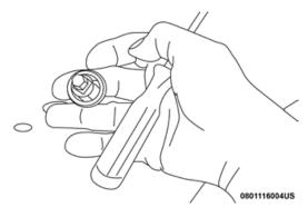
Removing The Bulb From The Bulb Socket
