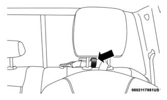
**Tether Strap Through Outboard Tether Strap Loop**
