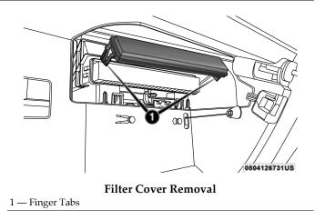
5. Remove the cabin air filter by pulling it straight out of the housing.
