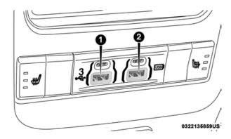
Rear Center Console Standard (Type A) USB Ports 1 — Standard USB Type A Port #1
