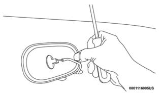
**Removing Bulb Socket From Clearance Lamp**
