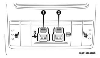
Rear Center Console Mini-USB (Type C) USB Ports 1 — Mini-USB Type C Port #1
