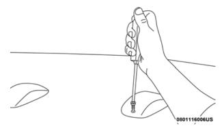
**Removing Rear Screw From Clearance Lamp**
