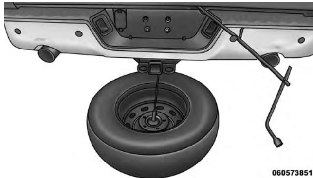
Pulling The Spare Tire Out
