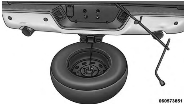
Pulling The Spare Tire Out
