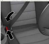
**Inserting Latch Plate Into Buckle**
