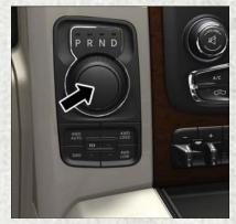
**Electronic Transmission Gear Selector**
