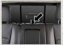
Crew Or Quad Cab Center Tether Anchorage With Head Restraint In Raised Position
