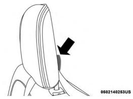
Tether Strap Through Outboard Tether Strap Loop
