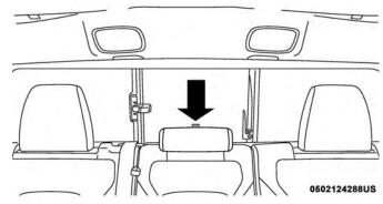
Center Tether Anchorage Over Head Rest
