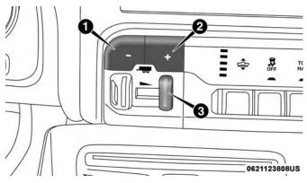
**Integrated Trailer Brake Module (ITBM)**
