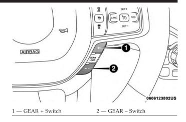
To exit ERS mode, simply push and hold the GEAR+ switch until the gear limit display disappears from the instrument cluster.
