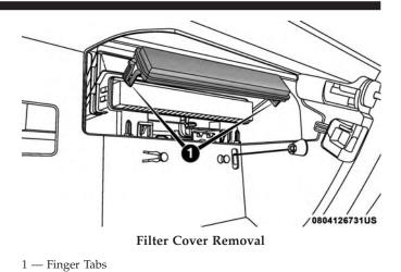
6. Remove the cabin air filter by pulling it straight out of the housing.
