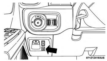
Instrument Panel Power Inverter Switch
