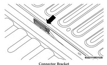
2. Remove the connector bracket from the sill by pushing inward in the locking tab.
