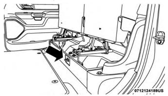
Rotate Lock Mechanism
