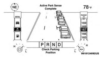
Active Park Sense Complete — Check Parking Position Perpendicular Parking Space Assistance Operation/Display
