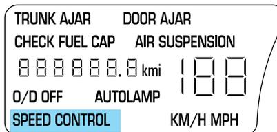
**O/D off:** Illuminates when the overdrive function of the transmission has been turned OFF using the transmission control switch (TCS), refer to the *Driving* chapter. If the light flashes steadily or does not illuminate, have the transmission serviced soon, or damage may occur.
