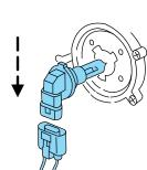
Handle a halogen headlamp bulb carefully and keep out of children's reach. Grasp the bulb only by its plastic base and do not touch the glass. The oil from your hand could cause the bulb to break the next time the headlamps are operated.
