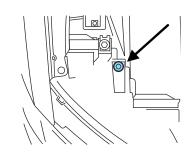
$\operatorname{HORIZONTAL}$  AIM IS NOT REQUIRED FOR THIS VEHICLE AND IS NON-ADJUSTABLE.
