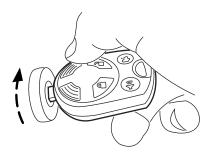
Likewise, when rotating the IKT to the 1 (LOCK) position in the ignition lock cylinder, the bottom edge of the IKT adjacent to the control can be utilized.
