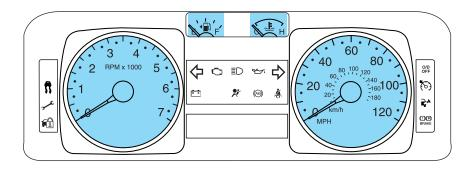
**Speedometer:** Indicates the current vehicle speed.
