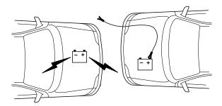
1. Connect the positive (+) jumper cable to the positive (+) terminal of the discharged battery.
