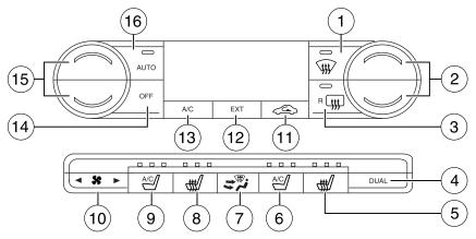
**Temperature conversion:** To switch between Fahrenheit and Celsius, refer to *Units (Fahrenheit/Celsius)* in the *Driver Controls* chapter. **MAX A/C setting:** In order to achieve maximum cooling performance, press  $\overset{\sim}{\sim}$ , A/C,  $\overset{\sim}{\sim}$ , and set the temperature to 60° F (16° C) and the highest blower setting.
