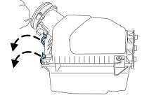
5. Install a new air filter element. Be careful not to crimp the filter element edges between the air filter housing and cover. This could cause filter damage and allow unfiltered air to enter the engine if not properly seated. 252
