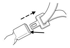
All restraints in the vehicle are combination lap and shoulder belts. While you are fastened in the safety belt, the combination lap/shoulder belt adjusts to your movement. However, if you brake hard, turn hard, or if your vehicle receives an impact of 5 mph (8 km/h) or more, the safety belt will become locked and help reduce your forward movement.
