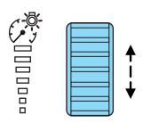
and visibility. The system automatically "dims down" as ambient light reaches the dash-mounted sensor. The interior control lights dim progressively in four steps until they reach nighttime operating levels. Certain displays like the message center and the climate control unit do not change with the dimmer control till the dash-mounted sensor senses full night conditions.
