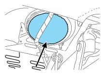
• The filter can be accessed from the first row seat. Move the front seats all the way back and up to ease access.
