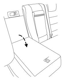
Before returning the seatback to its original position, make sure that cargo or any objects are not trapped behind the seatback. After returning the seatback to its original position, pull on the seatback to ensure that it has fully latched. An unlatched seat may become dangerous in the event of a sudden stop or collision.
