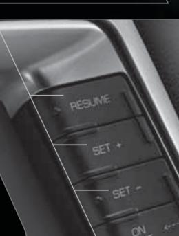
**TO SET THE SPEED:** Press **ON**. Accelerate to the desired speed. Press **SET +** or **SET -** and take your foot off the accelerator.
