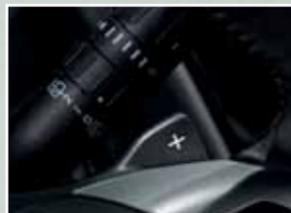
**SELECTSHIFT AUTOMATIC™ TRANSMISSION:** Gives you the ability to manually change gears if you'd like. To use, move the gearshift lever from D (Drive) to S (Sport). Now you can manually change gears with SelectShift by using the paddles located on your steering wheel. Pull the right paddle (+) to upshift, pull the left paddle (-) to downshift.
