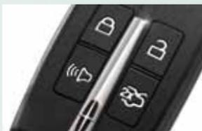
To unlock and open the driver's door, pull the front exterior door handle. To lock the doors, touch the sensor button on the door handle. To unlock the trunk, press the exterior trunk release button near the license plate. The intelligent access key also contains a mechanical key blade, which can be used to unlock the driver door if necessary.
