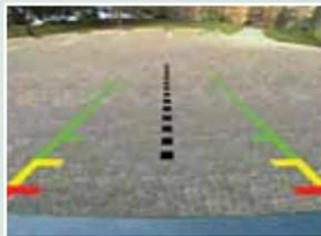
**REARVIEW CAMERA\*:** This system provides a visual display of the area behind the vehicle. The display automatically appears in the touchscreen when the vehicle is in R (Reverse) and uses green, yellow and red guides to alert you of your proximity to objects.
