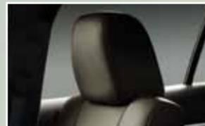
**TILTING HEAD RESTRAINTS\*:** Your vehicle's front row head restraints can be adjusted. Pull up to raise the head restraint. To lower, press the head restraint down while pressing and holding the guide sleeve adjust/release button. Tilt the head restraint forward for additional comfort by gently pulling the top of the head restraint. Once it is in the forward-most position, tilting it forward once more will release it to the upright position.
