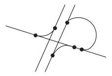
On the map CD, the road network is stored as a line pattern, which means that even extensive junctions only have one center point all roads lead to. That is why the navigation system indicates the distance to the next turn as the distance to the center of the junction. Therefore, the distance indications for freeway exits given by the navigation system may be different from those on the freeway signs. The freeway signs refer to the distance to the beginning of the exit.
