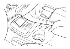
Turn the rotary button clockwise or counterclockwise to move the cursor on the screen. In this user manual, it will be referred to as SELECT.
