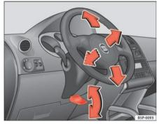
Fig. 128 Adjusting the steering wheel position
