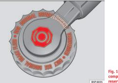
Fig. 161 In the engine compartment: Brake fluid reservoir cover
