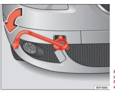
Fig. 195 The front right section of the vehicle: Fitting the front towing eye
