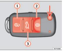
Fig. 66 Battery pilot lamp in remote control key
