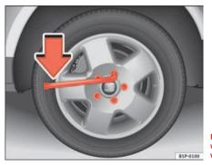
Fig. 166 Changing the wheel: Loosening the wheel bolts
