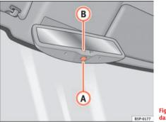
Fig. 90 Automatic antidazzle interior mirror.
