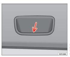
Fig. 69 Detail of the tailgate inner trim: recessed handle for closing the tailgate
