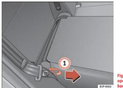
Fig. 100 Folding or opening the front seat backrests
