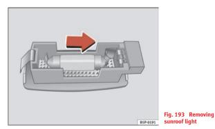
Remove the lamp, moving it in the direction of the arrow and outwards. ⇒ fig. 193 ■
