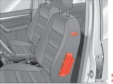
Fig. 22 Side airbag in driver seat
