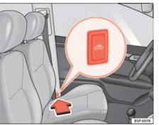
Fig. 67 Button for deactivating the interior monitoring system
