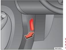
Fig. 151 Detail of the footwell: The release lever for the bonnet is located in the driver side footwell
