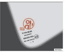
Fig. 6 Head restraint position warning label
