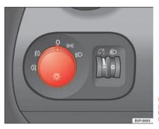
Fig. 75 Detail of the dash panel: Switch for lights, fog lights and rear fog light
