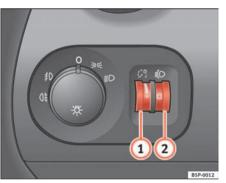
Fig. 77 Detail of the dash panel: Regulation for instrument and switch illumination and headlight range control
