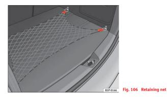
Use the fastening rings located on the side of the luggage compartment to attach the retaining net⇒ fig. 106
