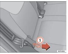
Fig. 98 Rear seat backrest angle adjustment The seats may be moved forwards independently. The movement can be 1/3 or 2/3 of the seat. There are various possible positions.
