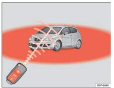
Fig. 65 Range of the remote control
