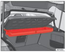
Fig. 118 Warning triangle storage under the rear cover
