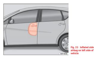
In some **side collisions** the side airbag is triggered on the impact side of the vehicle  $\Rightarrow$  fig. 23.
