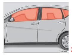
Fig. 25 Deployed curtain airbags
