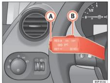
Fig. 143 Turn signal and main beam lever: switch and rocker switch for CCS
