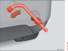
Fig. 196 Fitting the towing eye to the rear of the vehicle
