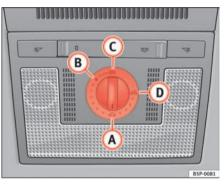
Fig. 72 Detail of the sunroof: rotary button for sliding/tilting sunroof
