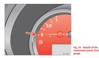
Details of the instrument panel: Fuel gauge
