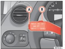
Fig. 141 Turn signal and main beam lever: switch and rocker switch for CCS
