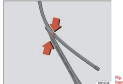
Fig. 159 Changing the front wiper blades To change the blades it is necessary to change the rest position of the wipers to the service position.
