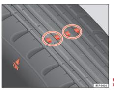
Fig. 162 Tyre tread wear indicators
