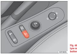
Fig. 48 Centre console: tyre monitor system button The tyre monitor indicator compares wheel revolutions and with this information, the diameter of each wheel using the ABS sensors. If the diameter of a wheel changes, the tyre monitor indicator lights (1). The wheel diameter changes when:
