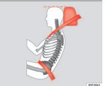
Fig. 93 Viewed from side: Properly adjusted head restraints and proper belt adjustment
