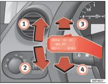
Fig. 79 Turn signal and main beam headlight lever
