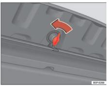
Fig. 119 Opening the storage compartment
