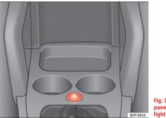
Fig. 78 Detail of the dash panel: Hazard warning light switch
