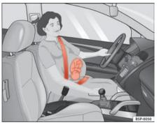
Fig. 15 Positioning seat belts during pregnancy
