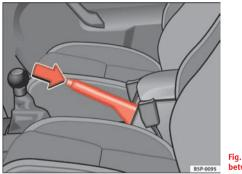
Fig. 139 Handbrake between the front seats
