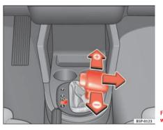
Fig. 138 Changing gear with Tiptronic
