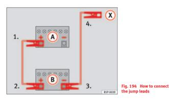
In  $\Rightarrow$  fig. 194, the flat battery is **A** and the charged battery **B**.
