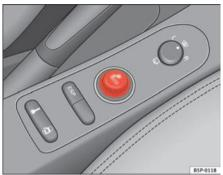
Fig. 115 The cigarette lighter is located in the electric socket on the front of the centre console
