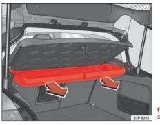
Fig. 121 Removing storage shelf
