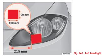
On the right headlight, if you are changing from driving on the right-hand side to the left-hand side.  $\Rightarrow$  fig. 144 On the left headlight, if you are changing from driving on the right-hand side to the left-hand side.  $\Rightarrow$  fig. 145  $\blacksquare$
