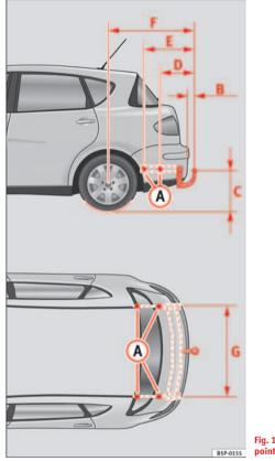
Fig. 149 Attachment points for towing bracket
