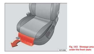
The drawer\*  $\Rightarrow$  fig. 103 (A) is opened by pushing the button and putting the cover back.
