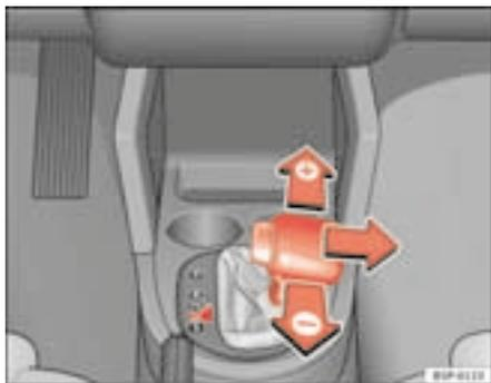
Fig. 137 Trocar com tiptronic
