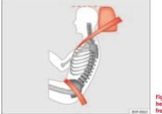
Fig. 4 Properly adjusted head restraint viewed from the side Adjust the head restraint properly to achieve maximum protection.
