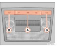
Fig. 79 Interior roof lining: front passenger compartment lighting
