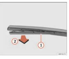
Fig. 164 Changing the rear window wiper blade
