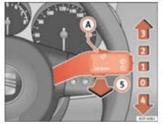
Fig. 84 Windscreen wiper and windscreen wash lever The windscreen wiper lever  $\Rightarrow$  fig. 84 has the following positions:
