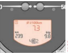
Fig. 40 Digital display in the instrument panel: average fuel consumption indicator
