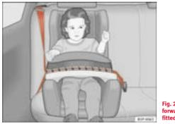
Fig. 29 A category 1 forward-facing child seat fitted on the rear seat.
