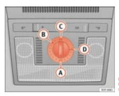
Fig. 71 Roof interior lining: closing the sliding/tilting sunroof
