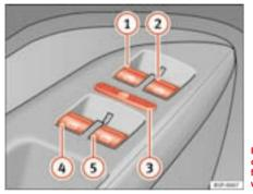
Fig. 69 Buttons on the driver's door: controls for front and rear electric windows
