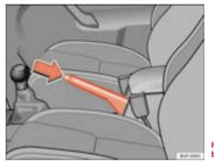
Fig. 138 Handbrake between the front seats
