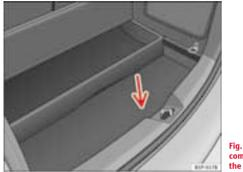
Fig. 168 Luggage compartment. Access to the spare wheel
