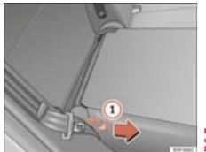
Fig. 98 Folding or opening the front seat backrests
