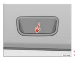
Fig. 67 The inner tailgate lining: hand hold
