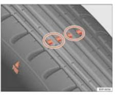
Fig. 166 Tyre tread wear indicators
