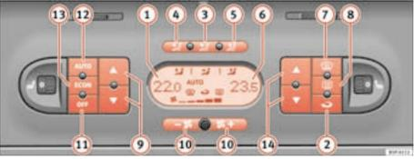
Fig. 125 On the dash panel: 2C Climatronic controls
