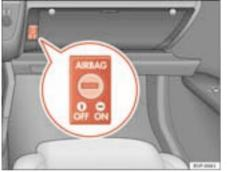
Fig. 26 In the glove compartment: there is key switch for disabling and enabling the airbags on the front passenger side
