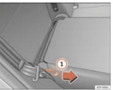
Fig. 97 Folding or opening the rear seat backrests
