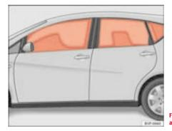
Fig. 25 Deployed curtain airbags
