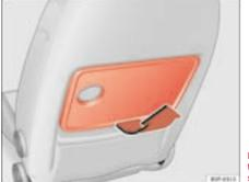
Fig. 102 Folding tray for the front left hand side seat
