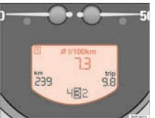
Fig. 42 Digital display in the instrument panel: average fuel consumption indicator.
