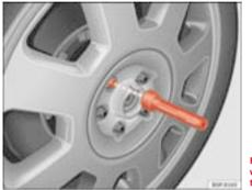
Fig. 173 Changing the wheel: Hexagonal socket tool for the bolts
