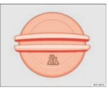
Fig. 160 In the engine compartment: Coolant expansion tank cap
