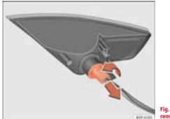
Fig. 190 Rear light after removal from bumper
