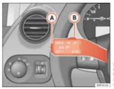
Fig. 141 Turn signal and main beam headlight lever: switch and rocker switch for the cruise control
