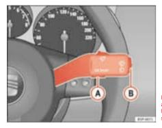
Fig. 39 Windscreen wiper and windscreen wash lever: switch A and rocker switch B
