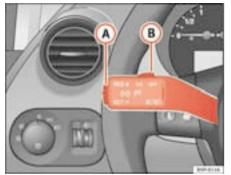
Fig. 139 Turn signal and main beam headlight lever: switch and rocker switch for the cruise control
