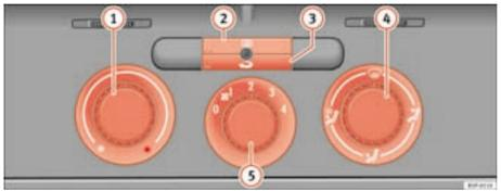
Fig. 121 On the dash panel: Heater controls
