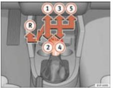
Fig. 131 Centre console: diagram for 5 speed manual gearbox
