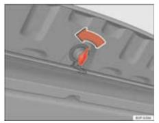
Fig. 118 Opening the storage compartment The warning triangle is located in a stowage box under the luggage compartment cover  $\Rightarrow$  fig. 118.To open this storage compartment, turn the knob 90° fig.
