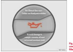
Fig. 159 In the engine compartment: Engine oil filler cap
