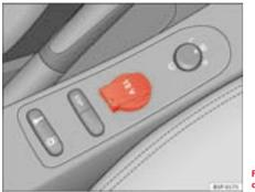
Fig. 115 Socket, centre console, front
