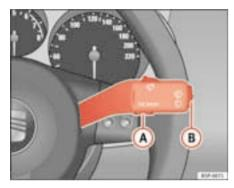
Fig. 45 Windscreen washer lever: button A to confirm the menu option and rocker switch B to change the menu
