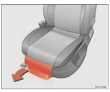
Fig. 101 Stowage area under the front seats
