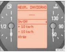
Fig. 46 Digital display in the instrument panel: winter tyres indicator
