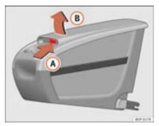
Fig. 111 Mobile stowage compartment Opening
