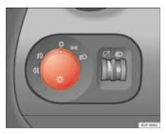
Fig. 73 Description of the instrument panel: lights control, antifog lights and rear antifog light
