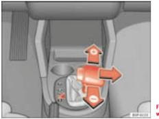
Fig. 137 Changing gear with Tiptronic
