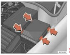
Fig. 176 Fuse box cover in engine compartment
