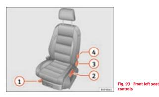
The control elements in  $\Rightarrow$  fig. 93 are mirrored for the front righthand seat.
