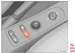
Fig. 48 Centre console: tyre monitor system button
