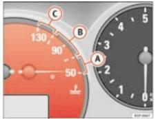
Fig. 35 Instrument panel: engine coolant temperature
