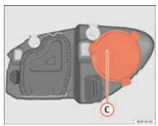
Fig. 181 Main beam headlights
