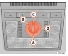
Fig. 70 Roof interior lining: closing the sliding/tilting sunroof
