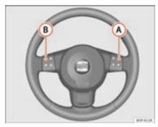
Fig. 57 Steering wheel Audio + Telephone version controls
