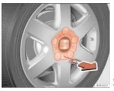
Fig. 169 Changing the wheel: Pull off the hub cap
