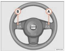
Fig. 58 Steering wheel audio version controls
