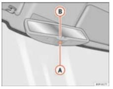
Fig. 88 Automatic antidazzle interior mirror.
