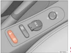
Fig. 60 Centre console: central locking button
