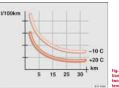
Fig. 152 Fuel consumption in litres per 100 km at two different ambient temperatures
