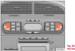
Fig. 94 Thumb wheel for the front seat heating
