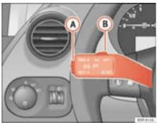
Fig. 140 Turn signal and main beam headlight lever: switch and rocker switch for the cruise control
