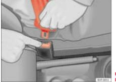
Fig. 16 Removing latch plate from buckle
