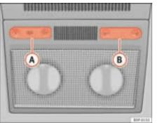
Fig. 78 Interior roof lining: front passenger compartment lighting
