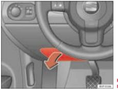
Fig. 175 Left side of dash panel: Fuse box cover
