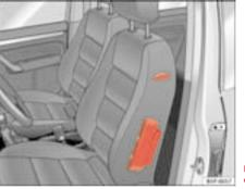
Fig. 22 Side airbag in driver seat
