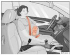
Fig. 15 Positioning seat belts during pregnancy
