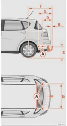
Fig. 153 Attachment points for towing bracket
