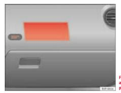
Fig. 19 Front passenger airbag located in dash panel The front airbag for the driver is located in the steering wheel  $\Rightarrow$  fig. 18 and the airbag for the front passenger is located in the dash panel  $\Rightarrow$  fig. 19. Airbags are identified by the text "AIRBAG".
