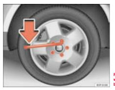
Fig. 170 Changing the wheel: loosening wheel bolts
