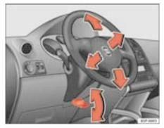
Fig. 127 Adjusting the steering wheel position
