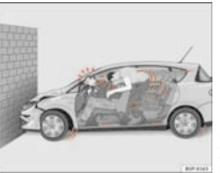
Fig. 8 The vehicle collides with the wall: the occupants are not wearing seatbelts
