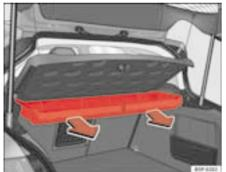
Fig. 120 Removing storage shelf
