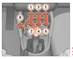
Fig. 132 Centre console: diagram for 6 speed manual gearbox
