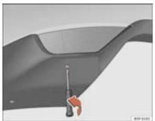
Fig. 189 Rear light fitted on bumper and viewed from below
