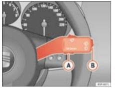
Fig. 43 Windscreen washer lever: button A to confirm the menu option and rocker switch B to change the menu
