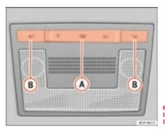
Fig. 81 Interior roof lining: front reading lights, type 2
