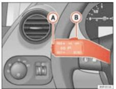
Fig. 143 Turn signal and main beam headlight lever: switch and rocker switch for the cruise control
