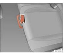
Fig. 95 For unlocking the rear seat
