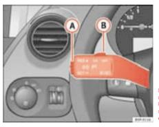
Fig. 142 Turn signal and main beam headlight lever: switch and rocker switch for the cruise control
