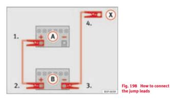
In  $\Rightarrow$  fig. 198, the flat battery is (A) and the charged battery (B).
