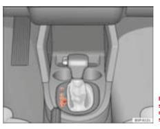
Fig. 133 Centre console: selector lever for automatic gearbox / direct shift gearbox (DSG)
