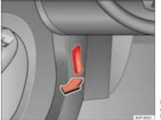
Fig. 155 Details of the driver-side foot well: bonnet release lever
