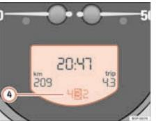
Fig. 37 Description of the instrument panel: screen with Tiptronic gear indicator
