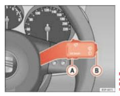
Fig. 41 Windscreen wiper and windscreen wash lever: switch A and rocker switch B
