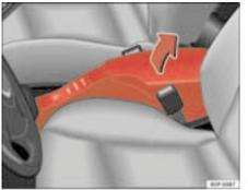
Fig. 100 Front armrest with stowage area
