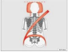
Fig. 90 Front view: headrest and seatbelt correctly adjusted
