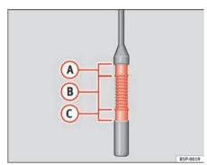
Fig. 163 Engine oil dipstick.
