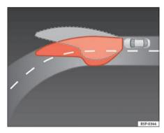
Fig. 76 Cornering lighting using directional headlights
