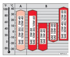
Fig. 162 Types of oil according to temperature
