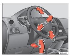
Fig. 132 Adjusting the steering wheel position
