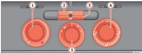
Fig. 126 On the dash panel: Heater controls
