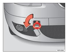
Fig. 204 The front right section of the vehicle: Fitting the front towing eve
