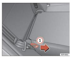
Fig. 98 Folding or opening the rear seat
