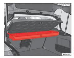
Fig. 122 Warning triangle storage under the rear cover
