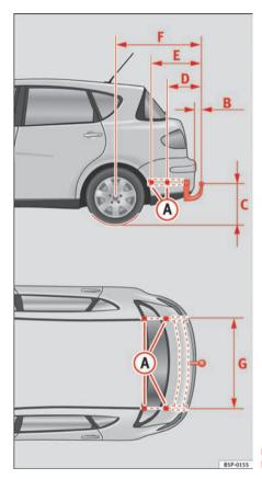
Fig. 158 Attachment points for towing bracket
