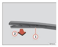
Fig. 169 Changing the rear window wiper blade
