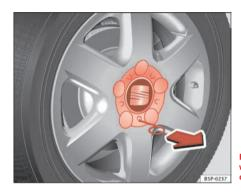
Fig. 174 Changing the wheel: Removing a hub
