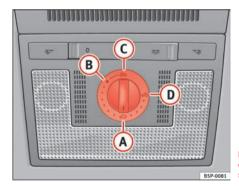
Fig. 70 Roof lining description: rotary sunroof control
