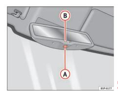
Fig. 89 Automatic antidazzle interior mirror.
