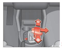
Fig. 142 Changing gear with Tiptronic
