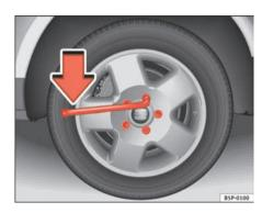
Fig. 175 Changing the wheel: loosen the wheel
