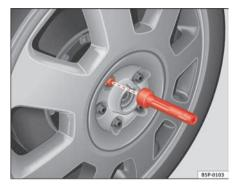
Fig. 178 Changing the wheel: Hexagonal socket in screwdriver handle to turn the wheel bolts
