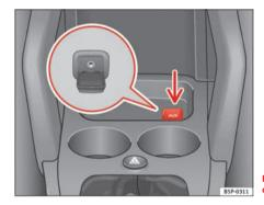
Fig. 118 Auxiliary audio connection
