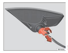
Fig. 195 Rear light after removal from bumper
