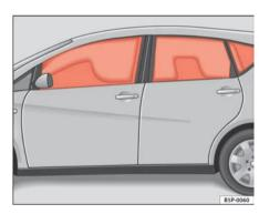
Fig. 25 Deployed curtain airbags
