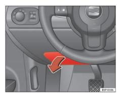
Fig. 180 Left side of dash panel: Fuse box cover
