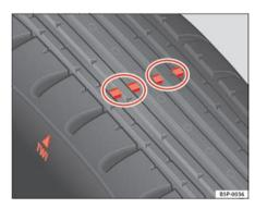
Fig. 171 Tyre tread wear indicators
