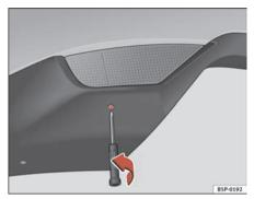
Fig. 194 Rear light fitted on bumper and viewed from below
