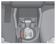
Fig. 138 Centre console: selector lever for automatic gearbox / direct shift gearbox DSG
