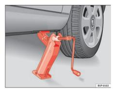
Fig. 177 Fitting the jack
