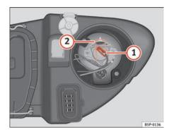
Fig. 187 Main beam headlights
