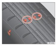
Fig. 124 Side view of tyres with tread wear indicators
