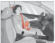
Fig. 14 Positioning seat belts during pregnancy
