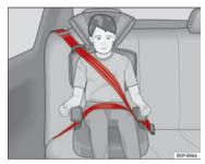
Fig. 27 Forward-facing child seat installed on rear seat
