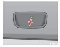
Fig. 52 Close-up of the inside trim of the rear lid: hand grip
