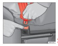
Fig. 15 Remove latch plate from buckle
