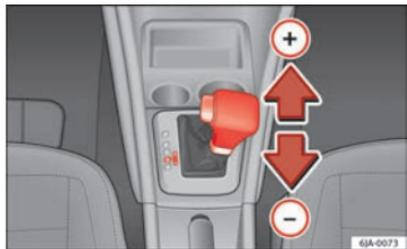
Fig. 106 Palanca selectora: Tiptronic
