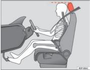
Fig. 2 Correct head restraint position for driver
