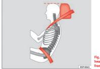
Fig. 4 Correctly adjusted head restraint viewed from the side Adjust the head restraint correctly in order to achieve maximum protection.
