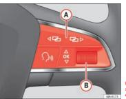
Fig. 37 Multifunction steering wheel: controls on the steering wheel
