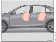
Fig. 21 Illustration of completely inflated side airbags on left side of vehicle
