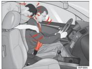
Fig. 9 The unbelted passenger in the rear seat is thrown forward violently, hitting the driver wearing a seat belt
