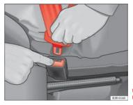
Fig. 15 Remove latch plate from buckle
