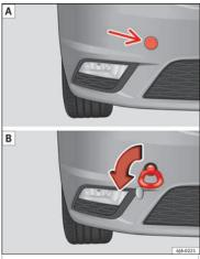
**Fig. 84** Front bumper: towline anchorage cover/fitting.
