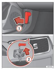
Fig. 7 Unlocking the bonnet.
