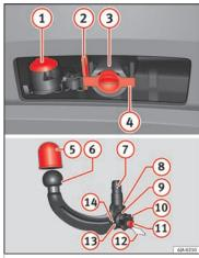
Fig. 195 Towing bracket device support for hitching/ball-headed bar.
