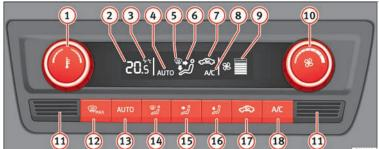
Fig. 171 Climatronic: controls.
