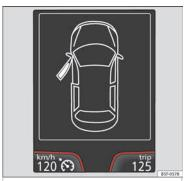
Fig. 41 On the instrument panel display: door open.
