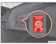
Fig. 17 Front passenger front airbag switch.
