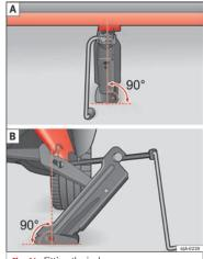
Fig. 64 Fitting the jack.
