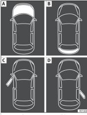
Fig. 38 A: bonnet open; B: rear lid open; C: front left door open; D: rear right door open (5-door vehicles only).
