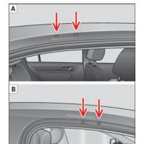
Fig. 167 Basic roof carrier attachment points.
