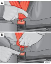
Fig. 11 Positioning and removing the seat belt buckle.
