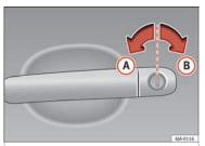
**Fig. 120** Key positions during vehicle locking and unlocking.
