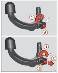
Fig. 196 Placing in service position.
