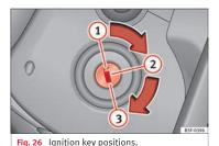
Switch ignition on: Place the key in the ignition and start the engine.
