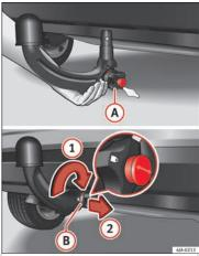
Fig. 198 Placing the ball-headed bar/locking and removing the kev.
