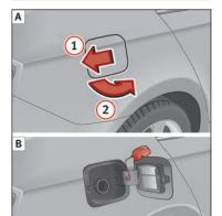
Fig. 48 Vehicle as seen from the rear right: fuel tank flap/fuel tank flap with tank unscrewed cap attached.
