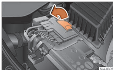
Fig. 248 Battery: opening the cover.
