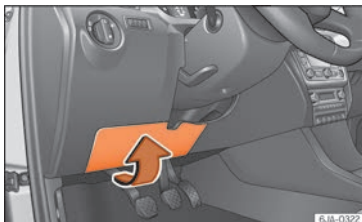
Fig. 55 On the dashboard on the driver side: lid of the fuse box.
