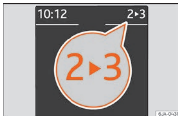
Fig. 219 Instrument panel: gear-change indicator (manual gearbox).
