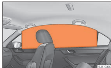
Fig. 24 Deployed head-protection airbags.
