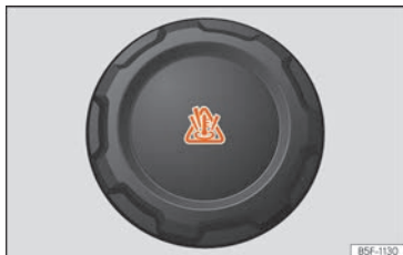
Fig. 52 Engine compartment: coolant expansion tank cap.
