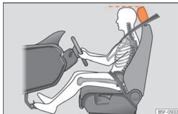
Fig. 73 Correct head restraint position for the driver.
