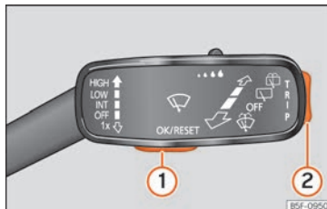
Fig. 38 Windscreen wipers lever: control buttons.
