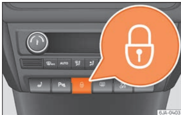
Fig. 4 Centre console: central locking switch.
