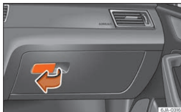
Fig. 147 Instrument panel: passenger side glove compartment.
