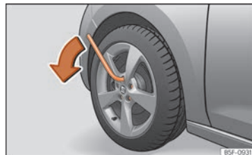
Fig. 63 Tyre change: slacken the wheel bolts. »
