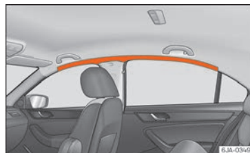
Fig. 23 Location of head-protection airbags.
