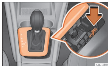
Fig. 45 Manual release of the selector lever.
