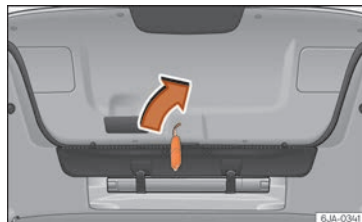
Fig. 8 Luggage compartment: access to manual release.
