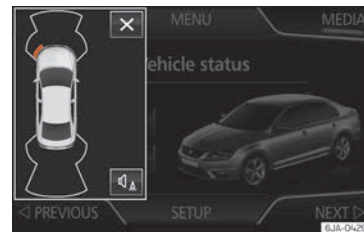
Fig. 228 Miniature indication of automatic activation.
