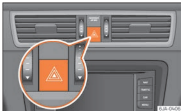
Fig. 32 Dashboard: switch for hazard warning lights.
