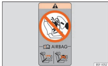
Fig. 26 On the rear frame of the passenger side door: adhesive in relation to the airbag.
