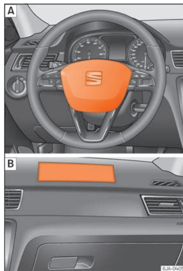
Fig. 18 Driver airbag in the steering wheel and front passenger airbag in the dash panel
