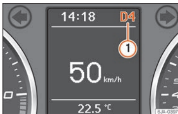
Fig. 217 Information display: selector lever positions.
