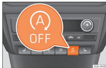
Fig. 221 Instrument panel: Start-stop button.
