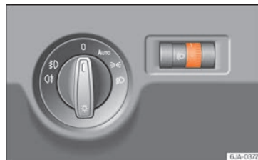
Fig. 130 Instrument panel: light range control.
