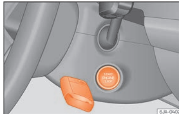
Fig. 213 Emergency ignition in vehicles with Keyless Access.
