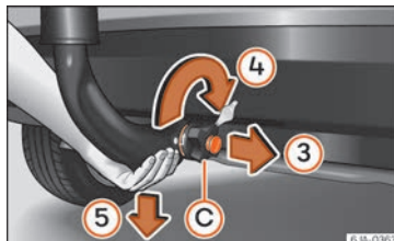
Fig. 240 Unblock the ball-headed bar.
