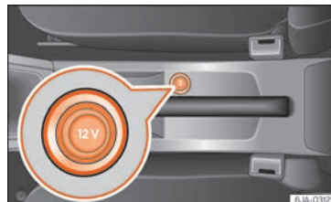
Fig. 154 Centre console: 12 V power socket.
