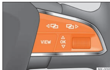
Fig. 39 Right side of the multifunction steering wheel: control buttons.
