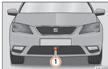
Fig. 224 On the front bumper: radar sensor.
