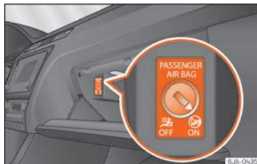
Fig. 20 Front passenger front airbag switch.
