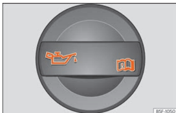
Fig. 51 In the engine compartment: Engine oil filler cap.
