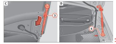
Fig. 105 C: Bonnet securing rod in the bonnet. D: Bonnet supported by the bonnet securing rod.
