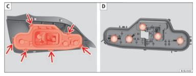
Fig. 149 Tail light unit: C: Remove the bulb holder, D: Remove the bulbs.
