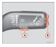
Fig. 11 Windscreen wiper lever: button (A) to confirm the options and rocker switch (B) to change the options.
