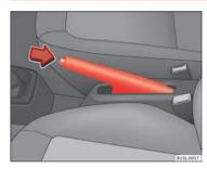
Fig. 86 Between the front seats: Handbrake.
