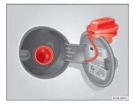
Fig. 103 Open fuel tank flap with tank plug attached to the holder.
