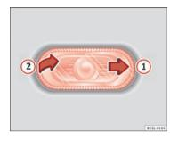
Fig. 152 Removing the side turn signal.
