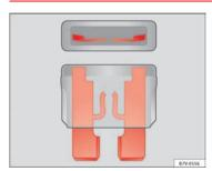
Fig. 144 Image of a blown fuse.
