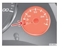
Fig. 101 On the instrument panel: fuel gauge for petrol.
