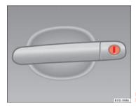
Fig. 127 Driver side door handle with lock cylinder.
