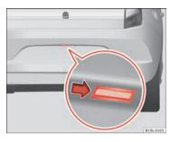
Fig. 150 On the rear bumper: Remove number plate light.
