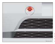
Fig. 156 On the righthand side of the front bumper: Remove the cover.
