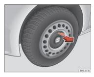
Fig. 133 Remove the hubcap of the steel wheel trim.
