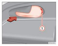
Fig. 20 In the passenger door: Door handle for mechanical locking.
