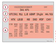
Fig. 158 TO: Vehicle data label: in the example, engine with code CBFA
