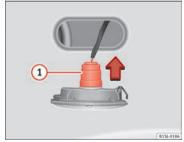
Fig. 153 Side turn signal: Changing the bulbs.
