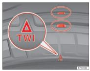
Fig. 117 Tyre tread: tread wear indicators.
