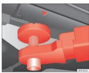
Fig. 123 Rear jacking points for raising vehicle with lifting platform or jack.
