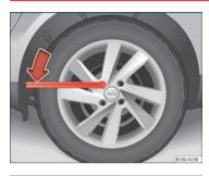
Fig. 136 Changing the wheel: Slacken the wheel bolts.
