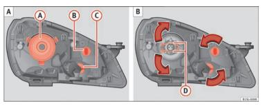
Fig. 145 In the engine compartment: Rear view of the front left headlight with rubber cover: (a) dipped beam and main beam headlights, (b) side lights and daytime driving lights and (c) turn signal.
