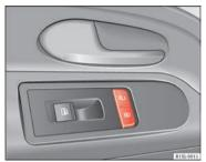
Fig. 19 In the driver door: central locking button.
