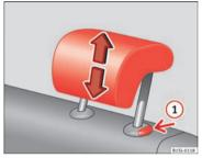
Fig. 32 Removing the rear head restraint.
