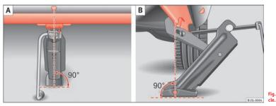
Fig. 139 jack mounted on the left rear part of the vehicle.
