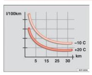
Fig. 88 Fuel consumption in litres per 100 km at 2 different outside temperatures.
