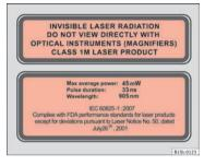
Fig. 124 Warnings relating to handling of the City Safety Assist system laser sensor function.
