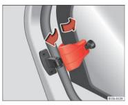
Fig. 25 Lever to open and close the rear window
