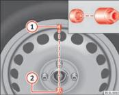
Fig. 137 Changing the wheel: Tyre valve ① and position of anti-theft wheel locking bolt ②.
