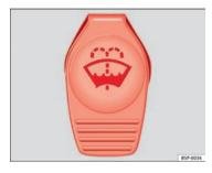
Fig. 63 In the engine compartment: wind-screen washer bottle top.
