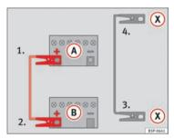
Fig. 155 Diagram for connecting jump leads if the vehicle providing assistance is fitted with the Start-Stop system: flat battery (a) and battery providing current (a).
