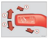
Fig. 55 Turn signal and main beam lever in their initial position.
