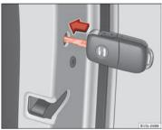
Fig. 129 Emergency locking of the vehicle using the vehicle key.
