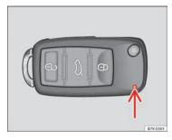
Fig. 14 Control lamp on the vehicle key.
