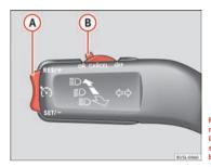
Fig. 91 Turn signal and main beam headlights lever on the left of the steering column: CCS buttons and controls.
