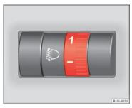
Fig. 57 Next to the steering wheel: Head-light range control.
