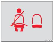
Fig. 36 Indication of seat belt status in the rear seats on the instrument panel display.
