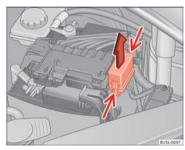
Fig. 143 In the engine compartment: fuse box cover.
