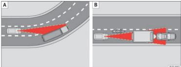
Fig. 95 A: Vehicle on a bend. B: Motorcyclist driving ahead out of range of the laser sensor.
