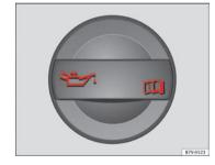
Fig. 107 In the engine compartment: Engine oil filler cap.
