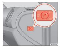
Fig. 49 On front passenger side: key switch for disabling and enabling the front passenger air-
