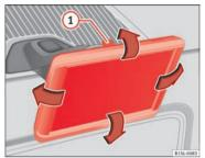
Fig. 120 In the centre console: Remove the navigator.
