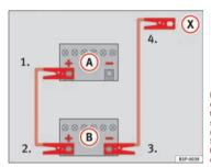
Fig. 154 Diagram for connecting jump leads if the vehicle providing assistance the current is not fitted with the Start-Stop system: flat battery (A) and battery providing current (B).
