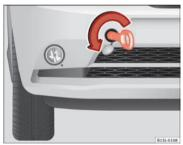
Fig. 157 On the righthand side of the front bumper: Screw in the towing ring.
