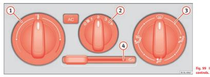
Fig. 99 In the centre console: Air conditioning system controls
