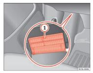
Fig. 142 Below the driver side dash panel: fuse box cover.
