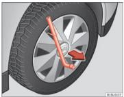
Fig. 134 Removing the full hubcap.
