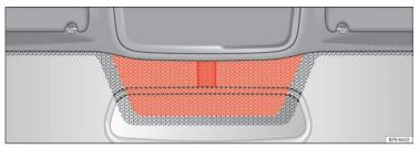
Fig. 59 Windscreen with reflective infrared and metal coating and small window (red surface).
