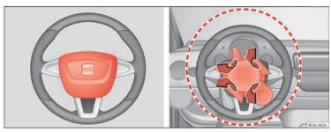
Fig. 47 Location and deployment area of the front airbag for the driver.
