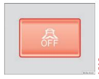
Fig. 94 In the lower part of the centre console: Button for the City Safety Assist function.
