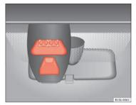
Fig. 92 On the windscreen: City Safety Assist function laser sensor.
