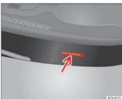
Fig. 159 Vehicle identification number.
