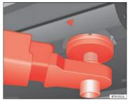
Fig. 122 Front jacking points for raising vehicle with lifting platform or jack.
