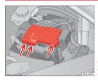
Fig. 110 In the engine compartment: Remove the cover from the vehicle's battery.
