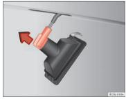
Fig. 151 Number plate light: Remove the lamp holder.
