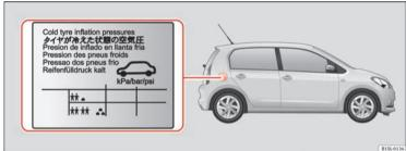
8151-0134 Fig. 116 Position of tyre pressure specification plate.
