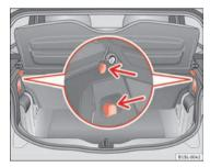
Fig. 69 In the luggage compartment: retaining hooks.
