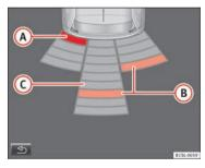
Fig. 90 On-screen OPS display: (A) an obstacle has been detected in the collision zone. (B) an obstacle has been detected in the segment. (C) zone recorded behind the vehi-
