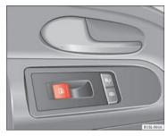
Fig. 24 In the driver door: electric windows button.
