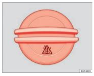
Fig. 109 In the engine compartment: Coolant expansion tank cap.
