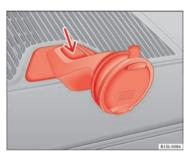
Fig. 121 Remove the navigator holder.
