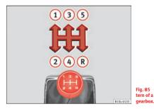
Fig. 85 Gear shift pattern of a 5-speed manual
