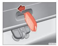
Fig. 130 From the luggage compartment: Manually unlocking the rear lid
