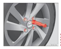
Fig. 140 Changing the wheel: loosen wheel bolts with the socket at the end of the wheel brace.
