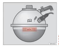
Fig. 108 In the engine compartment: Marking on coolant expansion tank.
