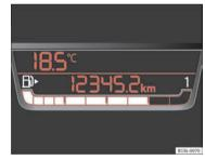
Fig. 102 Instrument panel display: fuel gauge for petrol.
