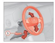
Fig. 33 Mechanical steering wheel adjust-
