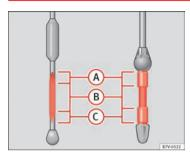
Fig. 106 Marked engine oil dipstick.
