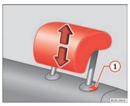
Fig. 31 Adjusting the rear head restraints.
