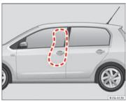
Fig. 51 On the left side of the vehicle: deployment area of side airbag.
