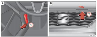
Fig. 104 A: Release lever in the footwell on the driver side. B: Release lever on the bonnet.
