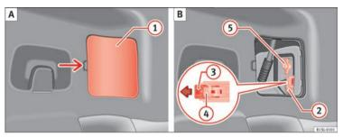
Fig. 148 On the side of the luggage compartment: TO: Remove the cover, B: Removing the tail light units.
