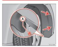
Fig. 146 In the front right wheel arch: Remove the retaining screws (arrows) and take out the expansive rivet (A).
