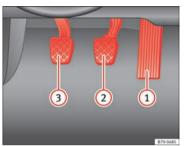
Fig. 84 Pedals: (1) accelerator: (2) brake: (3) clutch.
