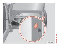
Fig. 128 In the front of the passenger side door: Emergency lock, hidden by a rubber cap.
