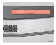
Fig. 126 In the luggage compartment: storage compartment for the warning triangle.
