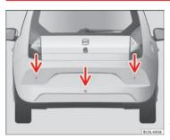
Fig. 89 Parking distance warning system sensors on the rear bumper.
