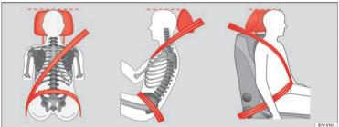
Fig. 44 Correct seat belt position.
