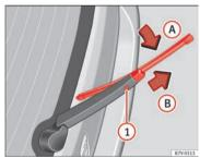
Fig. 112 Changing the rear wiper blade.
