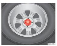
Fig. 118 In the luggage compartment: hand controlled wheel for securing the spare wheel.
