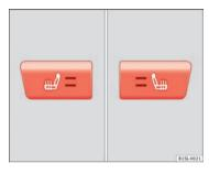
Fig. 34 In the centre console: Front seats heating switch.
