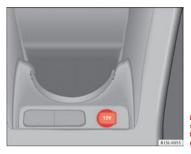
Fig. 82 Front centre console: 12 Volt socket in the storage compartment.
