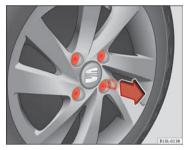
Fig. 135 Removing the wheel bolt caps.
