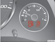
Fig. 108 On the instrument panel: fuel gauge for petrol
