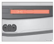
Fig. 133 In the luggage compartment: storage compartment for the warning triangle
