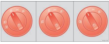
Fig. 56 Next to the steering wheel: diagram of some of the types of light switch
