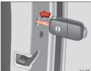
Fig. 136 Emergency locking of the vehicle using the vehicle key
