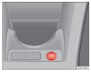
Fig. 84 Front centre console: 12 Volt socket in the storage compartment
