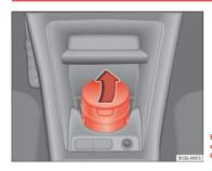
Fig. 82 In the front part of the centre console: Opening the ashtray
