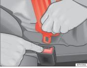
Fig. 43 Release the latch plate from the buckle
