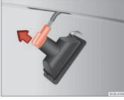
Fig. 158 Number plate light: Remove the lamp
