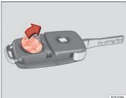
Fig. 16 Vehicle key: removing the battery
