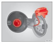
Fig. 109 Open tank flap with tank cap attached to the holder
