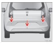
Fig. 95 Parking distance warning system sensors on the rear bumper
