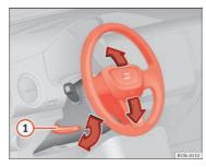
Fig. 33 Mechanical steering wheel adjustment
