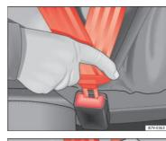
Fig. 42 Insert the latch plate into the buckle
