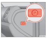
Fig. 49 On front passenger side: key switch for disabling and enabling the front passenger front airbag
