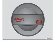
Fig. 114 In the engine compartment: Engine oil filler cap
