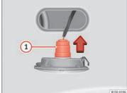
Fig. 160 Side turn signal: Changing the bulbs
