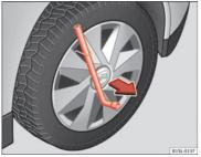
Fig. 141 Removing the full hubcap
