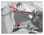
Fig. 41 Drivers with properly worn seat belts will not be thrown forward in the event of sudden braking
