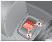
Fig. 67 Rear seat: unlock button (A); red marking (B)
