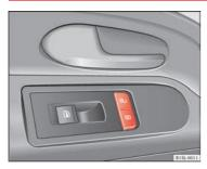
Fig. 19 In the driver door: central locking button
