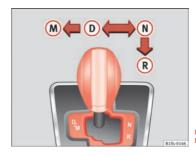
Fig. 90 Automatic gearbox diagram of gears
