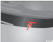
Fig. 166 Vehicle identification number
