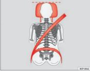
Fig. 29 Correct belt web and head restraint positions
