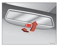
Fig. 64 Manual anti-dazzle function for rear vision mirror
