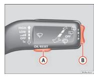
Fig. 11 Windscreen wiper lever: button (A) to confirm the options and rocker switch (B) to change the options
