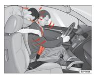
Fig. 40 The unbelted rear passenger is thrown forward violently, hitting the driver wearing a seat
