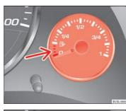
Fig. 107 On the instrument panel: fuel gauge for petrol
