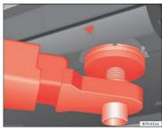
Fig. 129 Front jacking points for raising vehicle with lifting platform or jack
