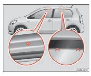
Fig. 72 Attachment points for the basic support and the roof carrier system
