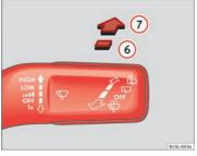
Fig. 61 Using the rear window wipers
