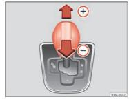
Fig. 91 Lever in the Tiptronic position
