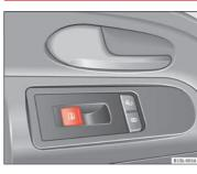
Fig. 24 In the driver door: electric windows button
