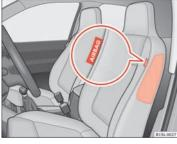
Fig. 50 On the side of the front seat: location of the side airbag
