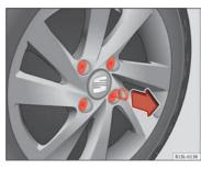
Fig. 142 Removing the wheel bolt caps
