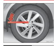
Fig. 143 Changing a wheel: Slacken the wheel bolts.
