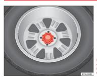
Fig. 125 In the luggage compartment: hand controlled wheel for securing the spare wheel
