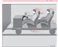
Fig. 37 Vehicle about to hit a wall: the vehicle occupants are not wearing seat belts
