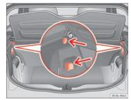
Fig. 71 In the luggage compartment: retaining hooks
