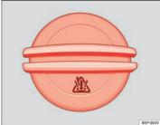
Fig. 116 In the engine compartment: Coolant expansion tank cap
