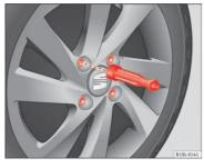
Fig. 147 Changing a wheel: loosen wheel bolts with the socket at the end of the wheel brace
