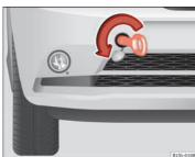
Fig. 164 On the righthand side of the front bumper: Screw in the towline anchorage
