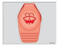
Fig. 63 In the engine compartment: wind-screen washer reservoir
