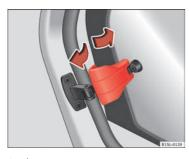
Fig. 25 Lever to open and close the rear window
