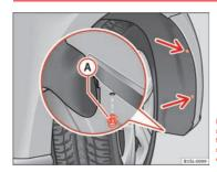
Fig. 153 In the front right wheel arch: Remove the retaining screws (arrows) and take out the expansive rivet (A).
