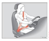
Fig. 45 Correct positioning of seat belts during pregnancy
