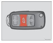
Fig. 22 On the vehicle kev: Button to unlock and open the rear lid
