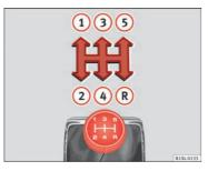
Fig. 88 Gear shift pattern of a 5-speed manual gearbox
