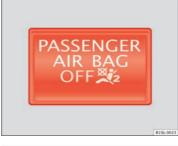
Fig. 46 Control lamp for disabling the front passenger front airbag on the dash panel
