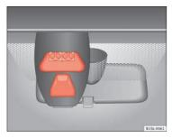
Fig. 98 In the windscreen: City Safety Assist function laser sensor
