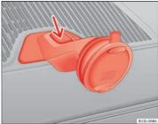
Fig. 128 Remove the navigator holder
