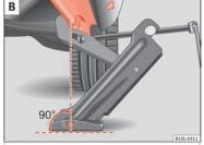
Fig. 130 Jack mounted on the left rear part of the vehicle
