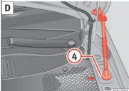
Fig. 106 C: Bonnet securing rod in the bonnet. D: Bonnet supported by the bonnet securing rod
