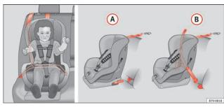
Fig. 20 On the rear seats: Possible installations for the child seat.
