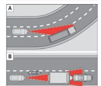
Fig. 91 A: Vehicle on a bend. B: Motorcyclist driving ahead out of range of the radar sensor.
