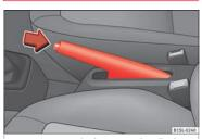
Fig. 80 Between the front seats: handbrake.
