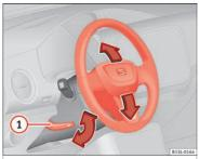
Fig. 3 Mechanical steering wheel adjustment
