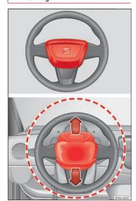
Fig. 12 Location and deployment area of the front airbag for the driver.
