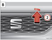
Fig. 105 A: Release lever in the footwell on the driver side B: Release lever on the bonnet
