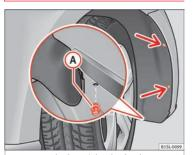
Fig. 147 In the front right wheel arch: Remove the retaining screws (arrows) and take out the expansive rivet (A).
