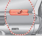
Fig. 13 Location and deployment area of the front airbag for the passenger.
