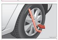
Fig. 51 Removing the full hubcap
