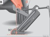
Fig. 56 Jack mounted on the left rear part of the vehicle
