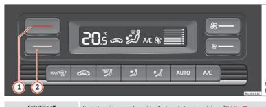
Fig. 37 At the top of the centre console: Climatronic controls
