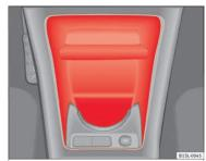
Fig. 161 In the front part of the centre console: Storage compartment with cup holder.
