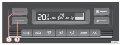
Fig. 144 At the top of the centre console: Climatronic controls
