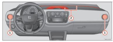
To obtain heating output, sufficient cooling and ventilation in the passenger compartment, the air vents must remain open.
