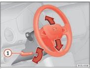
Fig. 17 Mechanical steering wheel adjustment
