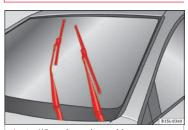
Fig. 61 Wipers in service position.
