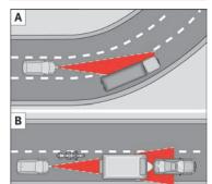
**Fig. 156** A: Vehicle on a bend. B: Motorcyclist driving ahead out of range of the laser sensor.
