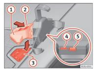
Fig. 135 In the centre console: close the compartment where the infotainment system is housed.
