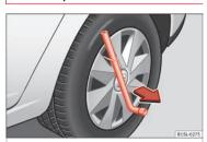
Fig. 51 Removing the full hubcap
