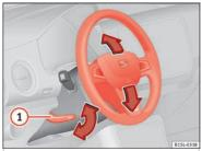
Fig. 17 Mechanical steering wheel adjustment
