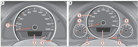
Fig. 95 Instrument panel, on dash panel: variant 1 (A) and variant 2 (B).
