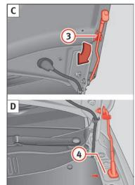
Fig. 9 C: Bonnet securing rod in the bonnet. D: Bonnet supported by the bonnet securing rod
