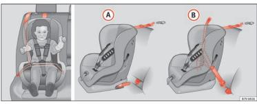
Fig. 25 On the rear seats: Possible installations for the child seat.
