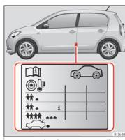
Fig. 174 Position of tyre pressure specification plate
