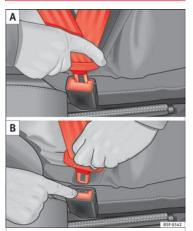
Fig. 14 Positioning and removing the seat belt buckle.
