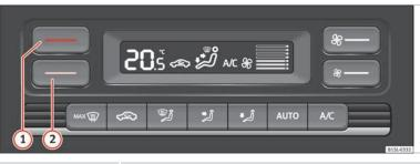
Fig. 37 At the top of the centre console: Climatronic controls
