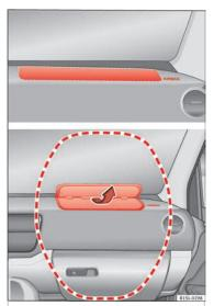
**Fig. 19** Location and deployment area of the front airbag for the passenger.
