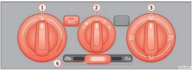
Fig. 38 At the top of the centre console: controls for the manual air conditioning and the heating and fresh air system.
