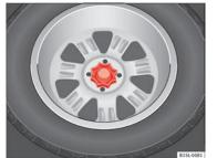
Fig. 177 In the luggage compartment: hand controlled wheel for securing the spare wheel
