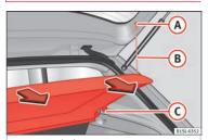
Fig. 137 In the luggage compartment: removing and installing the rear shelf
