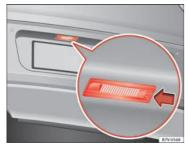
Fig. 157 In the rear bumper: number plate light
