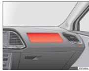
Fig. 20 Front passenger airbag located in dash panel
