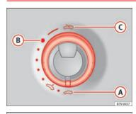
Fig. 59 On the interior roof lining: use the rotary button for opening and closing
