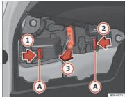
Fig. 155 Remove the bulb holder
