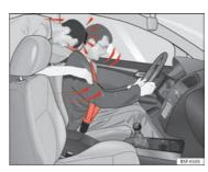
Fig. 11 The unbelted passenger in the rear seat is thrown forward violently, hitting the driver wearing a seat belt
