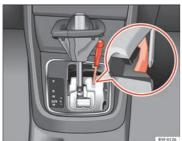
Fig. 97 Selector lever: manual release from position P
