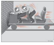
Fig. 9 The vehicle hits the wall: the occupants are not wearing seat belts
