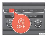
Fig. 92 Centre console: Start-Stop system button
