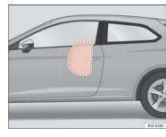
Fig. 26 Illustration of completely inflated side airbags on left side of vehicle
