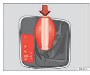
Fig. 94 Selector lever lock
