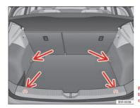
Fig. 84 Location of fastening rings in luggage compartment
