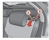
Fig. 83 Backrest release lever
