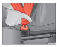
Fig. 13 Belt buckle and latch plate of seat belt
