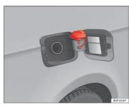
Fig. 111 Fuel tank flap with tank cap attached
