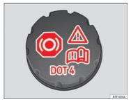
Fig. 116 Engine compartment: brake fluid reservoir, lid
