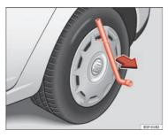
Fig. 124 Remove the complete hub cap
