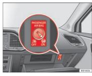
Fig. 28 Front passenger front airbag switch
