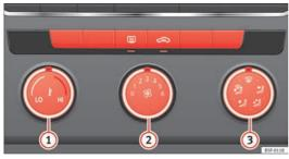
Fig. 87 In the centre console: heating system and fresh air controls
