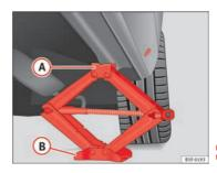
Fig. 129 Strut: mounting the jack on the vehicle
