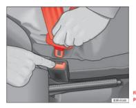
Fig. 17 Remove latch plate from buckle
