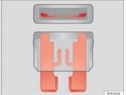
Fig. 138 Image of a blown fuse
