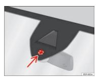
Fig. 69 Rain sensor sensitive surface
