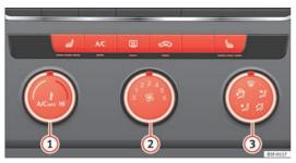
Fig. 86 In the centre console: Manual air conditioning controls
