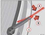
Fig. 119 Changing the rear wiper blade
