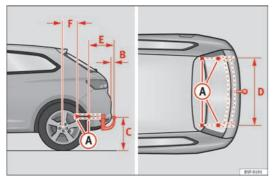
Fig. 110 Attachment points for towing bracket
