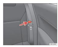
Fig. 82 Clip to support the seat belt
