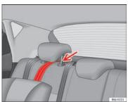
Fig. 36 Retainer strap: correct adjustment and fitting
