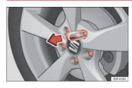
Fig. 125 Wheel: wheel bolts with caps
