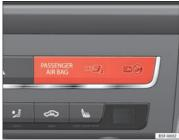
Fig. 29 Warning lamp for disabling the front passenger airbag
