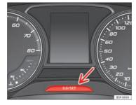
Fig. 40 Instrument panel: Odometer and reset
