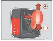
Fig. 95 Centre console: changing gear with Tiptronic
