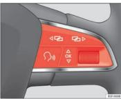
Fig. 43 Right side of multifunction steering wheel: buttons to access the instrument panel menus
