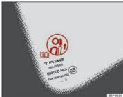
Fig. 6 Head restraint position warning label
