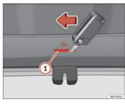
Fig. 57 Luggage compartment: access to manual release
