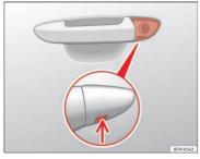
Fig. 54 Driver door lever: Hidden lock cylinder
