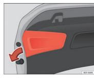
Fig. 154 Remove the cover from the rear lid
