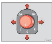
Fig. 71 Driver door: control for the exterior mirror
