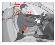
Fig. 12 A driver wearing the seat belt properly is secured by the belt in sharp braking
