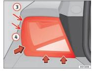
Fig. 152 Remove rear light unit from side panel
