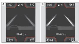
Fig. 101 On the instrument panel display: Indication on the Lane Assist system display (example 1)
