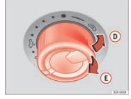
Fig. 60 On the interior roof lining: Press the button and pull on it to lift and close the sliding sunroof.
