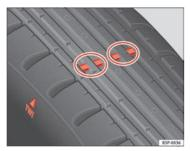
Fig. 120 Tyre tread: tread wear indicators
