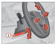
Fig. 89 Lever in the lower left side of the steering column
