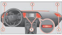
Fig. 88 On the dash panel: air vents
