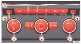
Fig. 85 In the centre console: Climatronic controls
