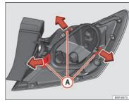
Fig. 153 Retaining tabs on reverse side of tail light
