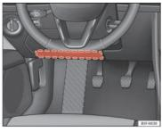
Fig. 23 On the driver side: location of the knee airbag
