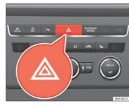
Fig. 63 Dash panel: switch for hazard warning lights
