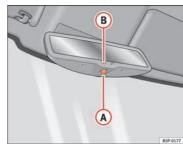
Fig. 72 Interior rear vision mirror with automatic setting for anti-dazzle position
