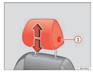
Fig. 75 Front seat: adjustment of the head restraint
