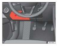
Fig. 136 On the driverside dash panel: fuse box cover
