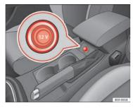
Fig. 77 Centre console: front/rear 12-volt power socket
