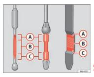
Fig. 113 Engine oil dipstick
