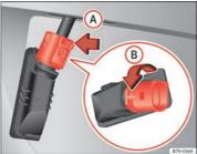
Fig. 158 Number plate light: remove the bulb holder
