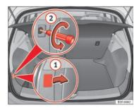
Fig. 151 Luggage compartment: Location of the bolt securing the tail light unit
