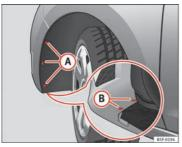
Fig. 148 Fog light: access to the connector and to the light bulb holder
