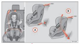
Fig. 33 On the rear seats: figure (4) shows the basic child restraint system mounting using lower retaining rings and the upper retaining strap figure (6) shows the child restraint system mounting using the vehicle seat belt
