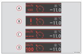
Fig. 98 Instrument panel display: CCS status indications
