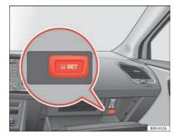
Fig. 107 Glove compartment: tyre control switch
