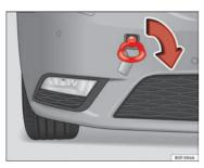
Fig. 133 Right side of the front bumper: towline anchorage screwed in
