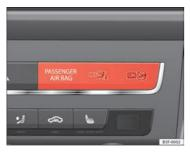
Fig. 18 Control lamp for disabling the front passenger front airbag on the dash panel
