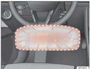
Fig. 24 On the driver side: Radius of action of the knee airbag
