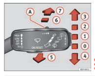
Fig. 66 Operating the windscreen wiper and rear wiper
