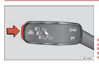
Fig. 44 On the turn signal and main beam headlight lever: button for the driving assistance systems
