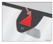
Fig. 103 In the windscreen: Field of vision of the Lane Assist system camera
