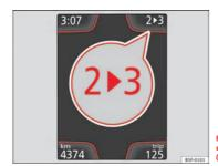
Fig. 41 Instrument panel: Gear-change indicator (manual gearbox)
