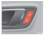
Fig. 52 Driver door: central locking switch
