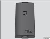
Fig. 137 In the engine compartment: fuse box cover
