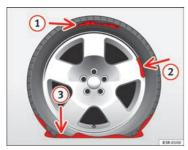
Fig. 122 Tyre: irreparable damage
