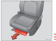
Fig. 83 Storage compartment under the front seats
