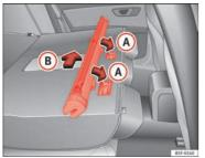
Fig. 100 Fitting the net partition in the rear seat backrests.
