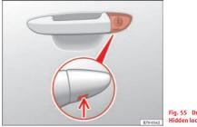
Fig. 55 Driver door lever: Hidden lock cylinder As a general rule, when the driver door is locked all other doors are locked. When the vehicle is unlocked manually, only the driver door opens. Please observe the instructions relating to the anti-theft alarm system  $\Rightarrow$  page 87.
