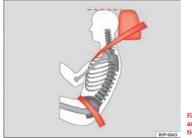
Fig. 15 Correct seat belt and head restraint positions, viewed from side
