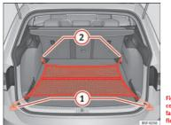
Fig. 108 In the luggage compartment: net bag fastened flush with the floor (LEON ST model).
