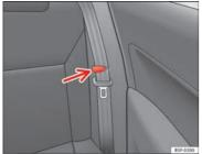
Fig. 89 Clip to support the seat belt
