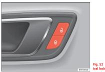
Fig. 52 Driver door: central locking switch
