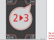
Fig. 41 Instrument panel: Gear-change indicator (manual gearbox) To familiarise yourself with the gear-change indicator, we recommend driving in the normal way to start with. A gear change will be recommended if the gear you are in is not the most economical choice.
