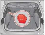
Fig. 88 Detailed view of the side trim in the luggage compartment: 12volt power sockets (valid only for the LEON ST model)
