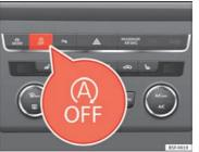
Fig. 120 Centre console: Start-Stop system button
