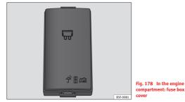
Only replace fuses with a fuse of the same amperage (same colour and markings) and size.
