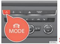
Fig. 144 Centre console: MODE button The required mode can be selected on the touch screen, in the menu that opens when the **MODE** button is pressed.
