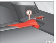
Fig. 95 In the luggage compartment: removing the rear shelf
