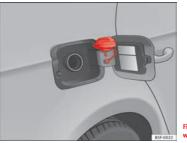
Fig. 151 Fuel tank flap with tank cap attached
