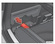
Fig. 97 In the luggage compartment: housing for storing the rear shelf.
