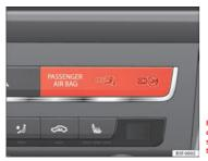
Fig. 18 Control lamp for disabling the front passenger front airbag on the dash panel
