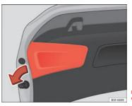
Fig. 195 Remove the cover from the rear lid
