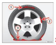
Fig. 163 Tyre: irreparable damage The tyre repair kit is designed to repair your tyre provisionally only. The damaged tyre should be replaced as soon as possible  $\Rightarrow \Lambda$ .
