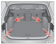
Fig. 105 In the luggage compartment: fastening rings (LEON ST model).
