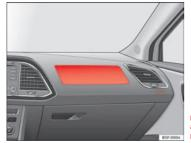
Fig. 20 Front passenger airbag located in dash panel
