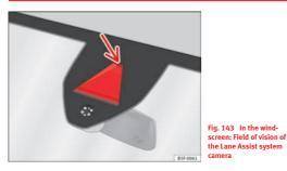
Using the camera located in the windscreen, the Lane Assist system detects the possible lines dividing the lanes. When the vehicle involuntarily approaches a dividing line it has detected, the system notifies the driver with a *corrective steering movement*. The corrective steering movement can be overruled at any moment.
