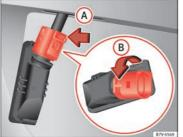
Fig. 199 Number plate light: remove the bulb holder
