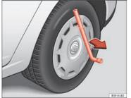
Fig. 165 Remove the complete hub cap
