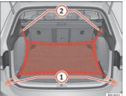
Fig. 109 In the luggage compartment: rings ① and hooks ② to fasten the net bag (LEON ST model).
