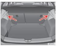
Fig. 106 In the luggage compartment: retaining hooks (LEON / LEON SC model).
