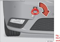
Fig. 174 Right side of the front bumper: towline anchorage screwed in
