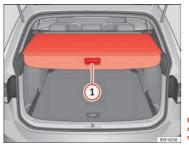
Fig. 94 In the luggage compartment: closing the rear shelf
