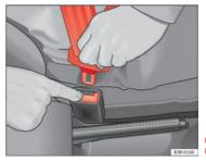
Fig. 17 Remove latch plate from buckle
