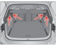
Fig. 107 In the luggage compartment: retaining hooks (LEON ST model).
