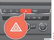
Fig. 66 Dash panel: switch for hazard warning lights
