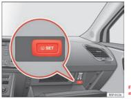
Fig. 147 Glove compartment: tyre control switch After changing the tyre pressure or replacing one or more wheels, the tyre monitoring indicator must be recalibrated. Do the same, for example, when the front and rear wheels are swapped.
