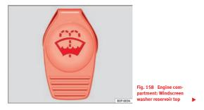
The windscreen washer reservoir  $\bigoplus$  contains the cleaning fluid for the windscreen, the rear window and the headlight washer system\*  $\Rightarrow$  Fig. 158. Reservoir capacity:  $\Rightarrow$  page 323.
