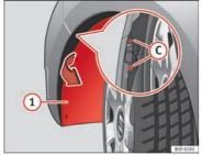
Fig. 190 Fog light: access to the connector and to the light bulb holder
