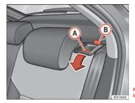
Fig. 90 Backrest release lever
