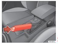
Fig. 119 Handbrake between the front seats
