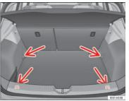
Fig. 104 In the luggage compartment: fastening rings (LEON / LEON SC model).
