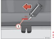
Fig. 58 Luggage compartment: access to manual release  Insert the key in the opening in the lining of the rear lid (1) and move the key in the direction of the arrow until the lock is released.
