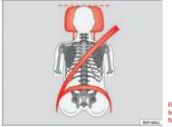
Fig. 3 Correctly adjusted head restraint viewed from the front Adjust the head restraint correctly in order to achieve maximum protection.
