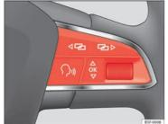
Fig. 43 Right side of multifunction steering wheel: buttons to access the instrument panel menus
