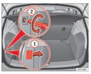
Fig. 192 Luggage compartment: Location of the bolt securing the tail light unit
