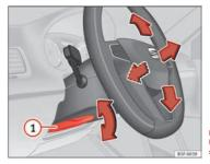
Fig. 117 Lever in the lower left side of the steering column
