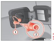
Fig. 152 Tank flap open: gas filler mouth ①, filler mouth retainer ②
