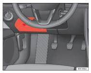
Fig. 177 On the driverside dash panel: fuse box cover
