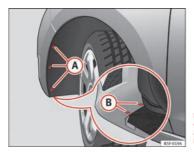
Fig. 189 Fog light: access to the connector and to the light bulb holder
